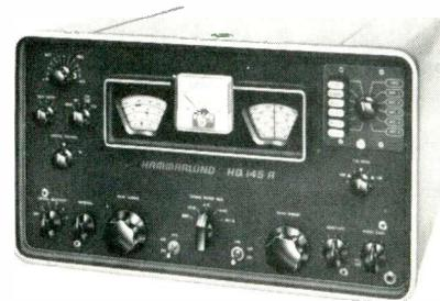
40, 20, 15, and 10 meter amateur bands; dual conversion above 10.0 Mc; six position crystal filter plus adjustable slot filter with up to 60 db attenuation; adjustable BFO for SSB and CW. A 1  $\mu$ V sensitivity gives 10:1 S/N ratio, the manufacturer says. Hammarlund.
