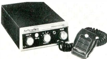
model CB-10, provides full modulation with 3.5 w of audio output through the three-stage transmitter. Power requirement is 1.0 amp maximum. The unit uses 14 transistors, 6 diodes, and 2 zener diodes. Receiver sensitivity in less than 1  $\mu$ v for 10 db S/N. Chassis dimensions are 2 $\frac{5}{8}$  x 6 x 9 $\frac{1}{2}$  in. Shipping weight 5 $\frac{1}{2}$  lb. The transceiver is supplied with push-to-talk microphone, mounting hardware, and channel 11 crystals. \$149.95 list. Hallicrafters.
