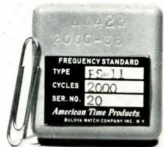
roduced. The output of type FS-11 is a limited sine wave of 3 v P-P min into 30k Ω. Standard input voltage is 28 vdc with units of lower input available. The unit is in a flat can 1 1/2 x 1 1/2 x 3/8 in., with a 6 pin termination for circuit board applications. Operating temperature is -5 to 85° C and it weighs 1 1/2 oz. Bulova.
