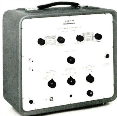
adjusting the thickness and number of horizontal and vertical bars or dots. The unit is designed for checking TV system linearity and is used with a linearity test pattern. Cohu.
