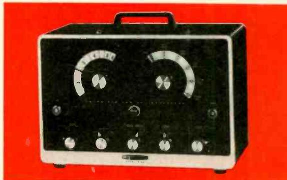
**Heath Model IG62 Color Bar/Dot Generator** Keyed rainbow type color signals. Patterns include dot, cross-hatch, horizontal, vertical, shading and color bars. Has 13 tubes.
