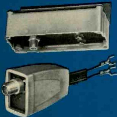
**COLORAXIAL MATCHING TRANSFORMERS AND KITS** Model TO-374A mast-mounting transformer converts any existing 300-ohm outdoor antenna to 75-ohm Coloraxial operation. Model T378 mounts on set to match it to 75-ohm coax. Available separately or as a set in Kit Model CAT-2.
