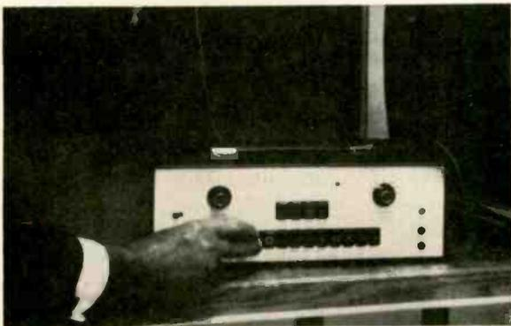
**Jackson Model 800 Bar/Dot Generator** NTSC type color signals. Patterns include cross-hatch, horizontal and vertical lines, dots and color bars. Gun killer. Has 14 tubes.
