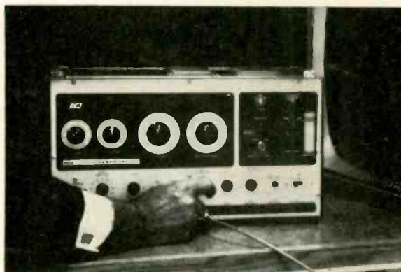
**B&K Model 1076 Analyst** Keyed rainbow type color signals. In addition to this instrument's broad TV signal substitution and troubleshooting facilities for all primary B/W TV circuits, this complete flying spot scanner provides white dot, white line and cross-hatch patterns for color TV convergence, adjustments and for signal tracing color circuits. It produces color bar chroma and burst signals. Has 16 tubes plus 5 in. scanning tube.
