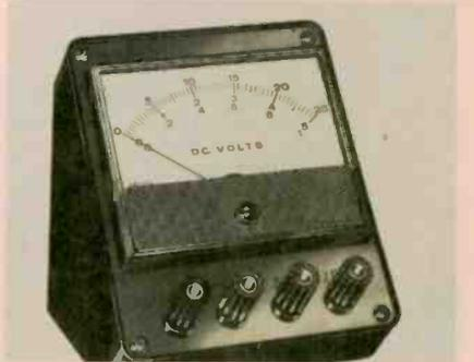
has a 3 1/2 in. plastic meter with a knife edge pointer. The molded plastic cases measure 4 3/16 x 3 7/8 x 4 3/16 in. Triplet.
