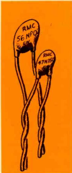
Fig. 1—A 44 pf N750 and 56 pf NPO capacitor are paralleled to obtain a total of 100 pf with TC of N330.
