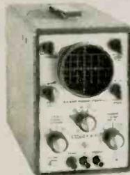
**5** New Model 435 - D-C Wideband Scope. Top-quality DC-4, 5Mc scope with 3" flat-face CRT, Zener calibrator. Outperforms 5" scopes three times its size, facilitates on-location color TV and other servicing. \$99.95 kit, \$149.95 wired.
