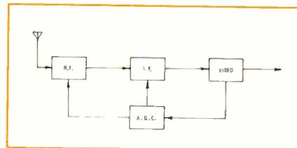
Fig. 1—Illustration of the 'closed loop' configuration of AGC system employed in most color TV receivers.
