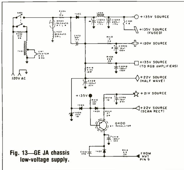
Fig. 13—GE JA chassis low-voltage supply.
