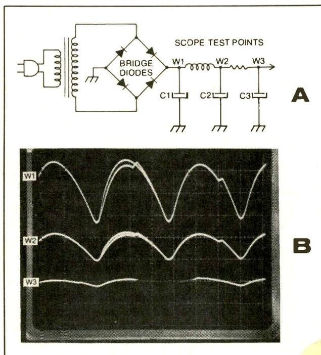
Fig. 26—Three-section filter system.
