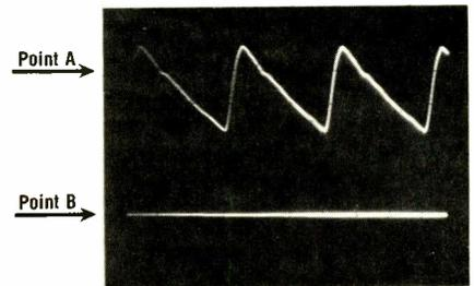
Fig. 2—Waveforms produced by the power supply circuit shown in Fig. 1. (A) shows the ripple present at point A in Fig. 1. (B) shows the waveform at point B in Fig. 1, after regulation.
