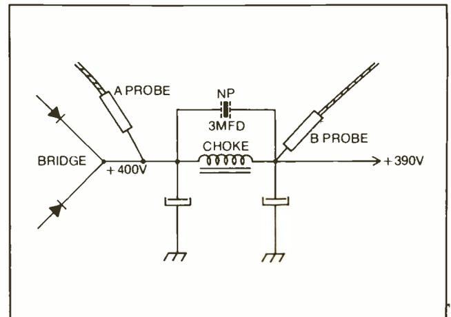
Fig. 23—Dual-trace connections for checking the filter system.
