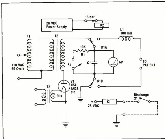
Fig. 4—A simplified schematic of a typical defibrillator.
