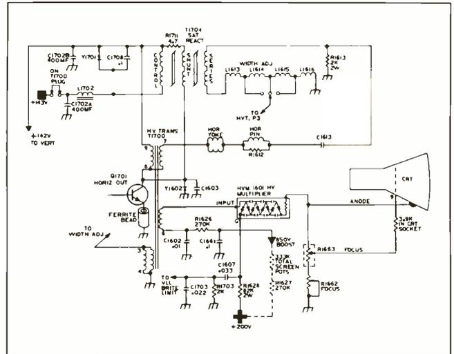
Fig. 9—GE MC chassis filter and high-voltage circuits.
