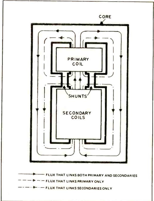
Fig. 1—Constant-voltage transformer construction.
