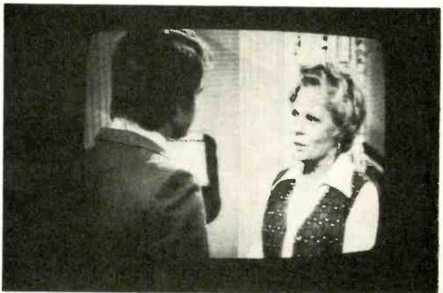
Fig. 5—Good picture even at a line voltage of 60V.
