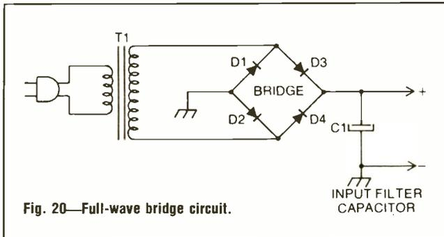
Fig. 20—Full-wave bridge circuit.
