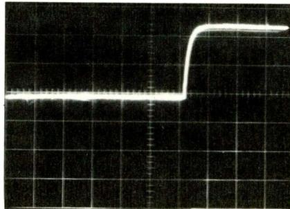
Fig. 4—A slightly damped waveform produced at turn-on in a high capacitance power supply.
