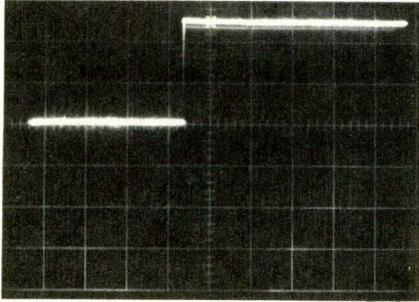
Fig. 3—A normal rising waveform of a positive power supply that is mostly resistive.
