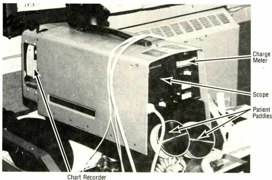
Fig. 3—A battery-operated portable defibrillator.
