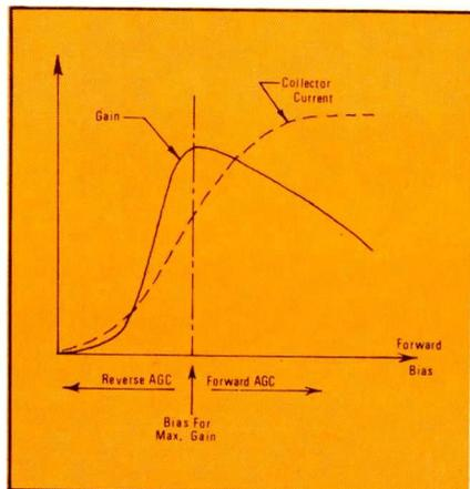
Fig. 2—Graph which illustrates that the gain of a transistor can be reduced by either increasing ('forward' AGC) or decreasing ('reverse' AGC) the base-emitter forward bias.
