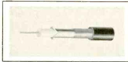
causes of poor reception. The new cable consists of a 20 AWG bare copper conductor insulated with cellular polyethylene. The shield is wrapped and adhesive bonded over the insulation. A 95% tinned copper braid shield supplies additional shielding and the entire assembly is protected by a black vinyl jacket with a nominal overall diameter of 195 inches.
