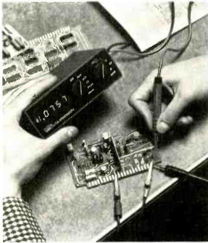
high-resolution unit offering 4½ digit resolution on all parameters. It is convertible for bench use with an optional bench stand, and features 10 microvolt sensitivity DC and AC and basic one-year accuracy of ±0.05% of input. Most logic components in the Model 248 are contained in a single LSI chip. It has only two controls, function and range. Priced at \$345.
