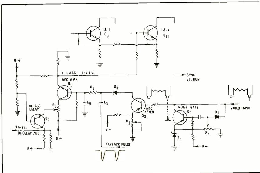
Fig. 3—A typical all-solid-state keyed AGC system.
