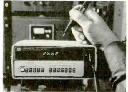
measurement range is from 10 nanoamps to two amps. The DMM, with rechargeable nickel-cadmium batteries, sells for \$500. The touch-hold probe sells for \$40.
