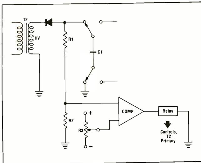
Fig. 5—A simplified schematic of the automatic charge control circuit in a defibrillator.
