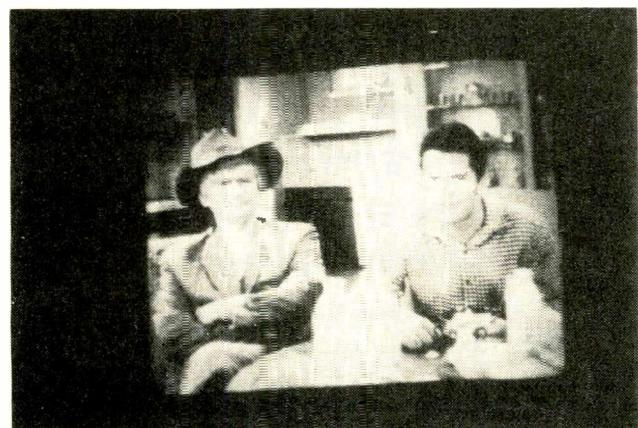
Fig 8—Small picture caused by open C1207.
