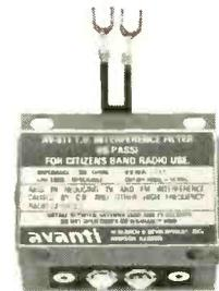
**AV 811 TV interference filter (hi-pass)** installs in TV antenna line and supplements inadequate TV filtering to prevent interference between TV or FM and CB or other high frequency radio services.
