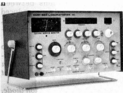
nels, and permit visual alignment of IF filters. CB-2700 also includes a phase locked loop oscillator permitting on knob selection of any of the present 40 channels with LED display of the channel. Priced at \$990.
