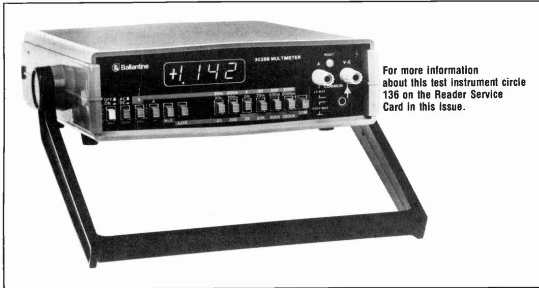
■ Ballantine Laboratories have just introduced a new portable rms responding digital multimeter with a sensitivity of 10 mV Full Scale and it is their claim that it is the only 3½ digit DMM to have 10 uV resolution and the capability to measure 10 milliohms.
