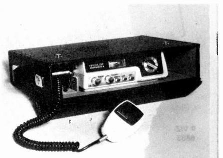
out removing the unit from the case. Openings at the top and bottom of the case allow the speakers to be heard, and a large opening at the back of the case permits antenna and power connections. The front flap folds down so radio controls and mike jack are accessible. A heavy duty handle is connected to the case, which is covered with durable Texion vinyl. It is designed for use with all major brands of CB.
