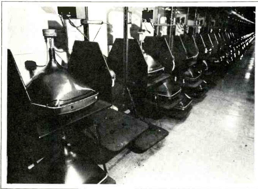
Fig. 8—Finished picture tubes are “aged” at voltages many times higher than would be encountered in actual use.
