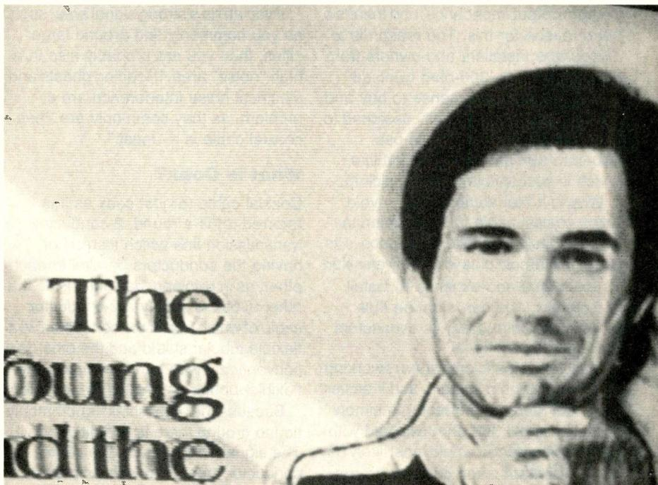
Fig. 1. Leading ghosts result from signals induced in the transmission line between the antenna and TV set. Short sections of open line (twinlead) act like an antenna inducing voltages that arrive at the set ahead of the main signal. Because the picture image "grows" from left to right on the screen, leading ghosts appear to the left of the main image.
