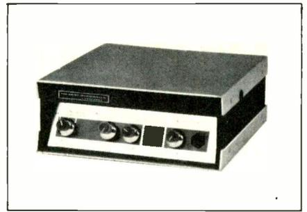
ohms. The Model S-402 is an ac powered unit with background music capability and paging override. The manufacturer states it can power up to eight speakers and operates from 12V dc for emergency use. The S-702 is a portable amplifier designed to operate, according to *Perma Power*, for 200 hours on one set of alkaline "D" cells. It delivers 35 watts nominal battery powered output.
