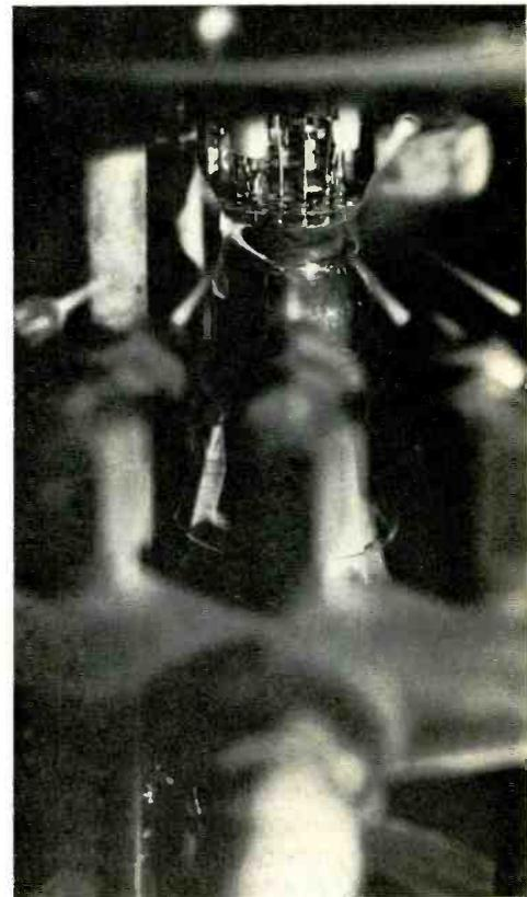
Fig. 7—In one of the final steps the neck glass is fused to the glass stem and then cooled.
