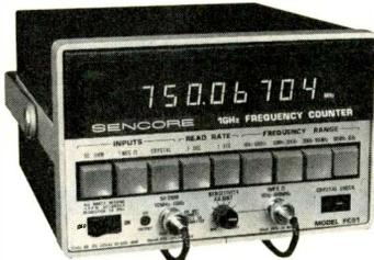
Fig. 17—Sencore's FC51, 1000MHz counter, can also count frequencies as low as 10Hz with up to .01Hz resolution.
