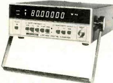
Fig. 9—Leader's 80MHz, seven digit LDC-822 features period function and 10MHz time base.
