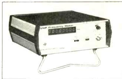
Fig. 23—Racal-Dana's Model 9313 200MHz counter has packaged the equivalent of over 5000 components on a single chip.
