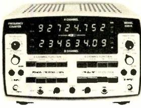
Fig. 14—A dual channel counter/timer, Systron Donner's Model 6361A. Both channels are identical and capable of counting to 100MHz.
