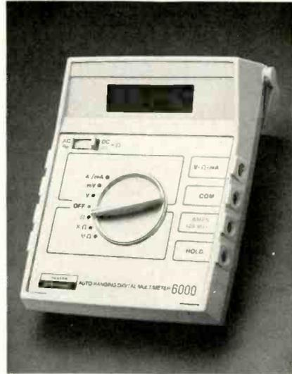
changing is automatic. Measurement ranges are dc and ac volts from .1mV to 1000V, dc and ac current from .001mA to 10A and resistance from .1 ohm to 19.99 megohms. The accessories include a hold probe which will hold a reading if the operator's eyes have to remain on the test point during measurement, a light meter attachment, HF and VHF RF probes, a 50KV high voltage probe, an ac clamp on amp-meter and a carrying case.
