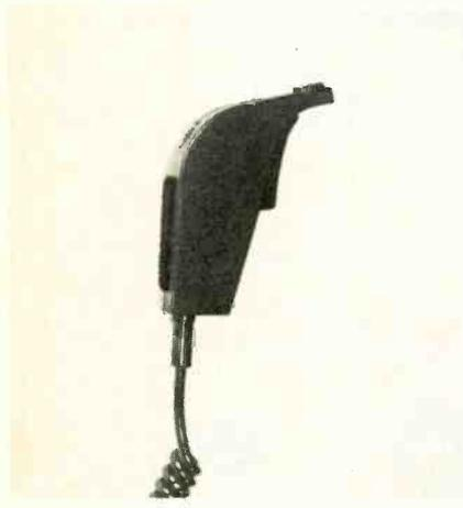
JMR Systems Corporation has produced a new acoustically designed, high fidelity, noise canceling, handheld mobile microphone. Designated the Model 45 Silencer, it is stated to be insensitive to noise originating within a few inches of the microphone, enabling the user to talk through the noise of most noisy environments. It is said to be a result of the firm's experience in developing and manufacturing aerospace-communications equipment.
