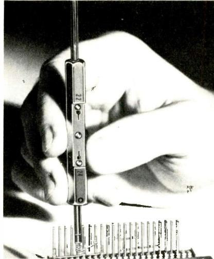
The compact, inexpensive *WSU-2224* tool, from *OK Machine and Tool*, wraps, unwraps and strips wire, thanks to a unique built-in stripping blade. Designed for use with 22-24 AWG (0.65-0.50mm) wire on standard .030 x .060 in. (0.76 x 1.52mm) and .045 in (1.44mm) square posts. Reportedly takes minutes to learn to use and makes connections in seconds without solder. Priced at \$12.75.
