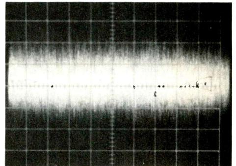
Let's "look at" the formula. It says that the noise voltage is the square root of the factors on the right hand side of the equation, and that the noise increases if the temperature increases, or if the resistance increases, or if the bandwidth increases. Let's crank in some practical figures as examples, using room temperature of 25 degrees centigrade, which is 298 degrees Kelvin. (Zero degrees Kelvin is *minus* 273 degrees centigrade, and is the point where atomic motion stops.)
