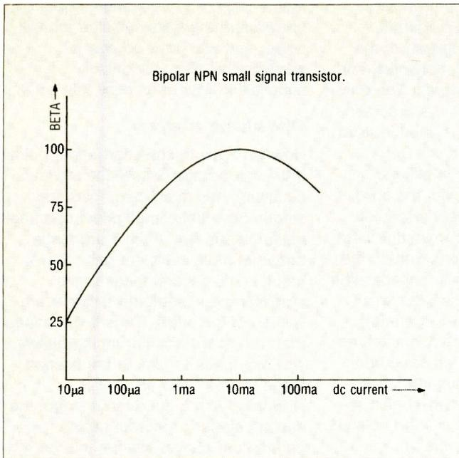
Fig. 1-The gain falls off at low current and at current above the level of the transistor's design.
