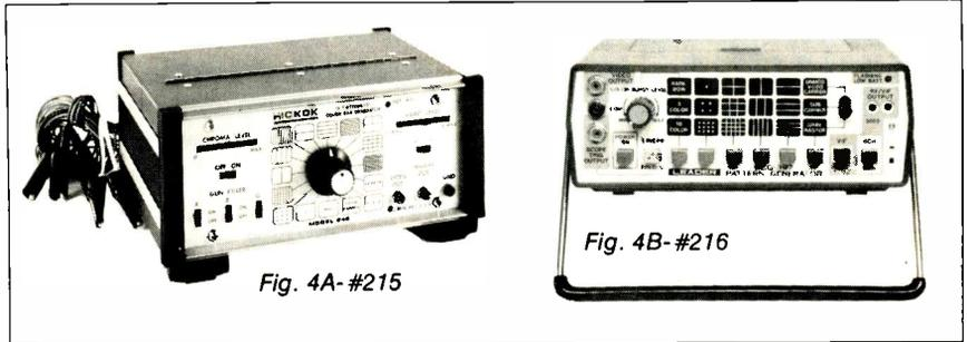
Fig. 4 - Two state-of-the-art progressions on the standard color bar generator are offered in portable form by Hickok and Leader. Operating on two standard 9 volt batteries Hickok's Model 246 (A) offers 16 basic patterns. Leader's Model 397 (B) offers 18 patterns and operates on four "c" cells. Both have adjustable color burst and RF, IF outputs.
