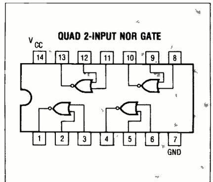
Fig. 3B—A TTL NOR gate, the 7402.
