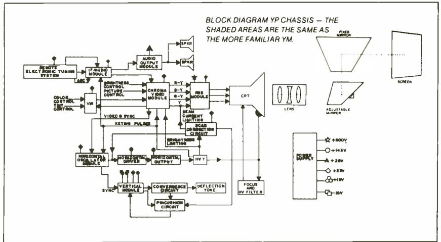
Fig. 2—Block diagram of the Y-P chassis. The shaded areas are the same as the Y-M. (Courtesy GE.)
