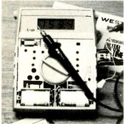
View of unit with range panel removed. Note easily accessible adjustment pots, the batteries and fuse compartments, plus the 153.4mV reading being "held" by the mold probe.
