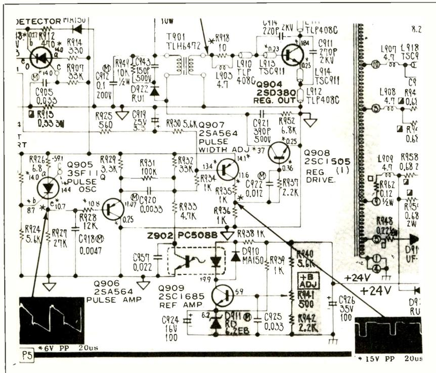
Fig. 6-The Quasar opto-coupler voltage regulator. (Courtesy Quasar Electronics Company.)
