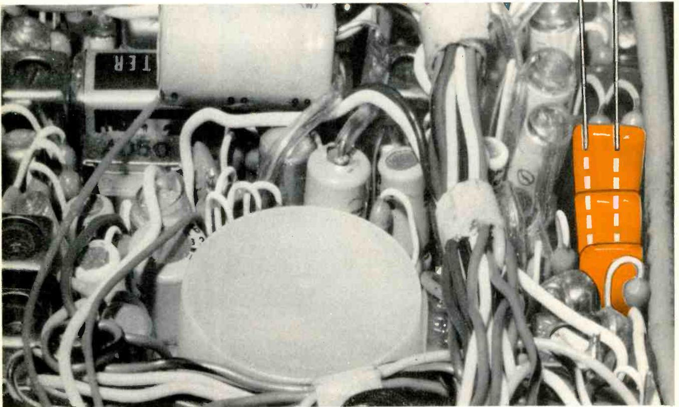
Low-cost Verti-Film<sup>★</sup> epoxy-coated polyester-film capacitors help you beat the cost/space squeeze when servicing imported communications and entertainment electronic equipment, letting you make exact replacements on crowded PWBs quickly and easily. Their single-ended design permits vertical installation in far less space than required by conventional axial- or radial-lead film capacitors.
