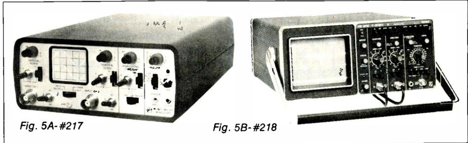
Fig. 5 - Still in their "infancy," portable oscilloscopes appear to be likely candidates for evolution in the portable market. Two companies at least are in (A) Non-Linear with its "mini" dual trace 15MHz, 4-by-5 cm CRT and Philips with two 25MHz versions; the Model 3212B is shown here (B). Obviously power requirements are still a problem with scopes. Philips is rated at 2.6 hours continuous use while Non-Linear says its unit will go for three hours.
