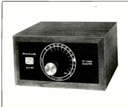
a noise figure of 7dB, spurious rejection of 90dB minimum, and image rejection of 85dB minimum. It uses three RF stages and has a price of \$150.
