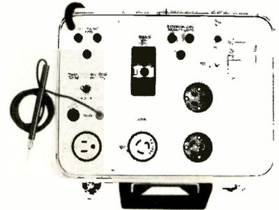
A new lightweight, rugged, all-in-one tester that checks for OSHA compliance of polarity, grounding and line leakage in 120 volt power tools, cord sets and receptacles is now available from *General Scientific Equipment Co.*, Philadelphia, Pa. The unit, called Multi-Check, provides simple visual indicators for "GO" or "NO-GO" operation, permitting a check of equipment in seconds. There are no scales to read, no readings to interpret. Instructions are printed on the
