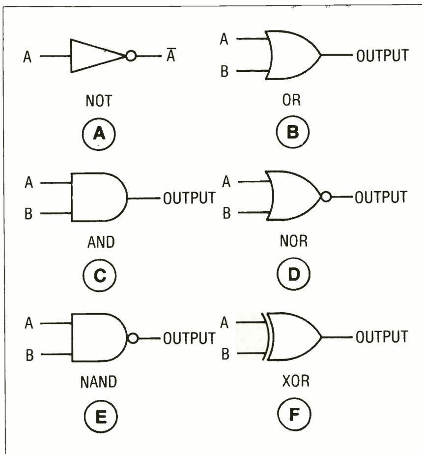
Fig. 1—Digital logic circuit symbols, A) NOT gate (inverter), B) OR gate, C) AND gate, D) NOR gate, E) NAND gate, and F) Exclusive-OR (XOR) gate.
