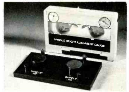
quickly check spindle height and prevent VCR tape edge damage. A *Memorex* spokesman states that checking spindle height alignment took a technician up to four hours previously; the SHAG can do it in 30 seconds. The suggested retail price is \$695.00.
