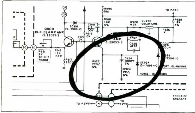
Color TV Chassis 19GC45—Hum bars, reduced height, distorted audio, no color. Possible cause—shorted CX216—low voltage power supply filter/capacitor. No set up line, dark picture, green streaking. Possible cause—shorted C208 in red G2 circuit. ET/D
