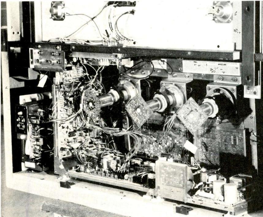
Fig. 3—The Quasar Projection Television Model PR6800QW interior view showing modular construction and the three CRTs. (Courtesy Quasar Electronics Company.)
