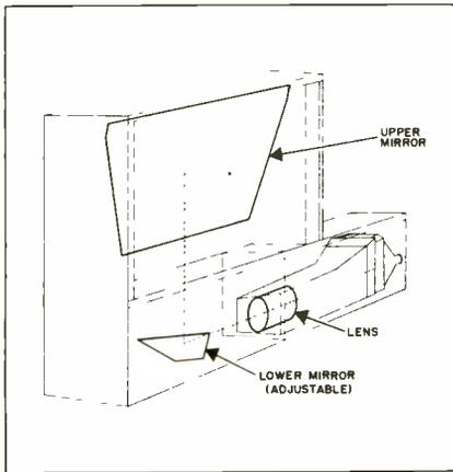
Fig. 1—Optical system of the GE Widescreen 1000. Mirrors direct the light from the projection lens onto the viewing screen. (Courtesy GE.)
