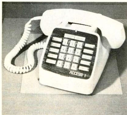
Electronics Corporation. The new telephone is a repertory dial telephone known as Access I. It can be programmed in seconds to remember nine frequently called or emergency numbers and automatically will remember the last number dialed manually. By depressing just two buttons, any of the stored numbers will be dialed automatically.
