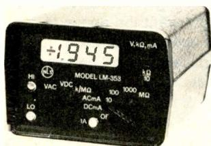
Non-Linear Systems new Model LM-353 3½ digit Digital Voltmeter includes voltage ranges to 1000V ac and dc, resistance ranges to 10,000 K ohms and current ranges to 1000 MA, all in a 9.2 ounce package measuring 1.9 inches high by 2.7 inches wide by 4 inches deep. Additionally the ohms ranges can be operated at a low applied voltage to avoid turning on semiconductor junctions. The LM-353 uses a LCD display and operates up to 100 hours on standard AAA cells and sells for \$149.50.
