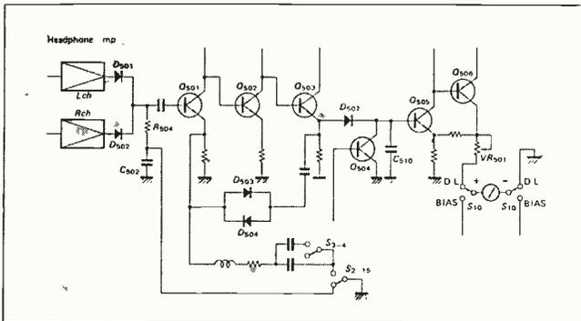
Fig. 3 Pioneer's peak meter circuit
