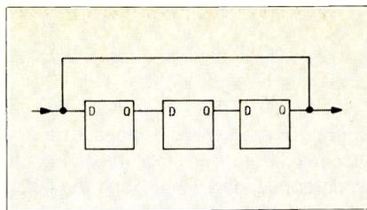
Fig. 5 A recirculating register automatically rewrites the data back into the device.
