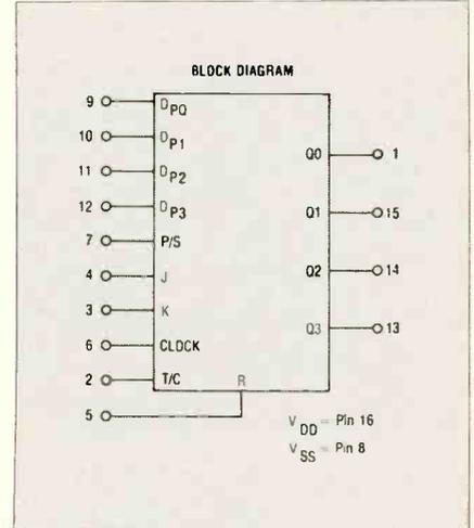
Fig. 13 A block diagram of a 4035, considered virtually a universal register usable in many shift register applications.
