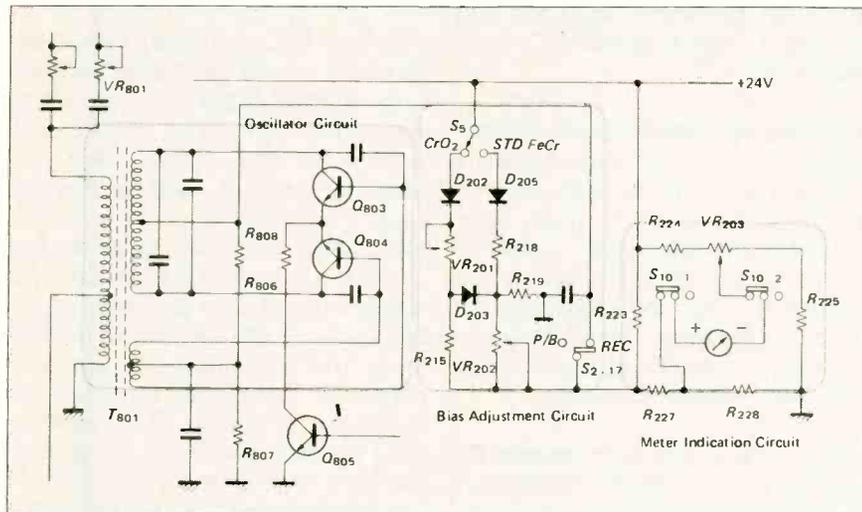
Fig. 9 The bias adjustment circuit in the CT-700
