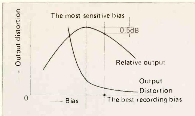
Fig. 6 Relation of level of bias, output and distortion
