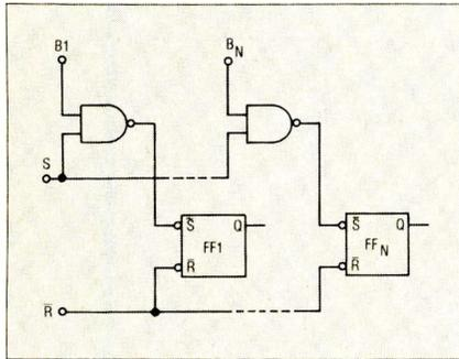
Fig. 3 The "parallel" entry shift register.
