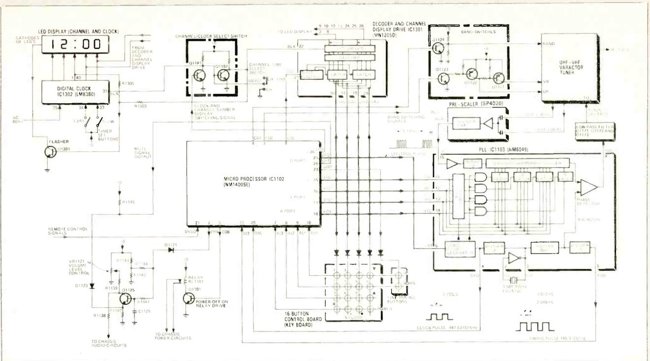
Fig. 2 Synthesizer tuning system block diagram
