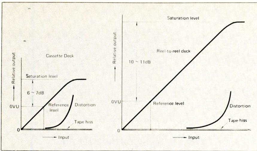
Fig. 1 Characteristics of input and output for reel-to-reel and cassette decks
