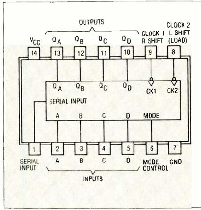
Fig. 6 A basic, four bit PIPO register.
