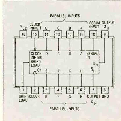
Fig. 9 The 74165 SISO/SIPO device triggers on positive going transitions.
