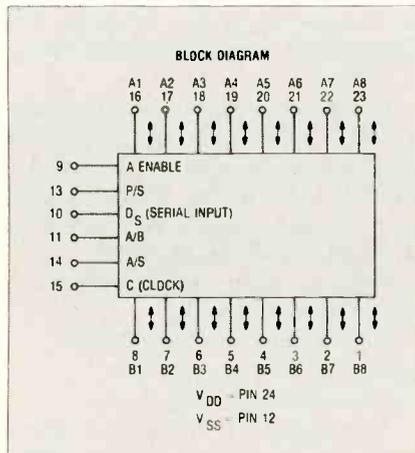
Fig. 12 The 4034 is a bidirectional register used to interface various buses. It may be programmed using four control lines.
