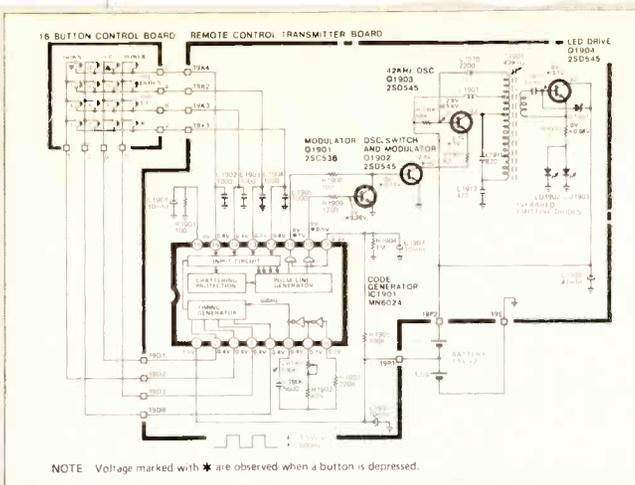
Fig. 7 The remote control transmitter
