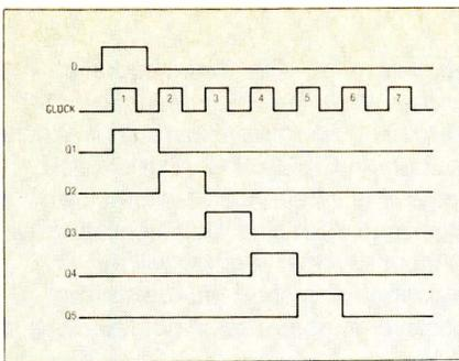
Fig. 2 The progression of a single bit of information through a serial in, serial out shift register.
