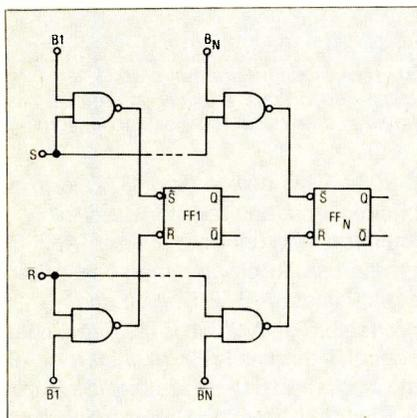
Fig. 4 The "jam" loaded parallel entry register.
