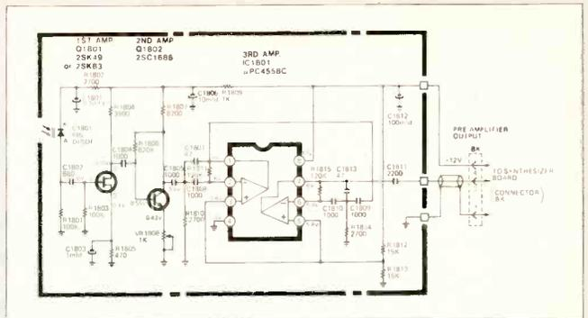
Fig. 8 Remote control preamplifier
