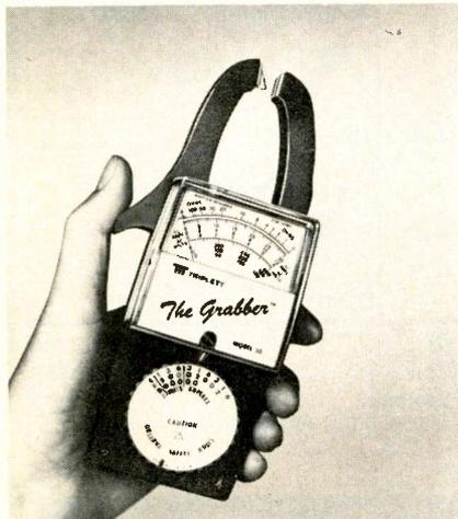
Triplet has just introduced a new clamp-on ammeter/ac voltmeter designated the Model 30. It features a one inch opening and a "Memo-Loc" pointer to permit out of sight measurements. Meter ranges cover 0-300 ac amperes in six ranges, 0-600Vac in three ranges and a ten ohm center scale ohmmeter range with an optional adapter. A leather carrying case is also available. The price is \$65.00.
