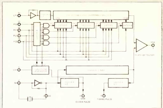
Fig. 4 PPL IC block diagram
