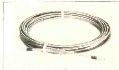
Klein Tools has a new series of round flexible fish tapes which they call Klein-Flex. Reportedly extremely flexible these tapes are made of braided spring steel music wire and have pull loops on both ends. They are available in 25, 35, 50, 75 and 100 foot lengths; special lengths on special order. **ETD**
