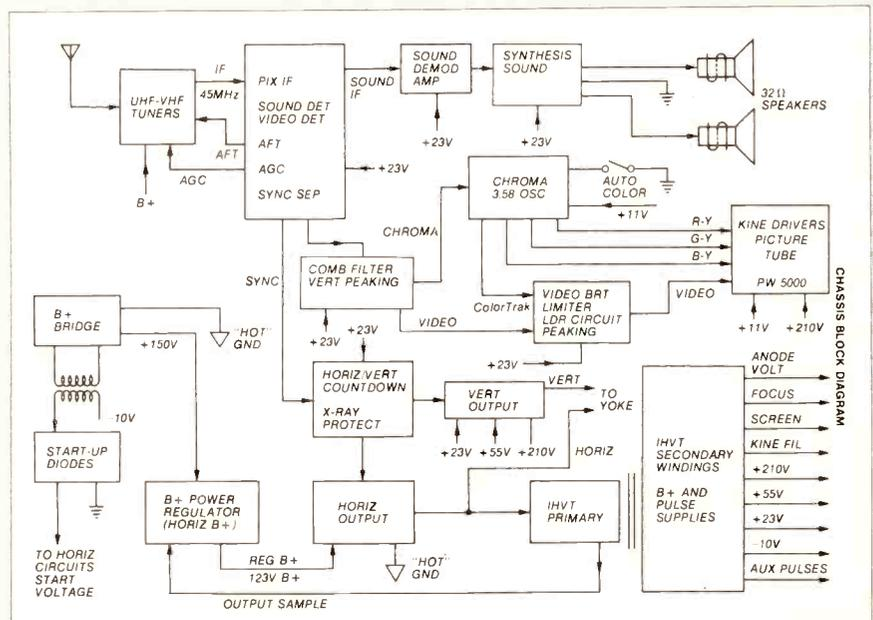
Fig. 1—Block diagram of the RCA CTC101 series.
