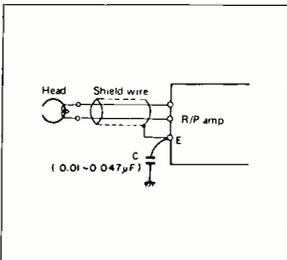
**Induced in the tape deck.** Connect C, specified head lead wire, to the chassis. Also, replacing the head leads with the shielded wire is sometimes effective, if the shielded wire is not employed. **Caution:** Never connect a capacitor to the signal line.
