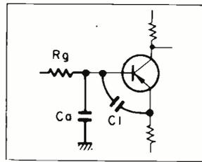
In a conventional amplifier, type 1, add a 47 to 100pF capacitor to C1 between the emitter and base. Also replace Rg and Ca with larger value components, but not exceeding 2.2Kohms and 100pF.
