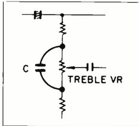
If Amp 1 is entering through tone control circuits employing B-type VRs (VAX or LUX), insert a capacitor across the treble control volume. The values should be 470 to 680pF: 100Kohms up to 1000pF: 10Kohms.
