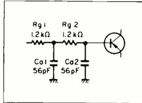
For a type 2 conventional amp, divide the filter consisting of Rg and Ca into two stages to get a sharper effect. The value of the parts should be:
