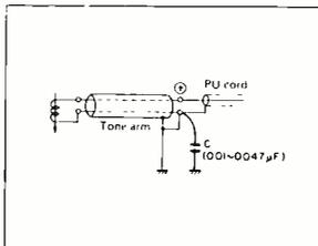
**Induced in phono cartridge or turntable lead wires.** Connect the earth lead to the ground via the capacitor specified; employ the shortest route from the tonearm to the chassis. Never connect to the positive lead.
