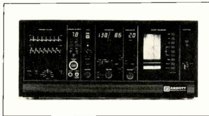
Fig. 3 A typical state-of-the-art patient monitor capable measuring heart rate, displaying analog waveforms of direct blood pressure and heart action, graphic "hard" copy of any parameter in the cabinet as well as cardiac output and a second direct pressure expressed in  $\text{CmH}_2\text{O}$ . (Photo courtesy Abbott Medical Electronics)
