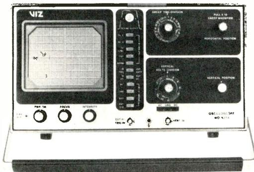
The ideal scope for most industrial, laboratory, educational and servicing applications. Frequency response DC to 15MHz. Rise time 23 nsec. Sensitivity 10mV/cm P-P. Ultrastable trig action with simplified level adjustment and LED polarity indicators. One direct/X10 LoCap probe supplied.
