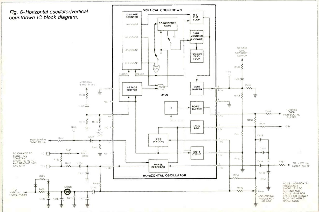
The two modes of operation allow the system to be compatible with nonstandard sync signals. The IC internally switches between the two modes of operation depending upon the type of signal being received. Mode switching occurs after eight consecutive cycles of receiving vertical sync that is either in coincidence or not in coincidence with the 525 count from the countdown system.
