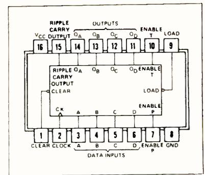
Fig. 9 Pinouts for the TTL series 74160-74163.
