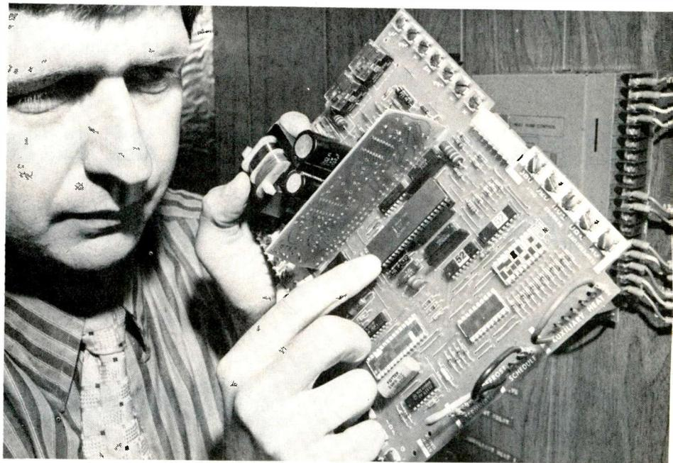
*Fig. 1—A sophisticated, programmable microprocessor is the heart of this advanced heat pump control system from Honeywell's Residential Controls Center. Transducers encode indoor, outdoor and wall temperatures in home or office buildings for computerized control of indoor air flows.*
