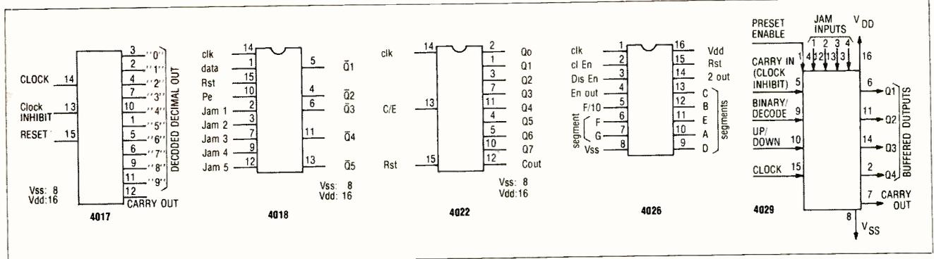
Fig. 10 The pinouts for several popular CMOS counters.
