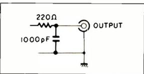
**Induced in the signal line of the tuner.** Connect a specified RC filter to the output terminal.
