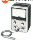
AC RMS/DCV: 0-1, 3, 10, 30, 100, 300, 1000V. P-P ACV: 0-2.8, 8.5, 28, 85, 2800V. DC. Input Z 11 MΩ. Ohmmeter 0.2Ω to 1000 MΩ. 4½" 200 μA meter. Eico 240, Kit \$59.95, Wired \$79.95. With 6½" meter & AC/DC Current readings.
