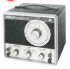
Provides simultaneous sine and square wave outputs. Covers 20 Hz-2MHz, 5 bands. Max. distortion 0.25%. Rise time at 20 KHz <0.1 µsec. Eico 379, Kit \$69.95, Wired \$94.50.
