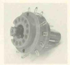
Fig. 8—With this test socket we can connect the test-instrument leads almost directly to the pins of the color picture tube, thus eliminating the vector-pattern distortion.
