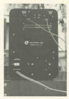
Fig. 1—The back of this instrument contains the B-Y and R-Y signal inputs, two switches for changing the instrument from an oscilloscope to a vectorscope, plus horizontal and vertical vectorscope centering controls. (As with other vectorscopes, a ground lead must also be connected between the instrument and the TV set.)
