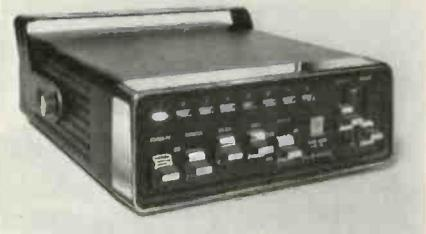
75, the solid-state receiver reportedly covers the 150 to 175MHz band. The scanning system automatically monitors on a sequential basis all eight channels within one second by means of electronic switching. A by-pass feature lets the receiver skip selected frequencies. Price: \$149.95. Fanon Electronics.
