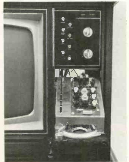
Front view of the TV-set console with tilt down convergence and secondary control panel, simplifying set-up adjustments.
