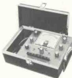
For all B-W & Color Picture Tubes. Each gun of Color Tube measured individually and numerically, provides required gray scale tracking information. Eico 633, Kit \$79.95, Wired \$109.95.
