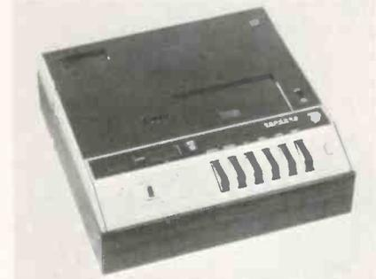
microphone are accessories included with the recorder. The unit measures  $10\frac{1}{2}$  in. D by  $10\frac{1}{4}$  in. W by  $3\frac{1}{2}$  in. H and weighs 4 lb 6 oz.
