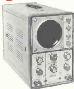
DC-8MHz (usable to 10 MHz). 5" flat-face CRT. Sensitivity 12 MV RMS/CM. Negligible relative H & V phase shift. Excellent curve tracer with Eico 443 (below). Eico 465. Kit \$179.95. Wired \$249.95.
