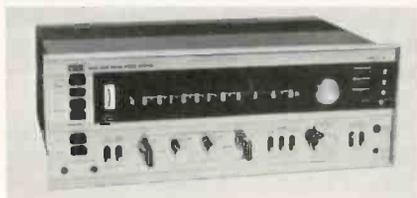
circuit in the FM section, providing full noise suppression. When tuned accurately the "center tune light" illuminates and the sound goes ON.
