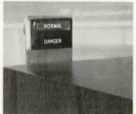
sets, emits a red warning signal whenever TV-set voltage rises above a permissible level. According to the manufacturer, the device may be quickly attached to any color-TV set, and con-
