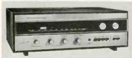
(main and remote). Output terminals are provided for a separate mono extension speaker. Other front panel conveniences include a stereo headphone jack for private listening, switches for loudness contour defeat, stereo/mono, tape monitoring and high filter. A zero-center tuning meter pinpoints FM tuning and the receiver has an FM output distortion as low as 0.2 percent at 100 percent modulation on FM, plus  $-95$ dB spurious response rejection to reduce interference in difficult signal areas.
