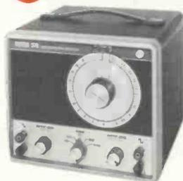
Provides simultaneous sine and square wave outputs. Covers 20 Hz-2MHz, 5 bands. Max. distortion 0.25%. Rise time at 20 KHz <0.1  $\mu$ sec. Eico 379, Kit \$69.95, Wired \$99.95.
