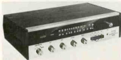
pre-aligned for easy construction. The preamp controls inputs and outputs for every music program source, and the FM tuner circuit has time-switching multiplex for mono and stereo FM reception.
