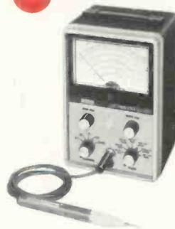
AC RMS/DCV: 0-1, 3, 10, 30, 100, 300, 1000V. P-P ACV: 0-2.8, 8.5, 28, 85, 280, 850, 2800V. DC Input Z 11 M $\Omega$ . Ohmmeter 0.2 $\Omega$  to 1000 M $\Omega$ . 4 1/2" 200  $\mu$ A meter. Eico 240, Kit \$59.95, Wired \$79.95. With 6 1/2" meter & AC/DC Current readings. Eico 242 FET-TVOM, Kit \$69.95, Wired \$94.50.
