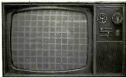
Fig. 4—TV picture produced when TV set and analyst are both tuned to Channel 30. All other UHF channels are also available from the analyst.
