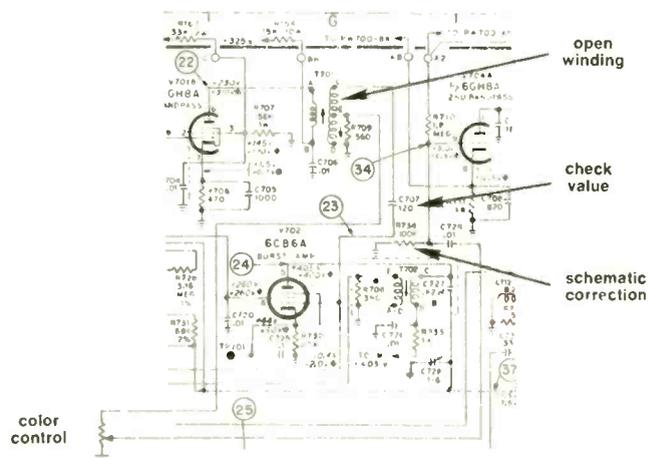
the winding connected between terminals C and E, the color signal input to the burst amplifier stage will be incorrect. However, the path for chroma input to the second bandpass amplifier stage will be normal.
