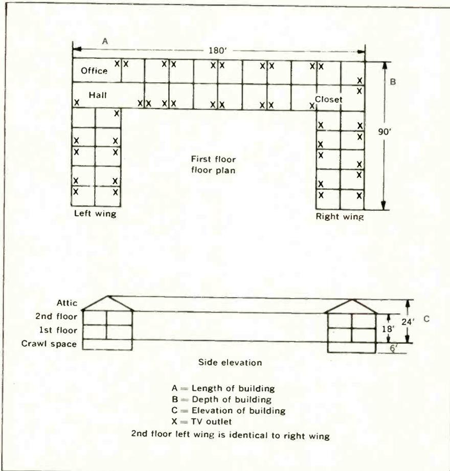
Fig. 2—A typical layout for a motel or school requiring a distribution system.
