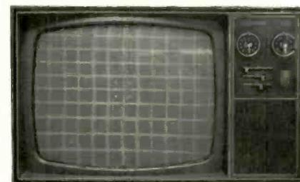
Fig. 8—TV picture produced when IF signal is fed to collector of second IF transistor.
