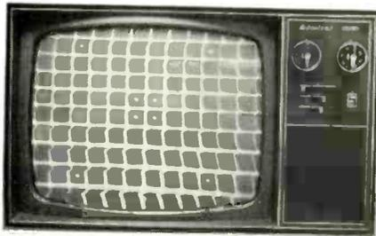
Fig. 11—TV picture produced when video signal is fed to base of first video amplifier transistor.
