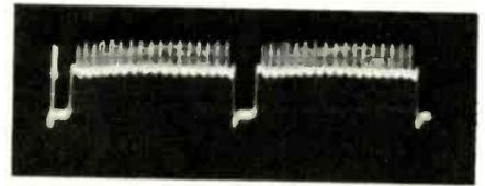
Fig. 18—Waveform of signal received at Terminal G of printed-circuit board when an RF video signal is applied to the TV set and the scope is synchronized to the TV set and analyst's horizontal sweep rate. The positive pulses correspond to the vertical lines in the test pattern.
