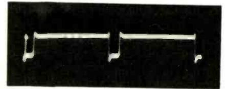
Fig. 17—Waveform of signal received at Terminal G of printed-circuit board when no RF video signal is applied to the TV set and the scope is synchronized to the TV set and analyst's horizontal sweep rate. The negative pulses are formed by the horizontal sync signal.
