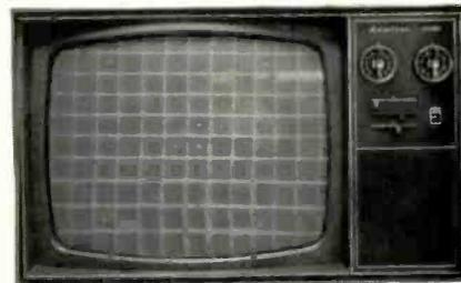
Fig. 10—TV picture produced when IF signal is received from unattached analyst lead.
