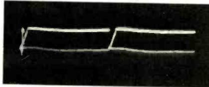
Fig. 14—Waveform of signal received at Terminal G of printed-circuit board when no RF video signal is applied to the TV set and the scope is synchronized to the TV set and analyst's vertical sweep rate. The negative pulses are formed by the vertical sync signal.
