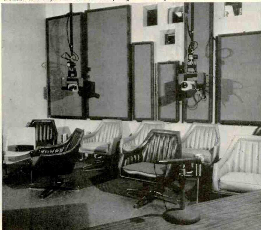
In the previewing room of the New England Telephone Company's TV system, two remote-controlled, ceiling-mounted cameras are used for self-critiques and role-playing.
