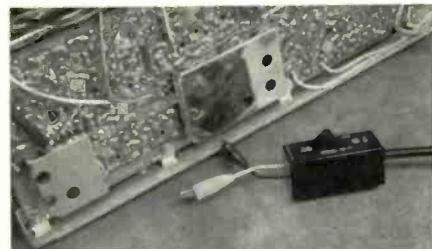
Fig. 9—Analyst lead injects IF signals into TV set even when not physically attached.
