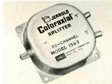
cable. An expansion tool, ET-659, is supplied to expand the cable bushing for CAC or CAC-6 cable size. The 1563 splitter is said to have a splitting loss rated at 3.5dB for VHF and 3.8dB for UHF, with 18dB isolation between outputs and a frequency range of 54 to 890MHz. List price per unit is \$6.95. Jerrold.
