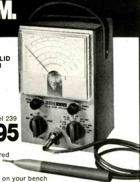
Use the new 239 on your bench or in the field. Checks semiconductor and vacuum tube circuits. 11 Megohm DC input impedance. Reads AC rms and DC voltages in seven 10db steps from 1 to 1000 volts on large 4½" meter. Measures and reads peak-to-peak AC to 2800 volts. Check resistance from 0.2Ω to 1000 MΩ on seven ranges. Includes exclusive time-saving Uniprobe.
