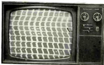
Fig. 13—TV picture produced when video signal is fed through delay line to grid of second video amplifier tube.
