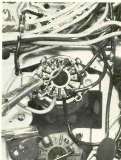
Fig. 11—Horizontal beat signals are eliminated by disconnecting horizontal oscillator from grid of horizontal-output tube (removing a resistor from pin 5 of tube socket) and injecting analyst horizontal grid-drive signal in its place.
