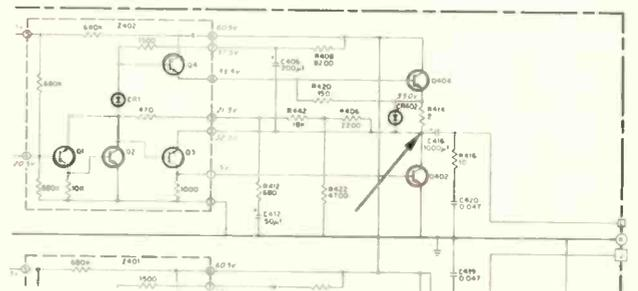
Before replacing a defective coupling capacitor, be sure the voltage at this point is correct. Possible causes of increased voltage include: shorted capacitor C411 or C412 (in illustration); open printed circuit; defective Z401 or Z402 board.
