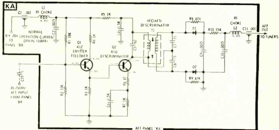
Fig. 3—Schematic of the automatic fine tuning circuit (AFT). Courtesy of Motorola Inc.
