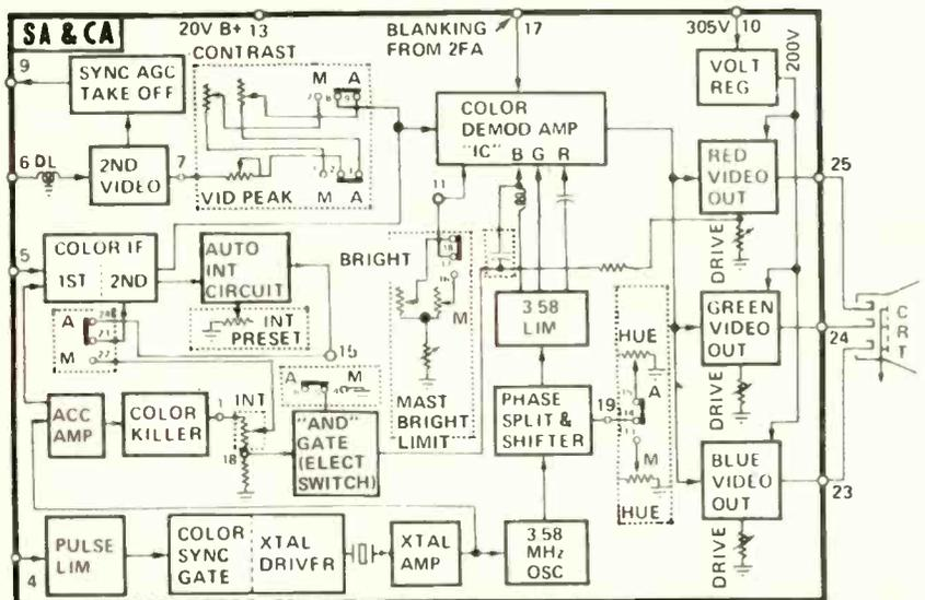
Fig. 1—Basic block diagram of the CA color panel with Insta-Matic color preset feature. Courtesy of Motorola Inc.
