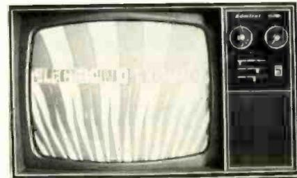
Fig. 20—TV picture produced when analyst vertical-grid-drive signal is fed to grid of vertical "output tube."
