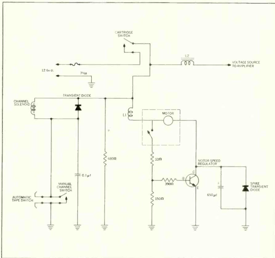
Fig. 2—Motor circuit for Ford Model IFD5003 stereo unit.
