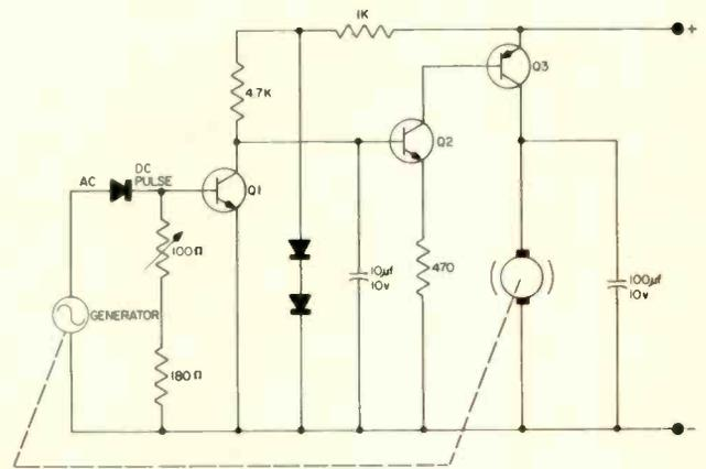
Fig. 2—Motor Generator Type Control
