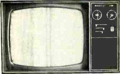
Fig. 21—Discontinuing injection of analyst vertical signal results in loss of test pattern.
