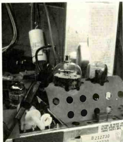
Fig. 13—By applying analyst's horizontal-plate-drive signal to cap of horizontal-output tube, while protecting this tube by removing its cathode fuse (lower right), TV set functions even though virtually its entire horizontal circuitry is bypassed.
