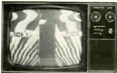
Fig. 7—TV picture produced when analyst horizontal-grid-drive signal is fed to grid of horizontal-oscillator tube.
