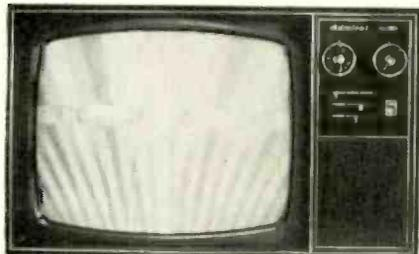
Fig. 9—Adjusting HORIZONTAL-HOLD control reduces beat signal shown on CRT.
