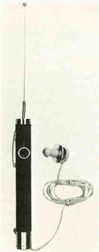
has a tunable range of 108MHz to 140MHz and works inside the aircraft without an outside antenna. The unit operates on two silver oxide hearing aid batteries which are included. Battery life is said to be approximately 25 hours. Price \$18.95. Saxton Products, Inc.
