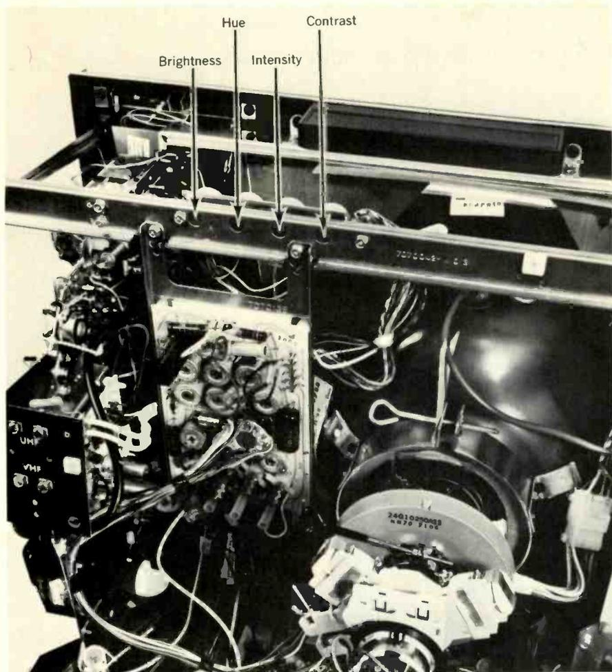
Rear view of the Motorola's color chassis TS-929 showing location of Insta-Matic preset controls.
