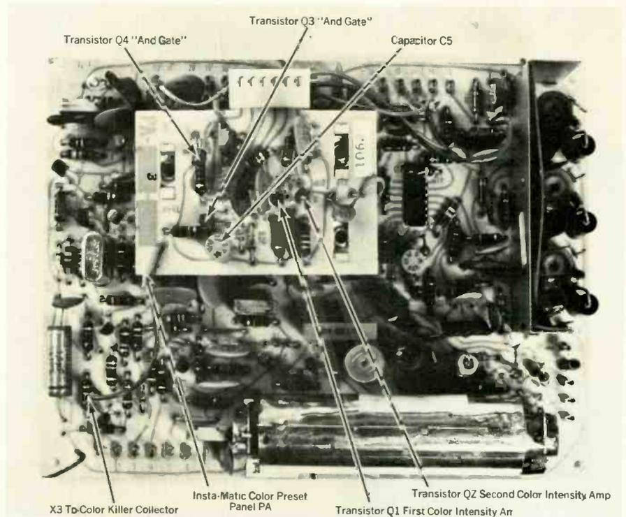
Location of some components on the color circuit panel CA and the color preset panel PA.
