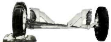
**Strong, smooth-riding Twin-I-Beam.** The independent front suspension that has revolutionized truck riding qualities. Two forged steel I-beam axles give it strength . . . big coil springs give it a smoother ride.
