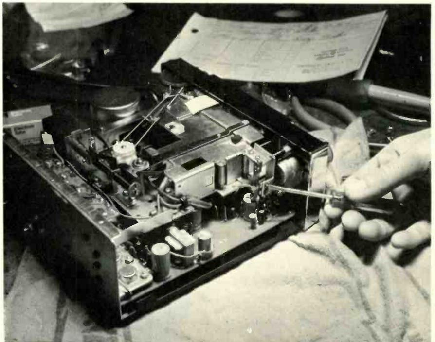
Fig. 6—An automatic channel switch with poor insulation to ground.
