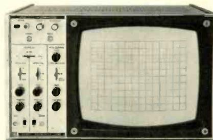
Virtually solid-state scope incorporates TV-type CRT for easier viewing
