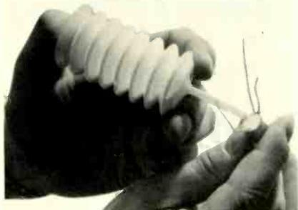
Filling of the syringe is accomplished by the plunger seal back, making the syringe suitable as a container for two-part material. Techni-Tool.
