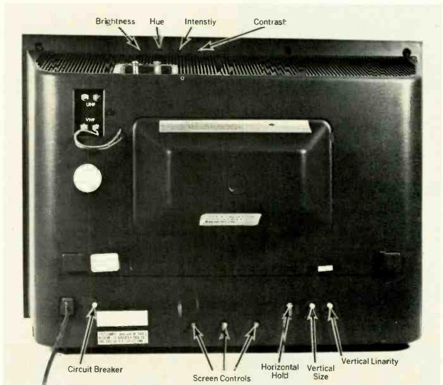
Rear view of Motorola's Model WP563GWA color-TV set, showing locations of service controls. The Insta-Matic preset controls can be adjusted with back cover in place.
