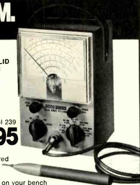
Use the new 239 on your bench or in the field. Checks semiconductor and vacuum tube circuits. 11 Megohm DC input impedance. Reads AC rms and DC voltages in seven 10db steps from 1 to 1000 volts on large 4 1/2" meter. Measures and reads peak-to-peak AC to 2800 volts. Check resistance from 0.2Ω to 1000 MΩ on seven ranges. Includes exclusive time-saving Uniprobe.
