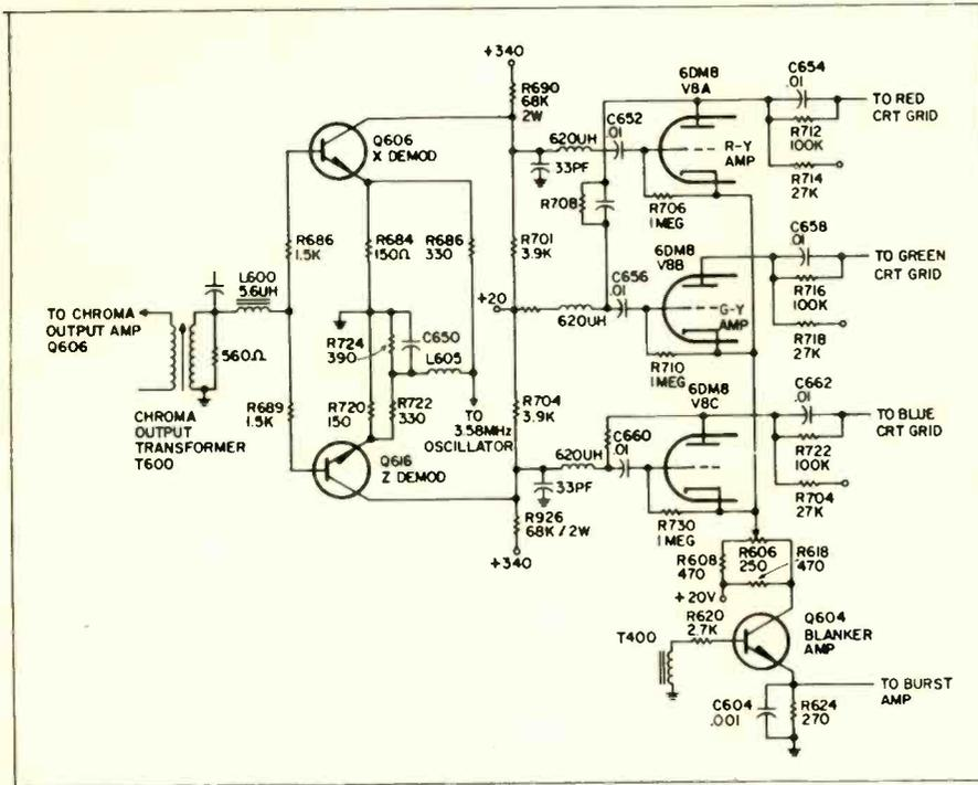
Fig. 6—Demodulators, and Color Difference and Blanking Amplifiers.
