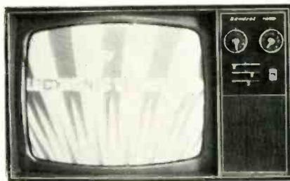
Fig. 15—Even though vertical-sync signal no longer functions, critical adjustments of VERTICAL-HOLD control still permit formation of desired test pattern.
