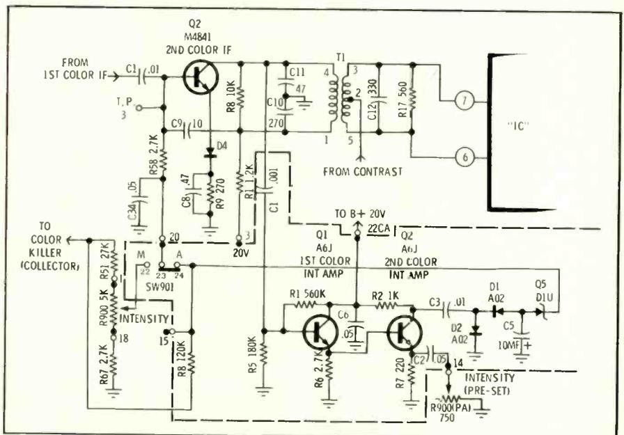
Fig. 4—Schematic of the automatic intensity circuit. Courtesy of Motorola Inc.
