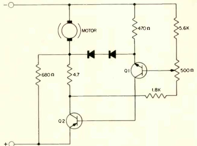
Fig. 3—Counter EMF Control Type Control
