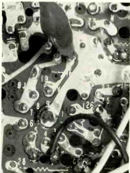
Fig. 3—Injecting analyst sync signal to grid of horizontal-oscillator-control tube.
