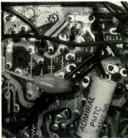
Fig. 22—Shorting grid of "oscillator tube" to ground (pin 10 of 25JZ8), prevents TV set from generating vertical scan signals. (Vertical sync coupling capacitor, CE11, is disconnected from printed circuit shown in upper central portion of photo.)
