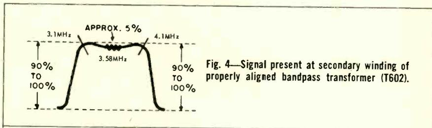
Fig. 4—Signal present at secondary winding of properly aligned bandpass transformer (T602).
