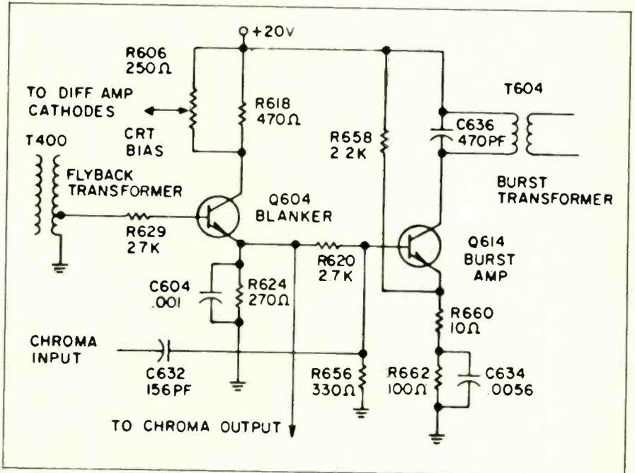
Fig. 9—Blanker Circuits.
