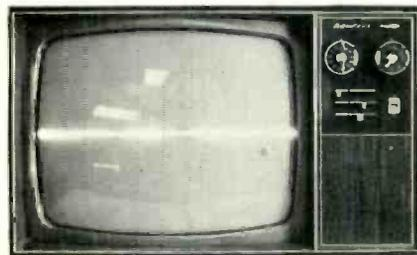
Fig. 23—Without vertical scan signal, only horizontal line appears on CRT.
