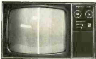
Fig. 8—Beat signal appears on CRT when both TV set's horizontal-oscillator signal and analyst's horizontal-grid-drive signal are applied to horizontal-output tube.
