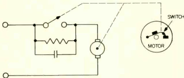
Fig. 1—Diagram of Centrifugal Switch
