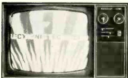
Fig. 4—TV picture produced when analyst sync signal is fed to grid of horizontal-oscillator-control tube.
