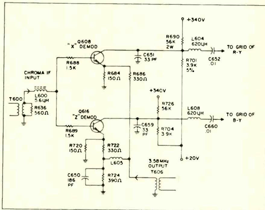
Fig. 5—X and Z Demodulators.
