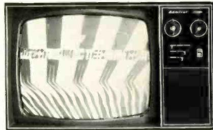
Fig. 18—TV picture produced when analyst sync signal is fed to cathode of vertical "oscillator tube."
