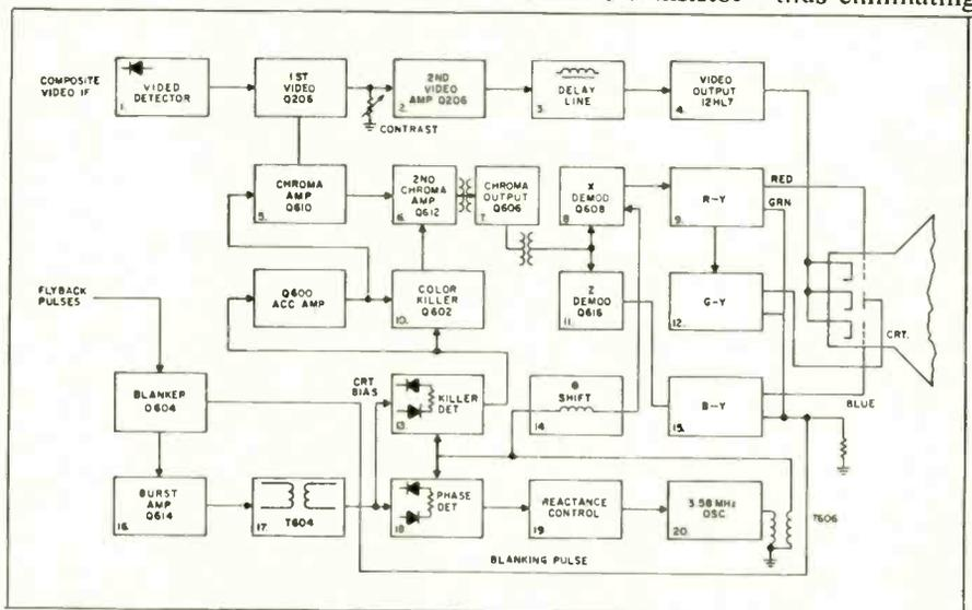
Fig. 1—Block diagram of video and chroma circuits.
