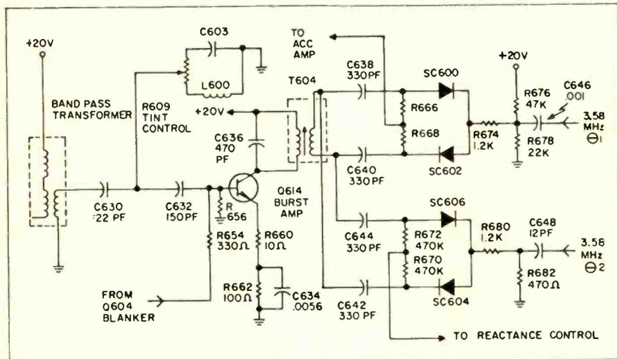
Fig. 7—Burst Amplifier and Phase Detectors.
