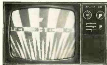
Fig. 12—With horizontal oscillator disconnected from horizontal-output circuit, injecting analyst's horizontal-grid-drive signal at grid of output tube results in a test pattern containing no beat signal.
