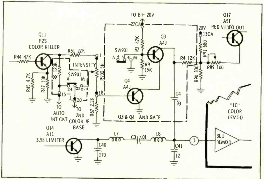
Fig. 2—Simplified diagram of the hue and tint circuit showing the solid-state switch which operates as a "AND GATE." Courtesy of Motorola Inc.
