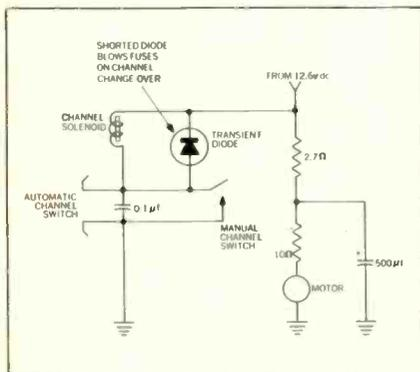
Fig. 5—A shorted transient diode across the solenoid will blow fuses during a channel change.
