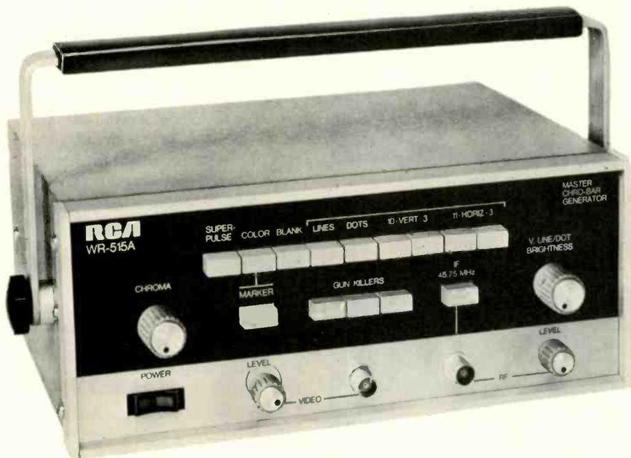
RCA's Type WR-515A Master Chro-Bar IC Color Bar Generator/Signalyst. For more details, circle 900 on the Reader Service Card.
