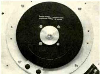
Fig. 17—Four screws secure the position-detector rotor to the magnet rotor.
