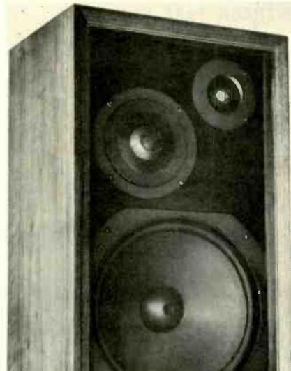
hemispheric dome tweeter. Reportedly the woofer cones are mold-shaped to produce optimum absorption characteristics. Specifications include: Frequency range—30Hz to 20kHz; maximum power handling capacity—60w; minimum amplifier power—10w rms per channel; impedance—8Ω; woofer free-air resonance frequency—19Hz; level controls—high and mid-range in five steps each ±2dB; and crossover
