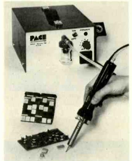
supply. Controls on the front panel of the power source permit controlling the temperature to any desired level up to 1000°F. Solder joints are melted with a coaxial tubular tip. Then, the foot pedal, connected directly to the power source, can be depressed to provide an instantaneous continuous vacuum. The continuous vacuum removes the molten solder and then cools the solder joint area to prevent the reswetting of component leads to hole and pad areas. Price: \$249.00. Pace Inc.
