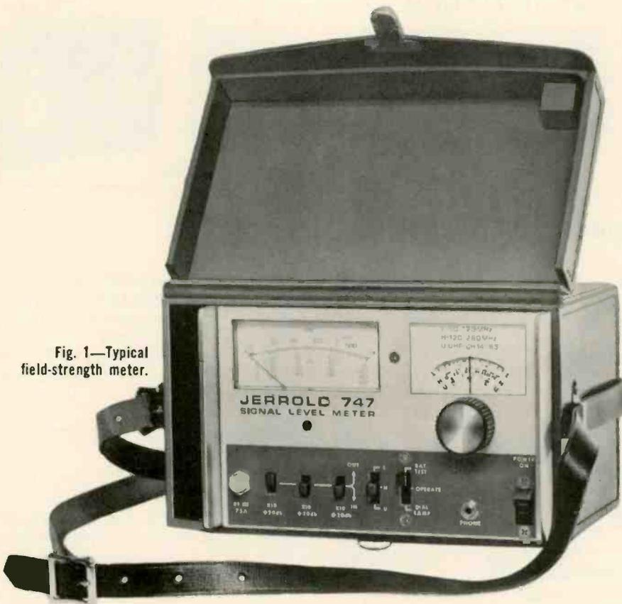
Fig. 1—Typical field-strength meter.
