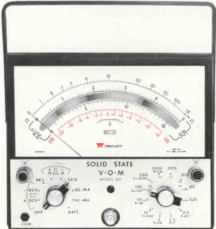
1. Lower power ohms — 8 ranges with 35 mV power source and 1 ohm center scale.
