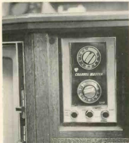
With the door open, the CHANNEL SELECTOR knobs, ON/OFF switch, VOLUME, AFT and AUTOMATIC TINT controls are exposed. Also, shown are the slide type COLOR and TINT controls.
