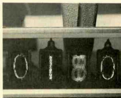
Fig. 16—The loading effect of the Logic Clip, when excess voltages are applied, causes all numerals in the neon indicator lamp to glow simultaneously.
