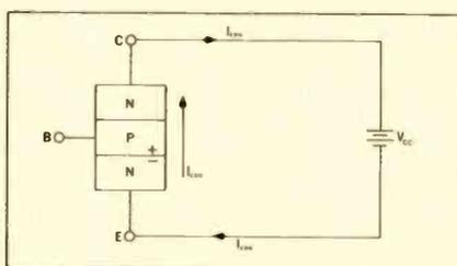
Fig. 5—Leakage current tends to forward bias the E-B junction.
