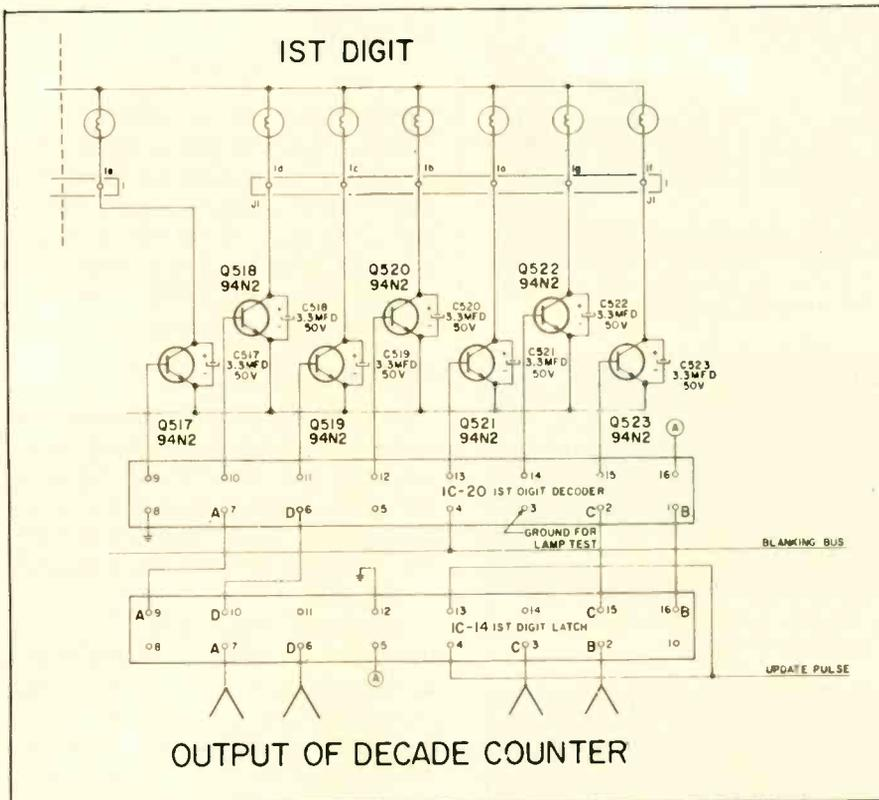
Fig. 20—Partial schematic showing connections between Digital-Latch IC, Digital-Decoder IC and indicator lamp circuits in Magnavox's 1500 DTI Receiver. Courtesy of Magnavox.
