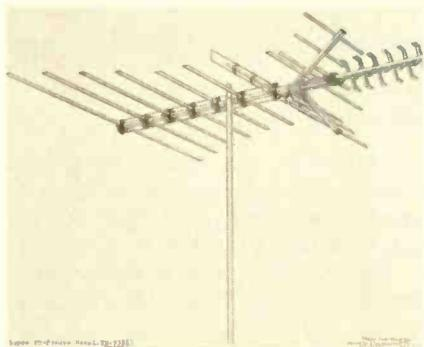
made of heavy gauge aluminum with a golden armor coating to minimize corrosion, they are easy to mount because they employ positive locking fold out elements, a single U-Bolt mast locking assembly and center-of-gravity balance. An especially important feature of the antennas is that they are electrically grounded to the mast. This provides a safety factor and makes it easier for technicians to test download continuity. Jerrold Electronics Corp.
