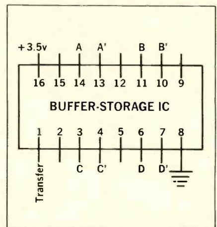
Fig. 3—Terminals of the Buffer-Storage IC as viewed from the top.
