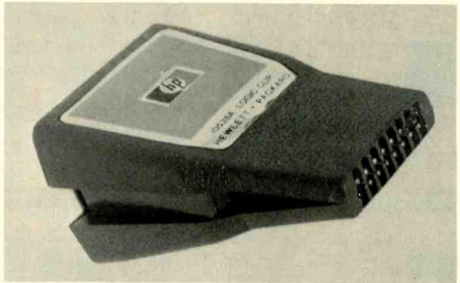
Fig. 1—Hewlett Packard's 10528A Logic Clip, used for observing digital-signal conditions present in the integrated circuits.
