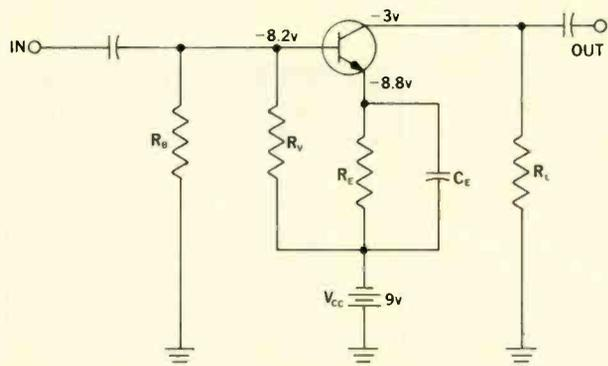
Fig. 13—Inverted configuration for an NPN transistor.
