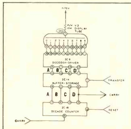
Fig. 2—Partial schematic showing connections between Decade Counter IC, Buffer-Storage IC, Decoder-Driver IC and display tube in Heath's IB101 Frequency Counter. Courtesy of Heath Co.
