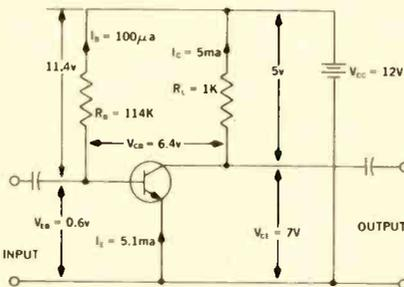
Fig. 2—Voltage distribution in the circuit.
