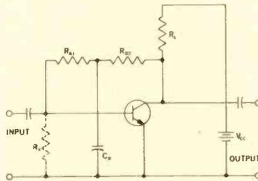
Fig. 8—Self-biasing circuit with  $C_e$  preventing ac negative feedback.
