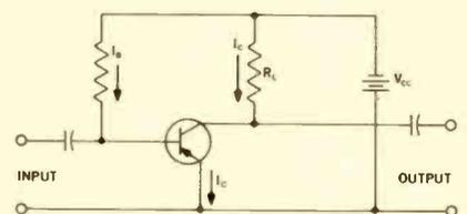
Fig. 3—PNP transistor biasing.
