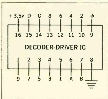
Fig. 14—Terminals of the Decoder-Driver IC as viewed from the top.
