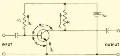
Fig. 1—Biasing an NPN transistor with a single battery.
