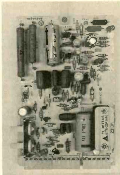
The "V" Board contains the vertical oscillator and drive circuits.
