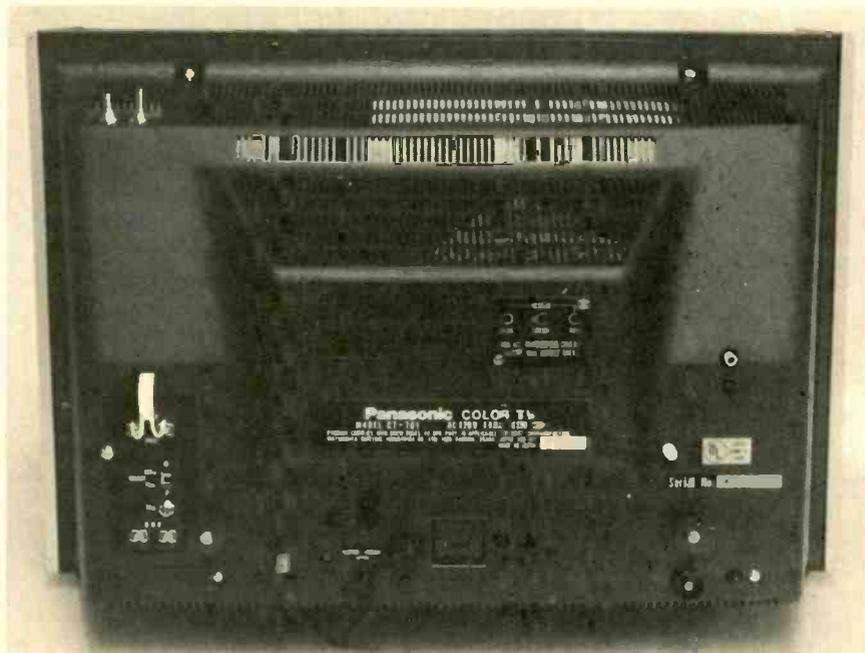
The back cover, sides and top of the cabinet are one piece. When removed, the complete chassis is exposed for servicing.
