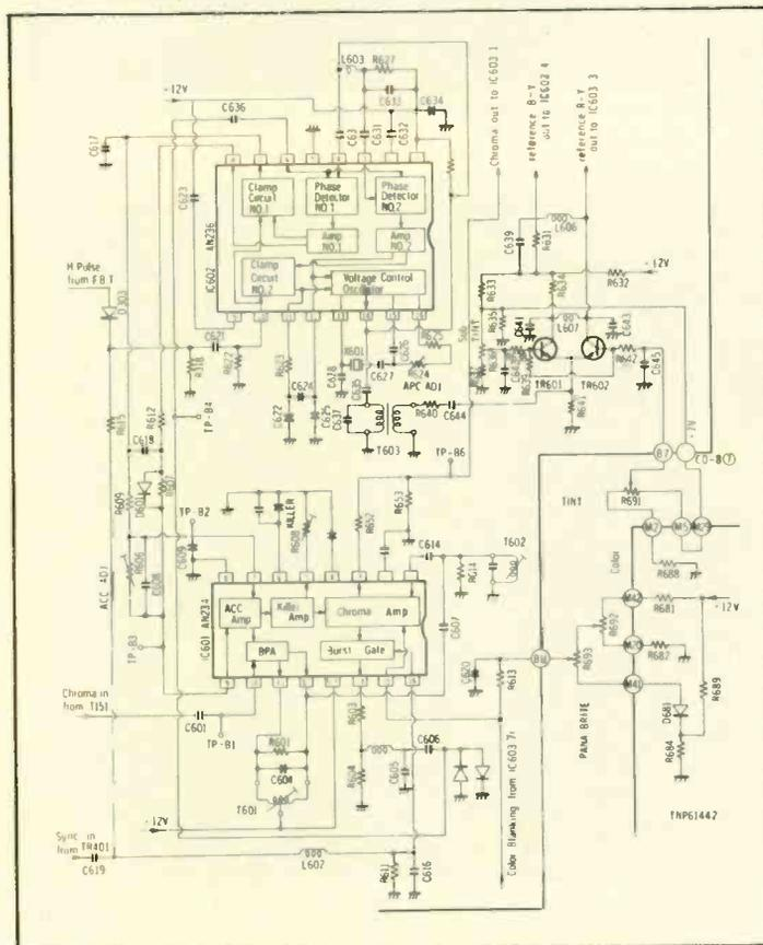
A simplified schematic of the color process and color oscillator circuits. Courtesy of Panasonic.
