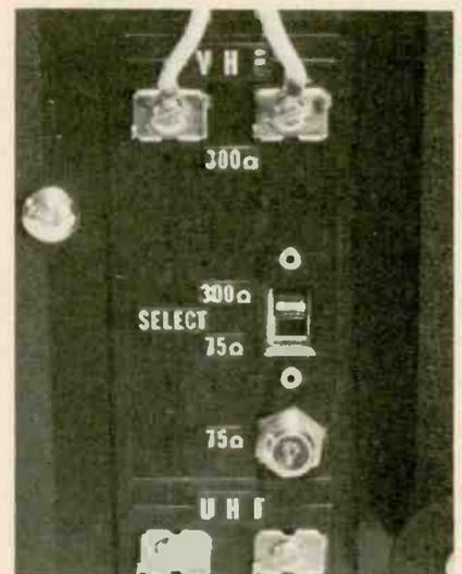
The antenna terminal board includes both 300Ω twin-lead and 75Ω coaxial input connectors with a slide switch for antenna selection.
