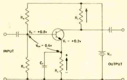
Fig. 6—Emitter stabilizing resistor prevents thermal runaway.
