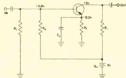
Fig. 12—Conventional configuration for an NPN transistor.
