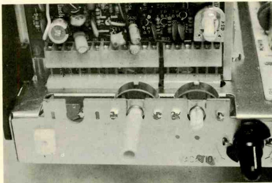
The modules employ pin type edge connectors and are mounted vertically in rigid metal guides.
