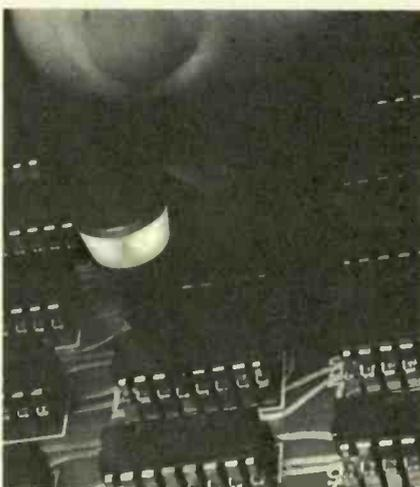
Fig. 18—Light is emitted by the Logic Probe when IC terminal voltages are greater than +1.5v.
