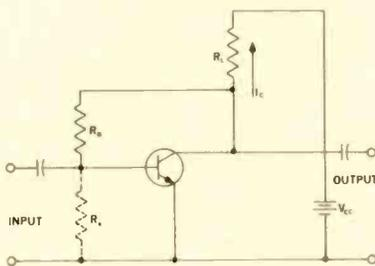
Fig. 7—Self-biasing method.
