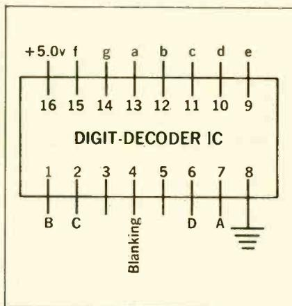
Fig. 21—Terminals of the Digital-Decoder IC as viewed from the top.
