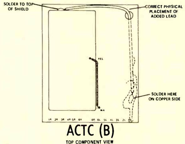
ACTC module (B) (Part No. 69-1000), between the top of the shield and terminal (1L) should correct the problem.
