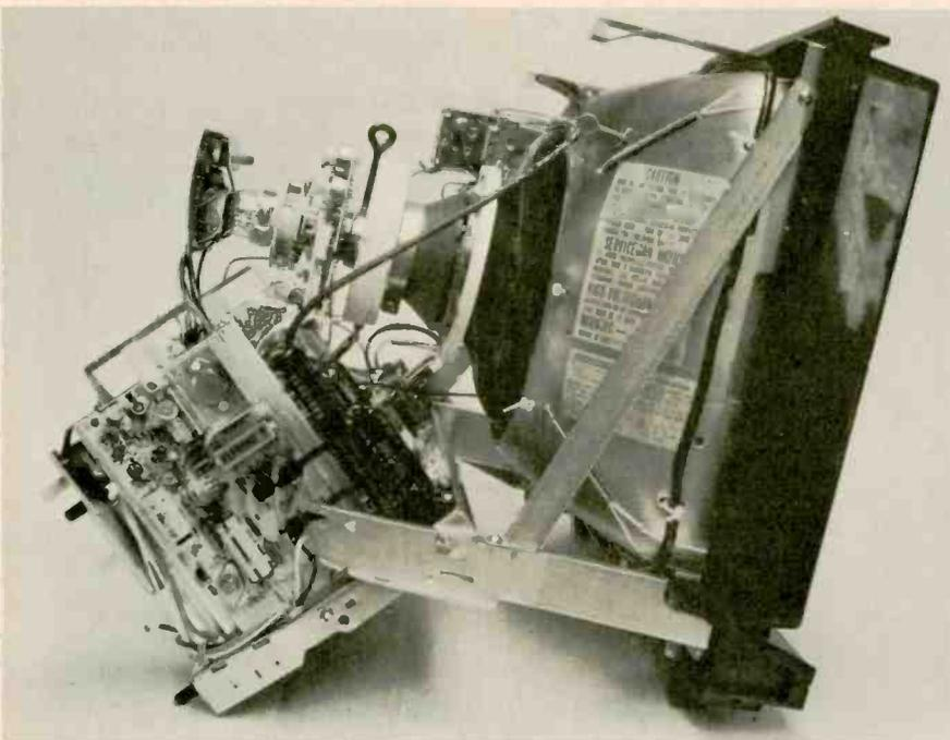
Tilting of the chassis for easier component removal, if required, is accomplished by loosening two screws on each side of the chassis.
