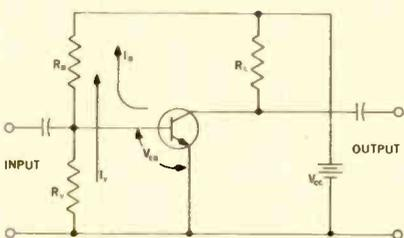
Fig. 4—Stabilizing resistor  $R_V$  forms a voltage divider with  $R_B$ .
