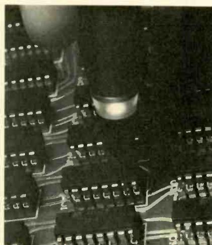
Fig. 19—Rapidly pulsating digital signals cause the Logic Probe light to either appear to flicker or glow less brightly, depending upon the pulse rate.
