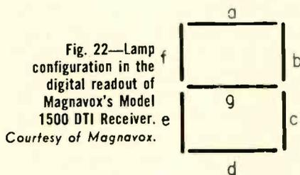
Fig. 22—Lamp configuration in the digital readout of Magnavox's Model 1500 DTI Receiver. Courtesy of Magnavox.
