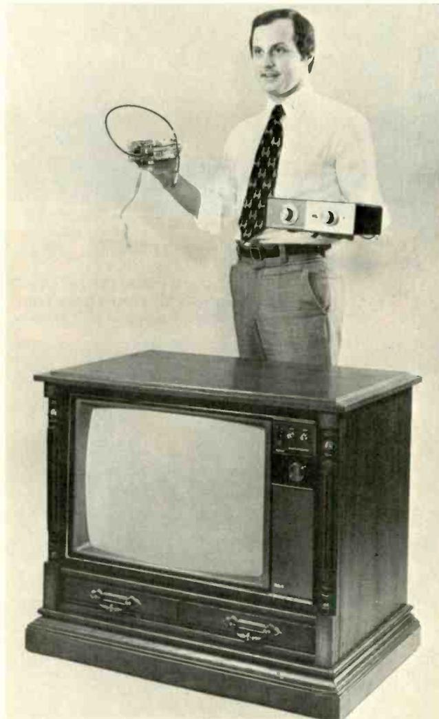
A compact, solid-state electronics unit (left) is now incorporated into the new ready-for-cable TV sets to replace the separate 24-channel selector (right) previously required for cable TV systems. RCA's new line of 25-in. (measured diagonally) color-TV features wireless remote control, AFT, and instant picture—all features previously unavailable with cable reception. *Courtesy of RCA Corp.*
