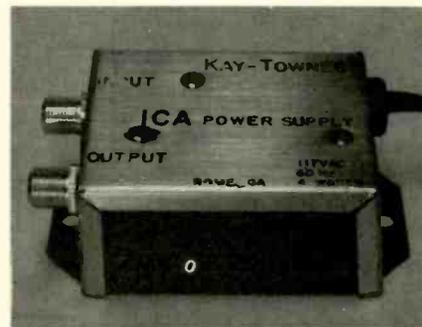
The ICA Power Supply supplies the voltage needed for the antenna amplifier through the coaxial lead.
