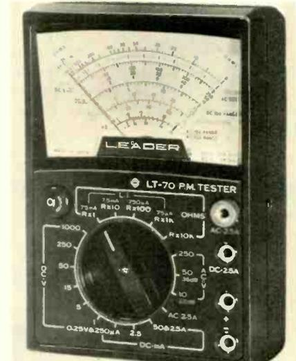
diode and transistor quality. Its sensitivity is reportedly 20K/v dc and 8K/v ac, with resistances rated up to 40M. Other specifications include the following: nine current ranges; DC—75 $\mu$ a to 2.5a and AC—2.5a. Voltage ranges from 0.25v to 1kv DC (10 steps) and 10v to 250v ac (3 steps). The output in the 10v range of -20 to +22dB, ac and in the 50v range
