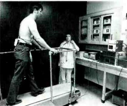
Fig. 5—An exercise ECG installation in which a patient's ECG is radioed by a VHF or UHF FM transmitter to a special receiver on the counter.
