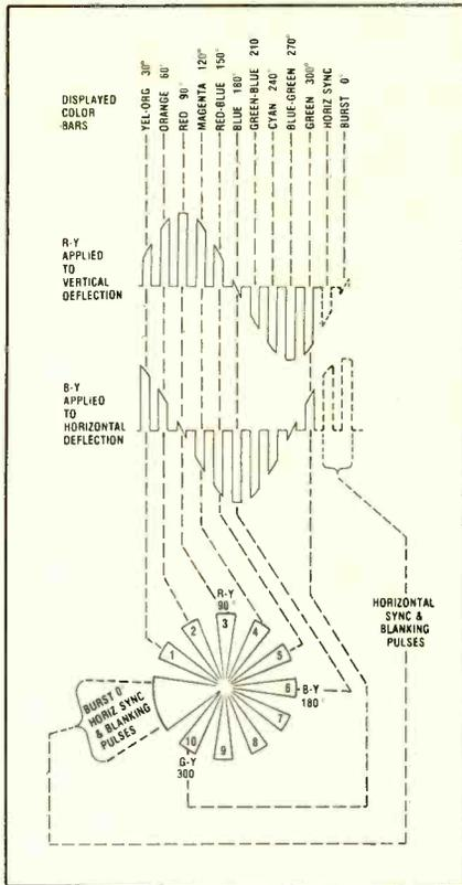
Fig. 2—An ideal chroma vector pattern and the R-Y and B-Y signals which would produce it. Dotted lines illustrate the corresponding relationships between the ten color bars displayed on the screen, the ten pulses of the R-Y and B-Y signals, and the ten petals of the vector pattern.
