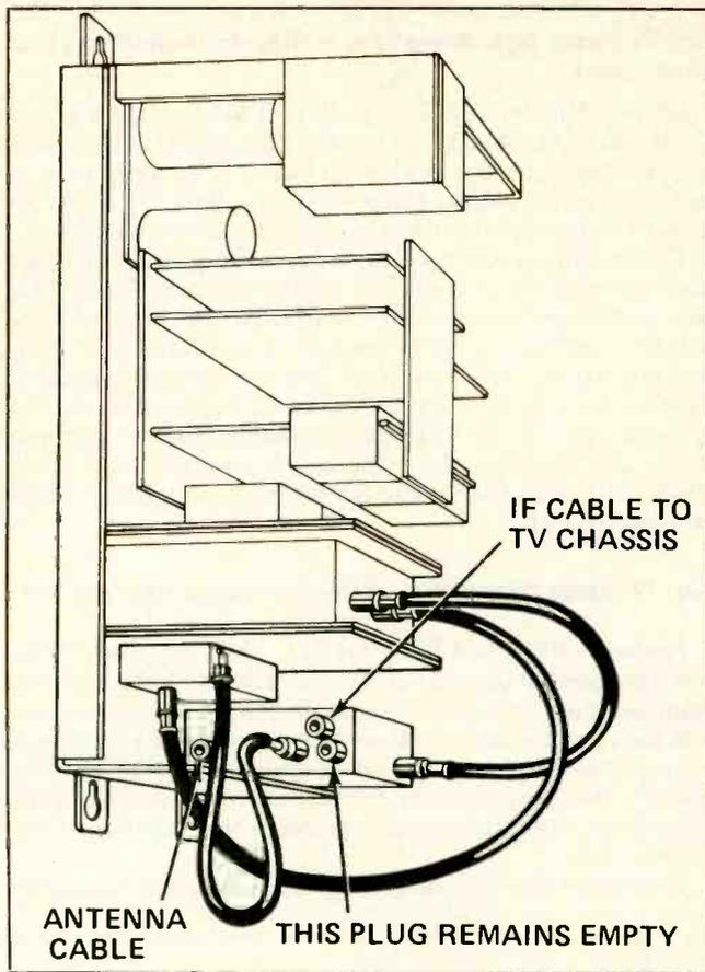
VHF tuner. As shown in the illustration, two coax cables connect to the VHF tuner. One is the antenna cable and the other is the IF cable to the TV chassis. Notice that one of the plugs remains empty. If the IF cable is connected to the empty plug, the results will be a snowy picture or no picture. When installing a replacement STAR Tuning Assembly, be sure to connect the IF cable to the correct plug. ■
