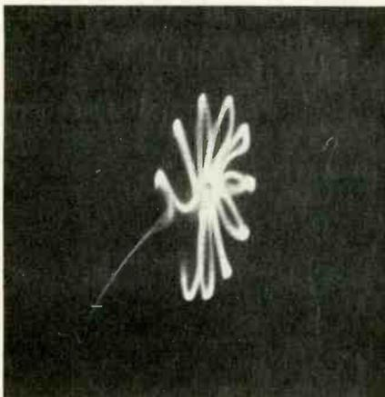
Fig. 5—Insufficient amplitude of the B-Y signal caused the vertically elliptical shape of this normally round vector pattern.
