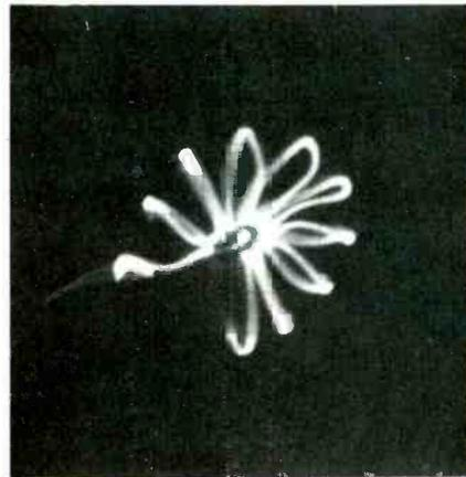
Fig. 9—Excessively curved and overlapped petals, as illustrated here, are usually caused by reduced bandwidth of the chroma bandpass amplifier.
