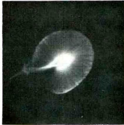
Fig. 8—An cut-of-sync chroma reference oscillator causes rapid rotation of the vector pattern.
