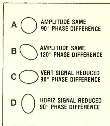
Fig. 1—Representations of the common Lissajous patterns produced by a scope when two different sinusoidal signals with the same frequency but with different phases and amplitudes are applied to the horizontal and vertical deflection plates.
