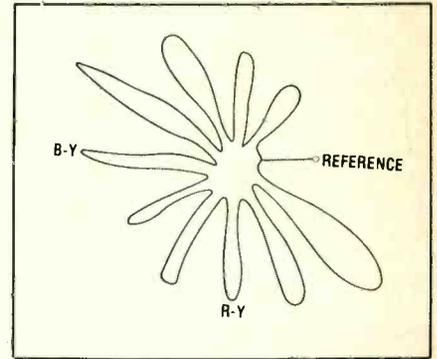
Fig. 4—Representation of the actual vector pattern produced by a color chassis in which the phase difference between the red and bluomodulators is 116 degrees and the R-Y and B-Y signals are obtained from the cathode connections of the picture tube.
