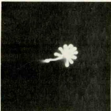
Fig. 7—Insufficient amplitude of both the R-Y and B-Y signals caused this abnormally small vector pattern.
