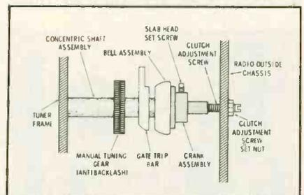
Fig. 5—The clutch/anti-backlash gear assembly. (From "Automobile Electronics Servicing Guide", by permission of Howard W. Sams Co.)
