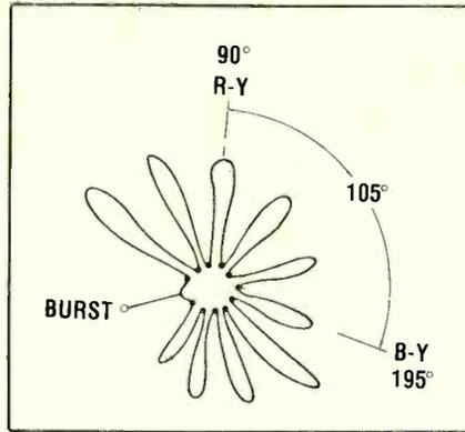
Fig. 3—Representation of the actual vector pattern produced by a color chassis in which the phase difference between the red and bluomodulators is 116 degrees and the R-Y and B-Y signals are obtained from the cathode connections of the picture tube.
