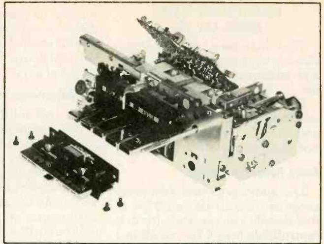
Fig. 2—Partially disassembled signal-seeking car radio. (Courtesy of Delco Electronics.)
