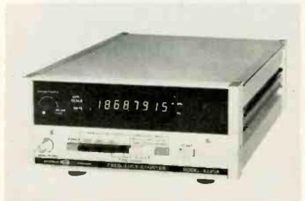
digit readings of frequency inputs to 50 MHz. For measuring low frequency tone signals the unique phase lock/multiplier circuit permits the counter to resolve 0.001 Hz in one second and display the measurement directly. This feature eliminates the long delay of 100 or 1000 second time bases, or the often confusing alternate technique of making a period mea-
