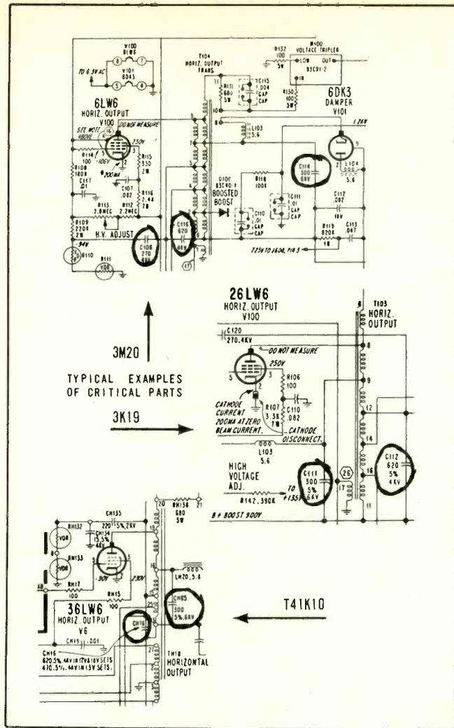
ral replacement parts. Refer to the service manual for the model being serviced to be sure that you get the correct replacement part.
