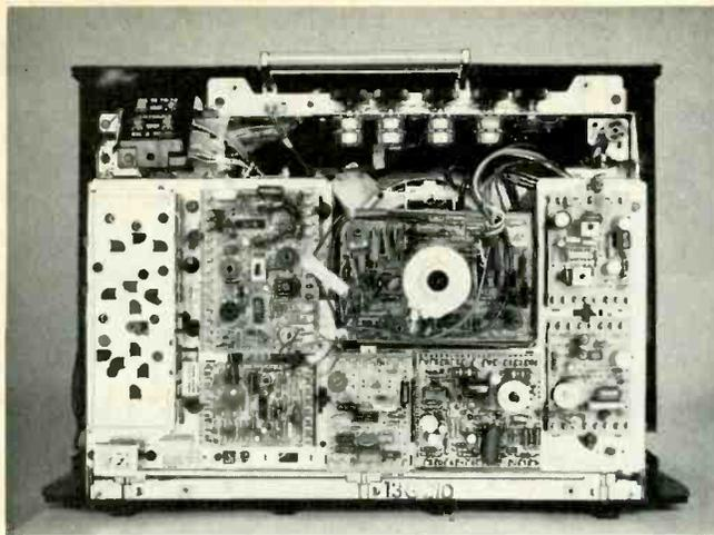
Fig. 1—Rear view of Zenith's new 13-inch (diagonal) TV set which employs a new modular, solid-state 13GC10 color chassis and a new in-line, 110-degree picture tube.
