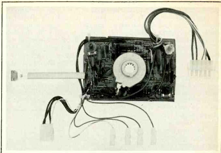
Fig. 5—The new 9-121 Video Output Module, which makes possible a simplified b/w tracking procedure, is mounted on the picture tube socket.
