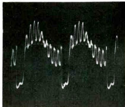
Fig. 10—Abnormal curvature of the baseline of the R-Y and/or B-Y signals, as illustrated here in an R-Y signal, causes the normally round center of the vector pattern to become elliptically shaped.
