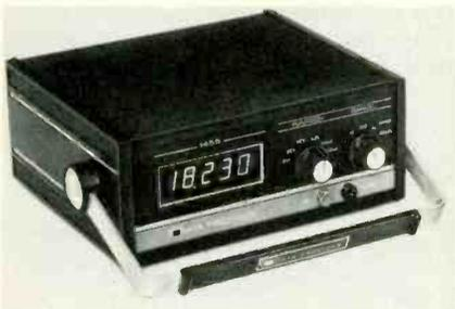
tion is 500 V DC or peak AC with CMRR of 120 dB at DC, greater than 100 dB at 50 and 60 Hz. The unit is equipped with its own internal NiCd battery module and recharger. It operates as a conventional bench-mounting laboratory DMM. Operated continuously on AC line power, the batteries remain on charge whether the instrument is off or on. When not line connected, it automatically operates from its batteries for at least six hours. The multimeter measures 8½ inches wide by 3½ inches high by 7½
