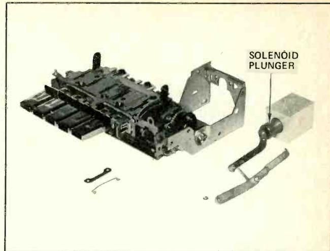
Fig. 3—Back view of signal-seeking car radio with PTM coil housing raised to expose the slide subassembly beneath it. (Courtesy of Delco Electronics.)
