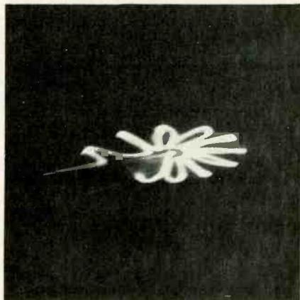
Fig. 6—Insufficient amplitude of the R-Y signal caused the horizontally elliptical shape of this normally round vector pattern.
