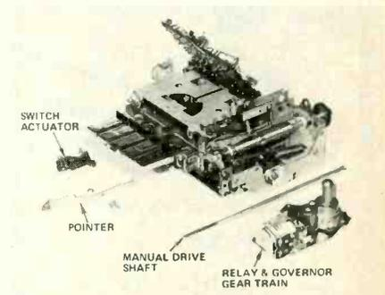
Fig. 8—Exposed view of rack and PTM drive assembly and other principal parts and mechanisms.
