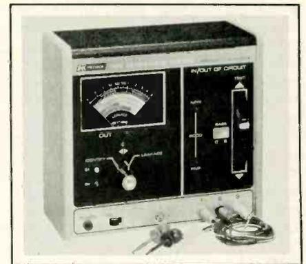
ment. The base (or gate) lead is automatically identified by the color in the small window on the front panel; collector and emitter leads are color identifiable in the same window. With one flip of a lever switch, you can determine if any PNP or NPN device is good, and you also get automatic set-up of lead connections for further testing. The unit measures 8 inches by 7 inches by 3 1/2 inches and is priced at \$150.
