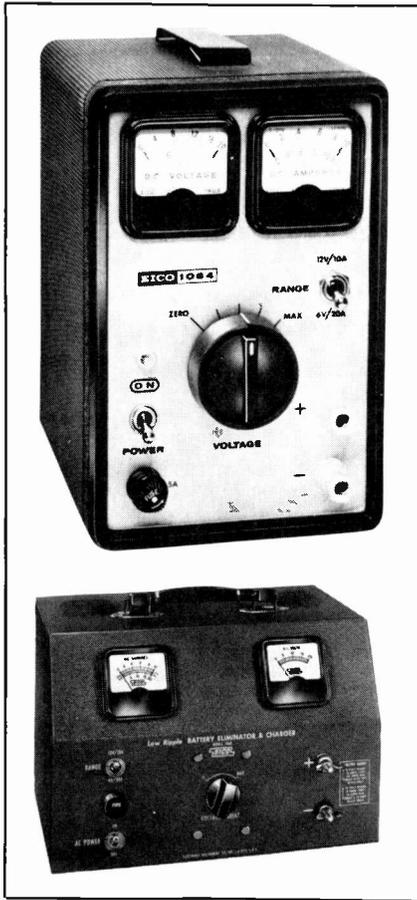
Fig. 2—Examples of typical heavy- and medium-duty bench power supplies. A) Medium duty. B) Heavy duty.
