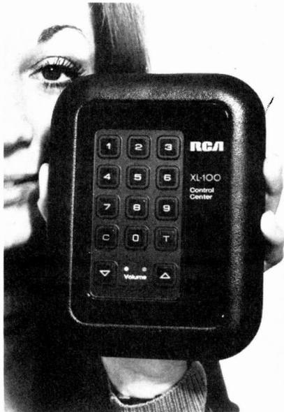
Fig. 7—The new Direct Address System control center is operated through a push-button array resembling that of a push-button pocket calculator keyboard.
