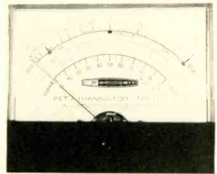
Fig. 9—Meter of IT-121. Top scale is direct-reading scale, with corresponding collector current/beta multiplication indicators below it.
