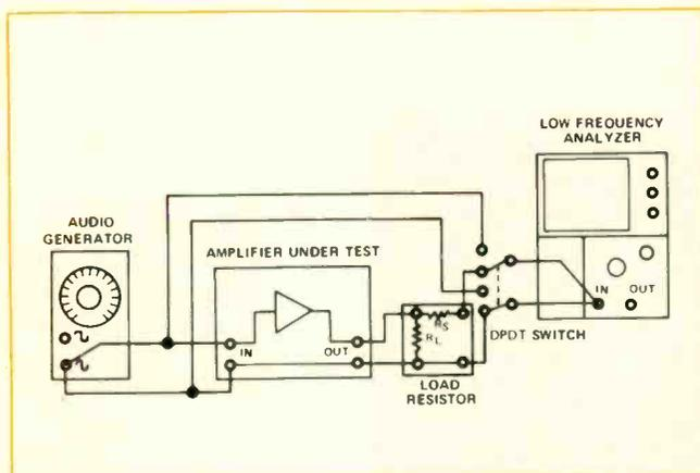
Fig. 18—This is the spectrum analyzer setup for measuring amplifier sensitivity.
