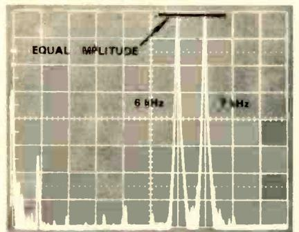
Fig. 8—A spectrum analyzer display showing correct signal settings and some responses, using the CCIF method of test.
