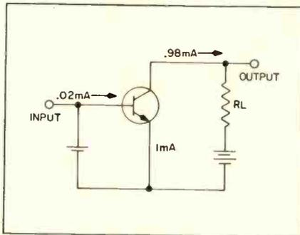
Fig. 2—Common-emitter circuit configuration. Emitter is common to both the input (base-emitter) and the output (collector-emitter) circuit.
