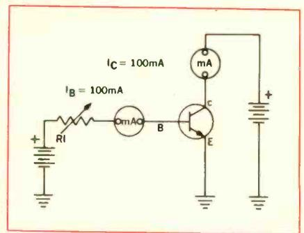
Fig. 3—Common-emitter circuit which, along with chart in Fig. 4, is used to illustrate how collector current level affects beta measurement.
