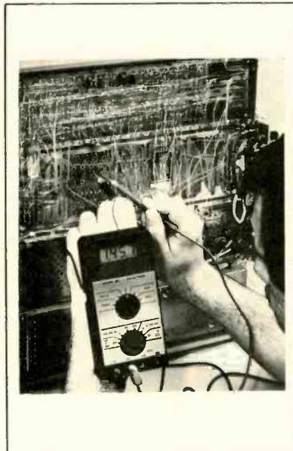
curacy of readings on DCV is 0.1% ± 1 digit. Model 22 features a large .5 inch LCD display, uses standard size disposable batteries and provides overload protection. It will also operate with rechargeable batteries or on AC. Priced at \$234.
