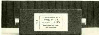
and the transceiver (or amplifier) to suppress undesired radiation by at least 60 dB's. Insertion loss at the operating frequency is less than 0.25 dB. The new filter, which handles up to 500 watts, may be used with AM, SSB, CW, or FM systems. It is said to pass all frequencies up to 30 MHz, but passes no signal beyond 32 MHz. Screwdriver adjustment allows for transceiver/filter match.
