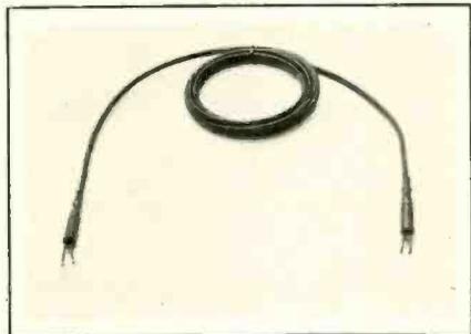
al cable but built inside the cable are multiple distributed resonators to trap 54MHz and 81MHz. The cable is designed to be connected in line between the CB transceiver and the CB antenna. It does not require the use of a jumper cable to make connection with the transceiver. The cable comes in two lengths; a 6-foot size, designed to be connected to an existing CB system, and an 18-foot length, designed to replace the RG coaxial cable commonly used in mobile CB.
