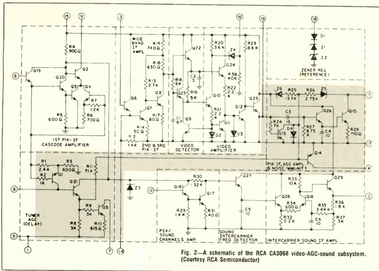
Fig. 2—A schematic of the RCA CA3068 video-AGC-sound subsystem. (Courtesy RCA Semiconductor)
