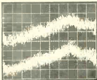
Fig. 15—A dual trace displayed when noise is used as an input to the spectrum display, with the sync selector switch at the 'line' position.
