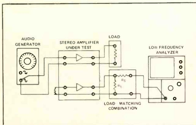
Fig. 20—A spectrum analyzer setup for measuring crosstalk in a stereo system. For quadrophonic systems, all channels, except for the one being measured, should be driven at rated power output.
