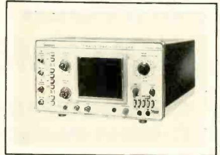
the scope wide bandwidth (DC coupled, DC to 15 MHz; AC coupled, 2 Hz to 15 MHz) with smooth roll-off through 27 MHz. Triggering is internal or external with sync positions for TVV, TVH and VITS. Sensitivity is 5 mV/cm and rise time is 24 nsec. The new scope automatically shifts from "chop" to alternate on faster sweeps. It is able to display Channel A, Channel
