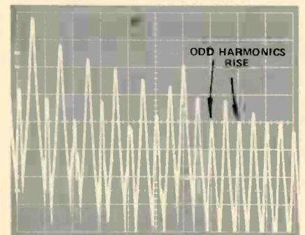
Fig. 14—A spectrum analyzer display of the distorted waveform seen at the bottom of the TIM display shown in Fig. 12.
