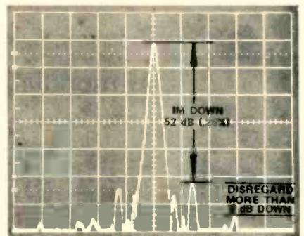
Fig. 9—A spectrum analyzer display that shows indication of SMPTE-type distortion, and its interpretation.
