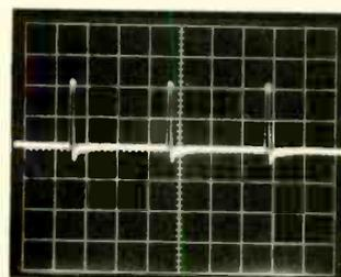
Fig. 6—The waveform produced when an open AGC filter capacitor causes pulses at the horizontal rate to appear on the AGC bus line.
