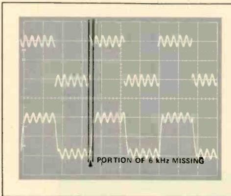
Fig. 12—A Transient Intermodulation Distortion (TIM) display on a spectrum analyzer using dual trace with a regular time base, adjusted for steady waveform.
