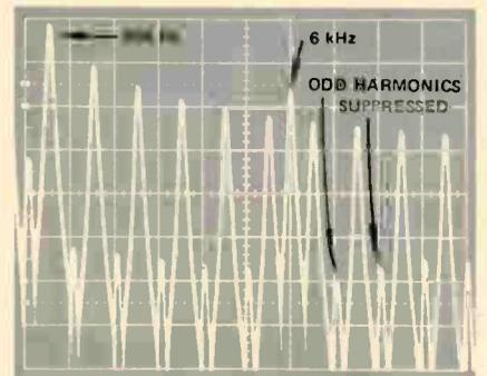
Fig. 13—A spectrum analyzer display of the waveform seen at the top of the TIM display shown in Fig. 12.
