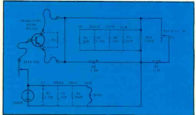
Fig. 11—BETA READDOUT circuit of IT-121. (Same circuit as in Fig. 10 except that meter and R10 are interchanged so that meter is in base circuit of transistor.)
