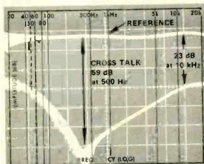
Fig. 21—A spectrum analyzer display of crosstalk measurement.
