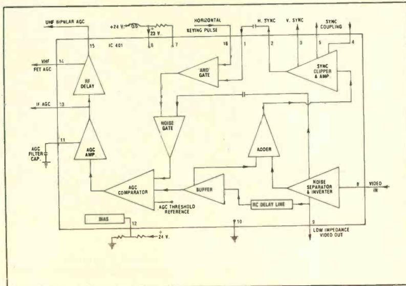
Fig. 4—A simplified diagram of Zenith's IC 401.
