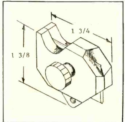
the holder guides the blade around the wire or cable. It is especially useful for coaxial cable, multiconductor cable, Romex cable and high voltage wire with thick-walled insulation. The blade is a standard single edge type and the body is made of ABS plastic. The blade is adjustable for various insulation thicknesses. A tab with a hole in it is included for hanging the guide on a tool board or chain. It lists for \$1.25.
