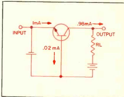
Fig. 1—Common-base circuit configuration. Base is common to both the input (emitter-base) and the output (collector-base) circuit.
