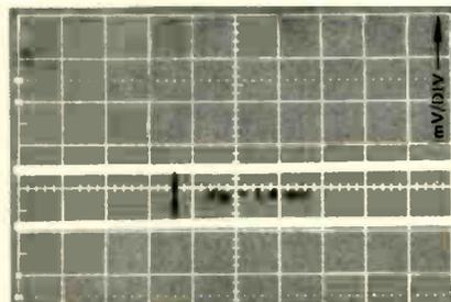
Fig. 17—In the last step of the Signal To Noise Ratio measurement, using the spectrum analyzer, the noise inputs are disconnected, two separated lines appear, and the separation between the lines is measured in volts. This measurement is the  $V_n$ .
