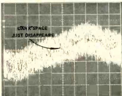
Fig. 16—In the Signal To Noise Ratio measurement, the voltage offset of the spectrum analyzer is adjusted until the dark area between the two traces shown in Fig. 15 just disappears.
