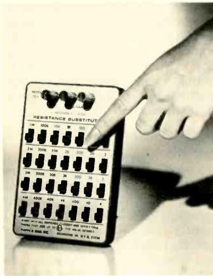
troubleshooting. It is housed in aluminum and features three binding posts, one to ground case. The slide-switch uses one-half watt resistors with 1% tolerance with an accurate range from 1 to 11, 111, 110 ohms, in one-ohm steps. The unit is priced at \$58.
