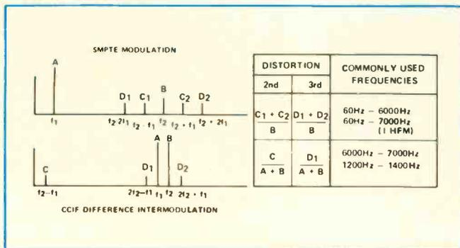
Fig. 5—A comparison of the two standard forms for Intermodulation Distortion (IM) measurement: top line is SMPTE basis for tests, and bottom line is CCIF test basis.
