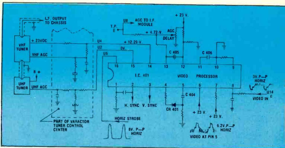
Fig. 5—A schematic diagram of the keyed AGC system used in Zenith's chassis 25GC50.
