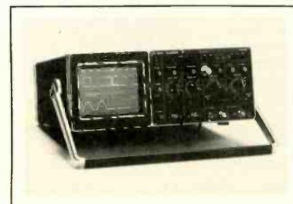
with calibrated delay, Channel A, Channel B, composite and external source. PM3214 is priced at \$1,395.
