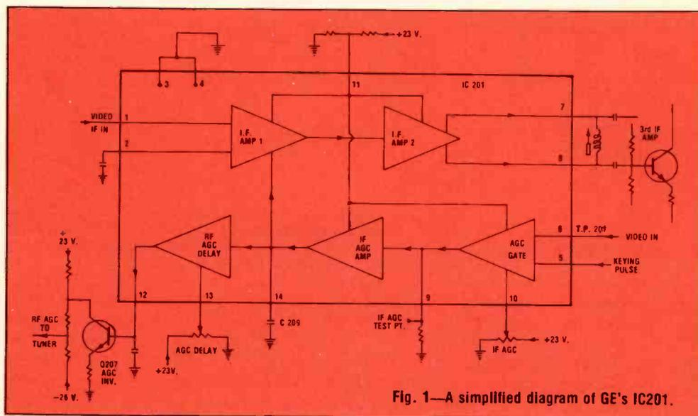
Fig. 1—A simplified diagram of GE's IC201.
