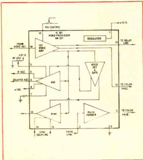
Fig. 3—A simplified diagram of Quasar's IC 301.
