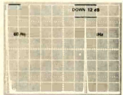
Fig. 7—A spectrum analyzer frequency display, showing relative amplitudes of signal set up for the SMPTE test.
