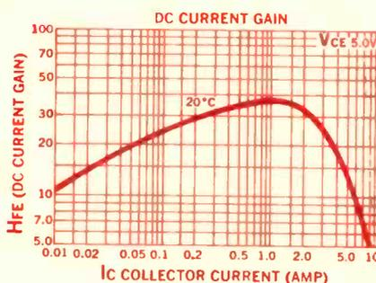
Fig. 4—Chart which illustrates how the DC beta of a bipolar power transistor depends on the collector current at which it is measured.
