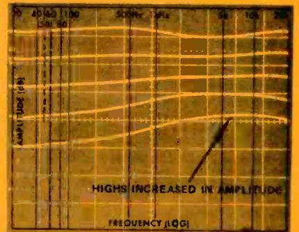
Fig. 4—Display of responses that show the frequency corrective action of a Dolby "B" encoder, when operating at different levels.
