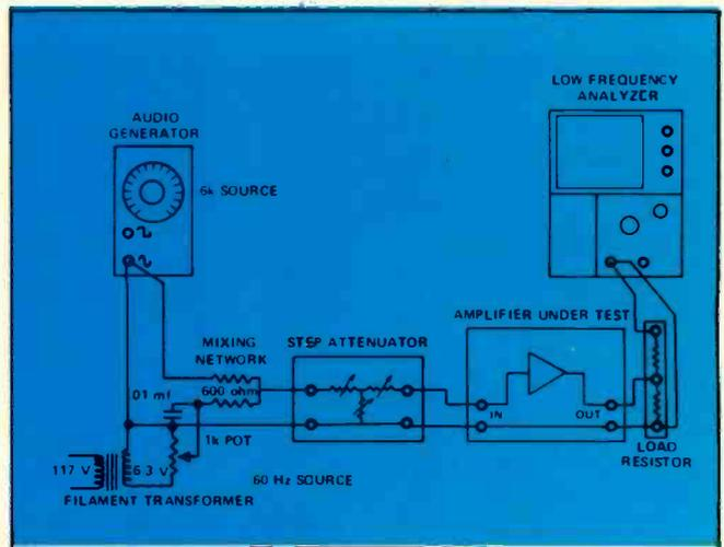
Fig. 6—A simple equipment setup for obtaining SMPTE-type data using a spectrum analyzer. A simple substitution can change this setup for the CCIF-type test.
