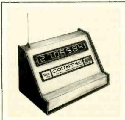
inch-high LED, 7-digit displays with polarizing lens. It is crystal controlled with accuracy up to 40 MHz, and 1 MV sensitivity provides pick-up and display of low power transmission without the need for coax connection. The Count-40 is designed for portable use and may be used for either base or mobile on-the-air frequency verification. It will operate on 12 VDC or 117 VAC, and comes with a 117 volt power adapter.
