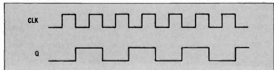
Table 2-Truth table for clocked operation of the J-K flip-flop plus the associated wave forms
