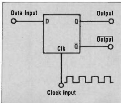
Fig 3—Block diagram of a Type D flip-flop
