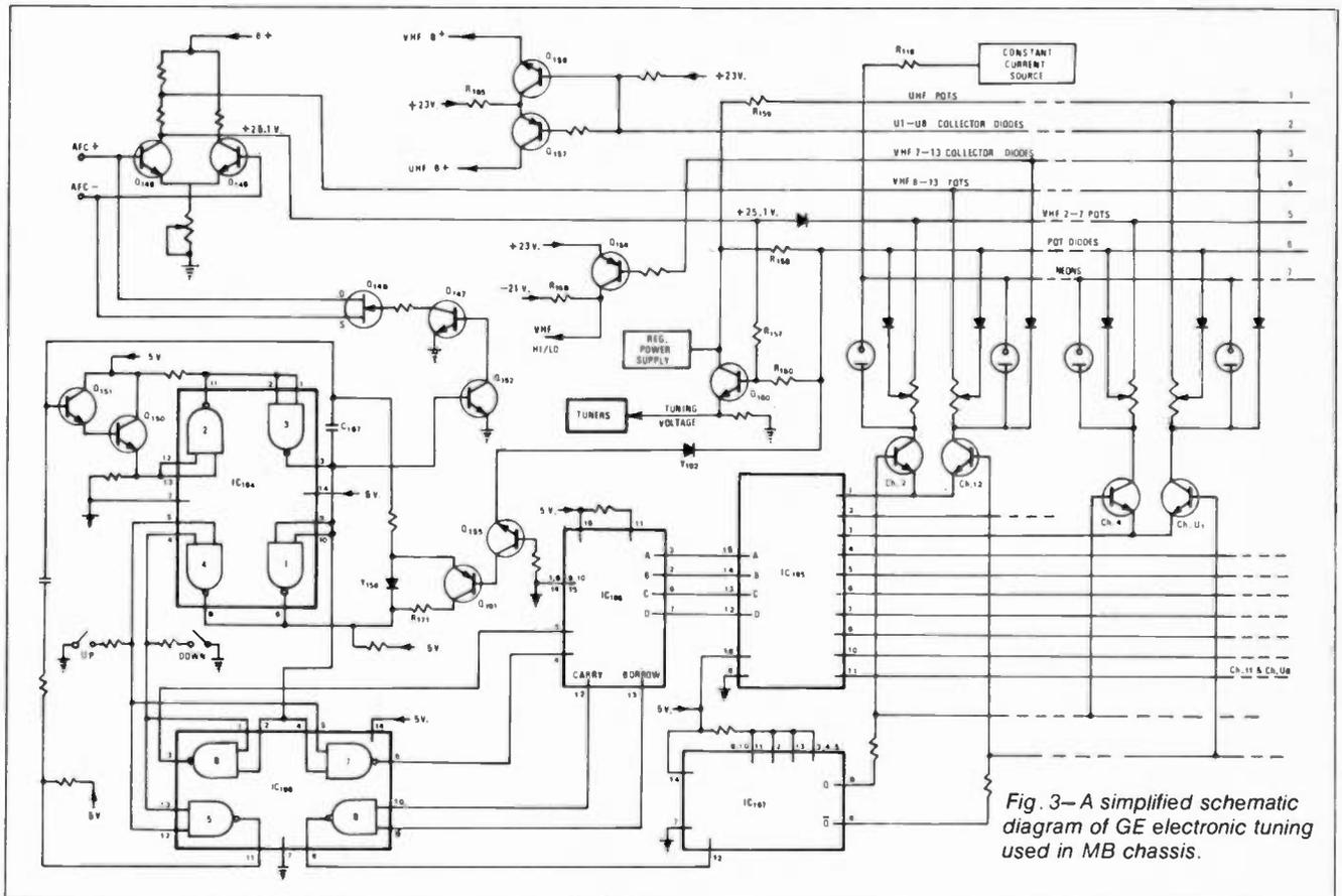
Fig. 3—A simplified schematic diagram of GE electronic tuning used in MB chassis.
