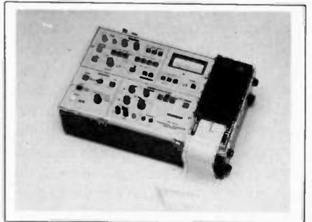
the chart section can also serve as a direct current reader to 10mV/cm. The design format includes: automatic start
