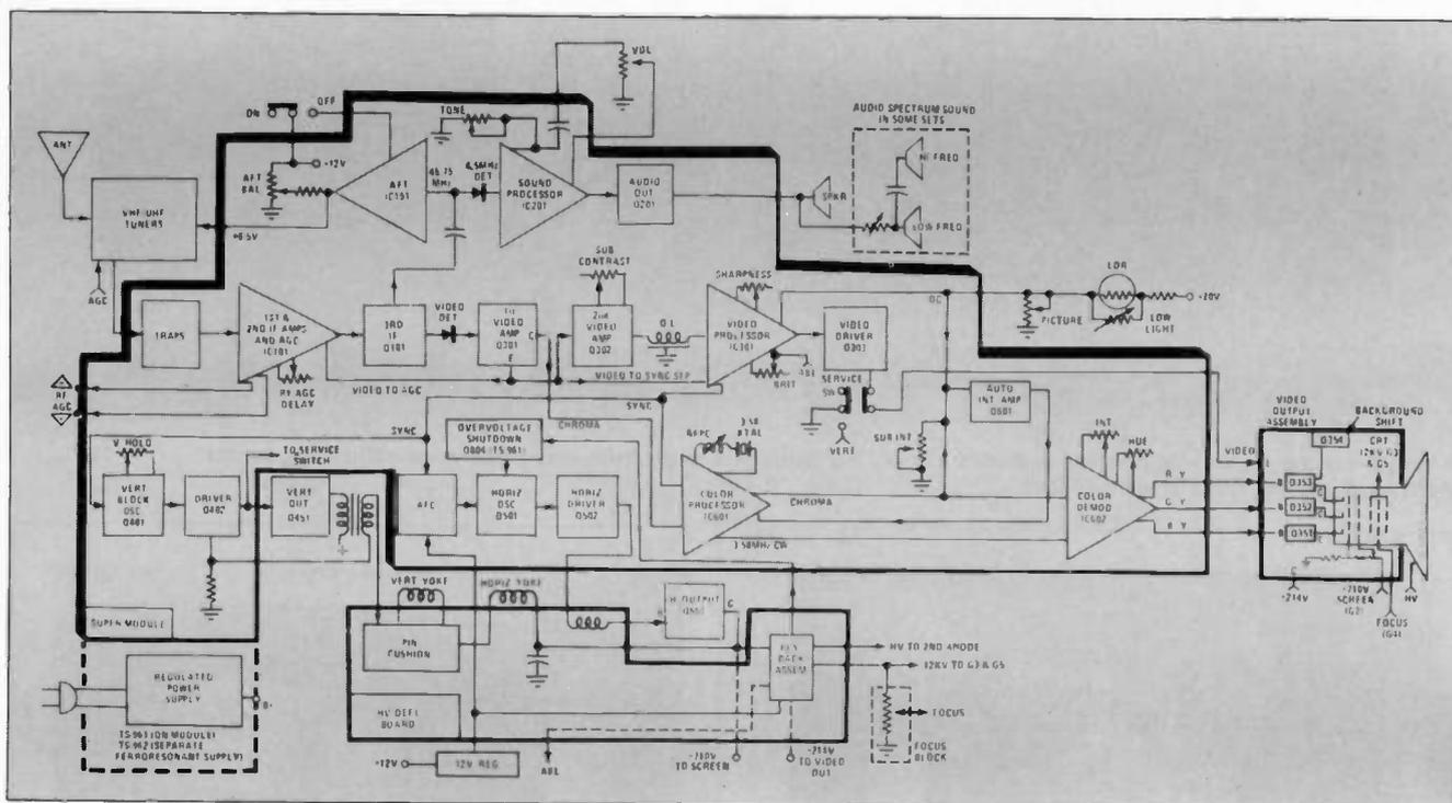
Figure 1 Block diagram of the basic TS-961 and 962 chassis.
