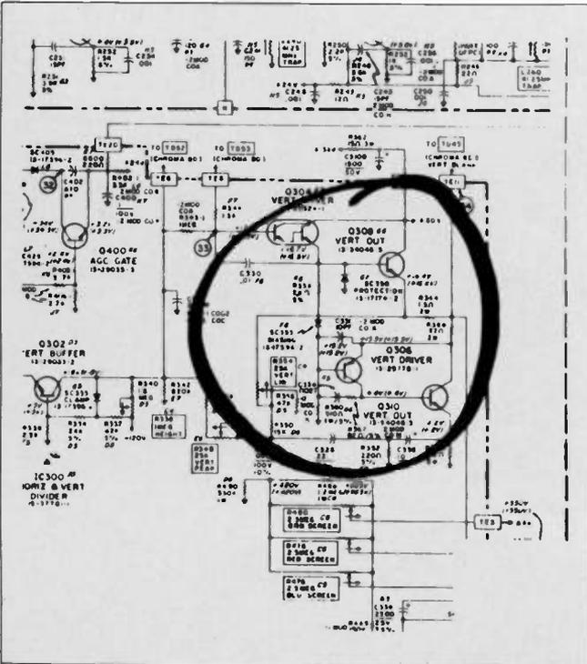
causes bottom of picture to fold up. SC808 is probably breaking down under load. Checks O.K. out of circuit.
