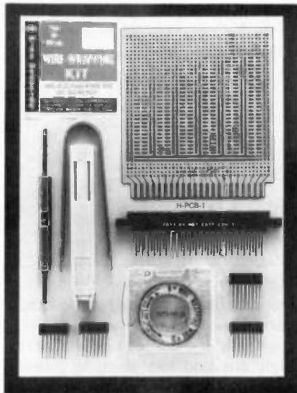
WSU-30, wraps and unwraps 30 AWG wire on .025 square pins and strips the wire. The board features glass coated epoxy laminate construction with solder coated 1 oz. copper pads. Sockets have gold plated terminals and thermoplastic bodies. The wire dispenser includes 50 feet of kynar insulated, silver plated copper wire. The kit is priced at \$25.99.
