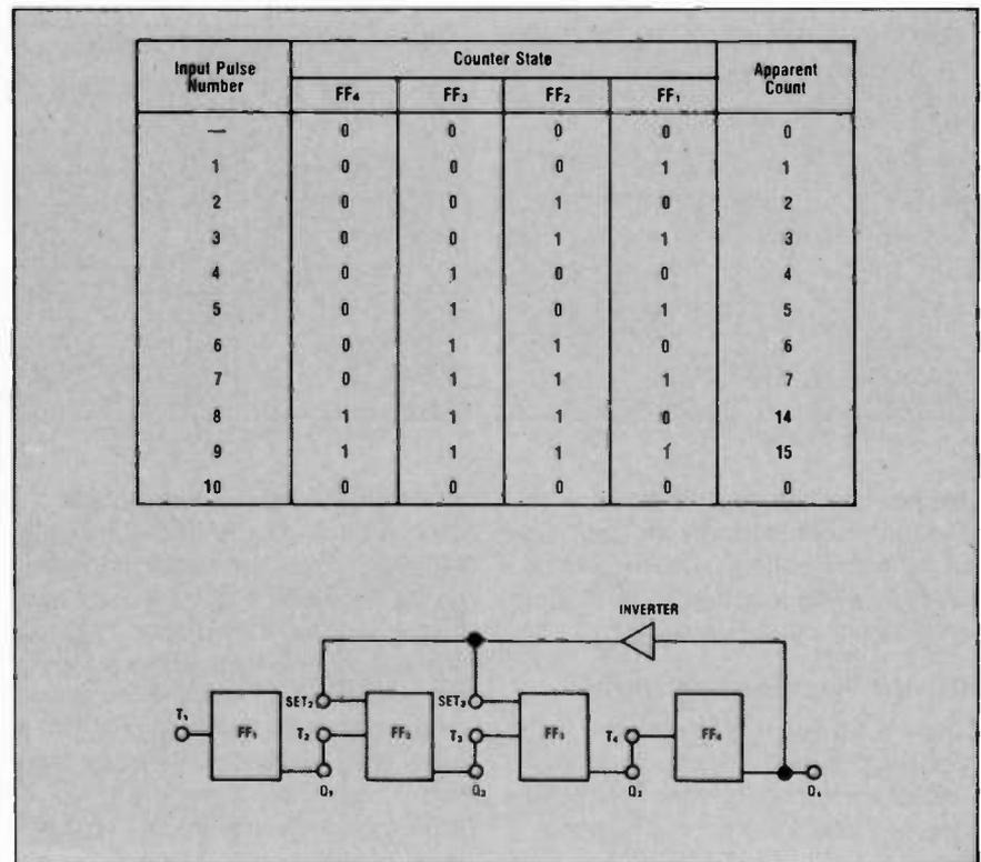
Fig 6-Block diagram of a scale of 10 counter and the table showing its summary of states.
