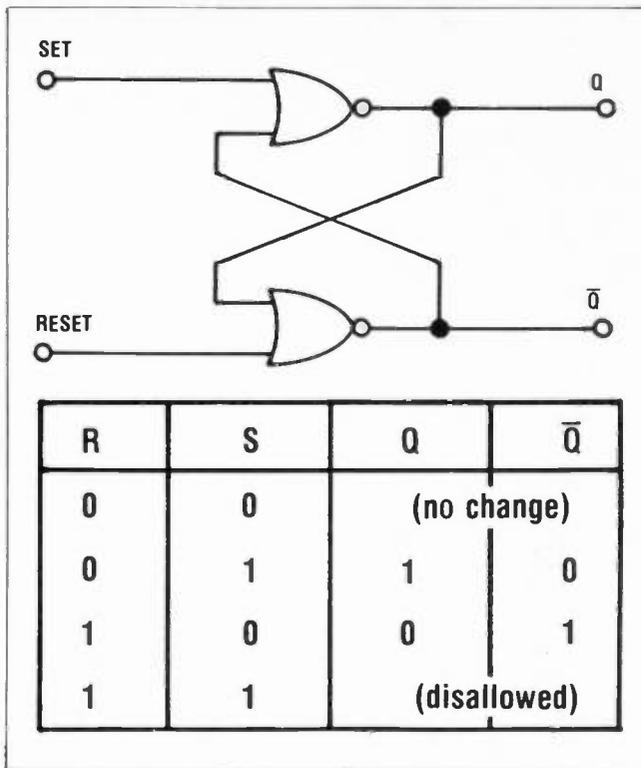
Fig 1—Two input NOR gate RS flip-flop with its associated truth table.
