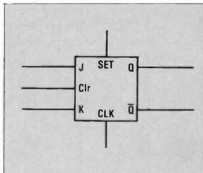
Fig 4—Block diagram of a J-K flip-flop
