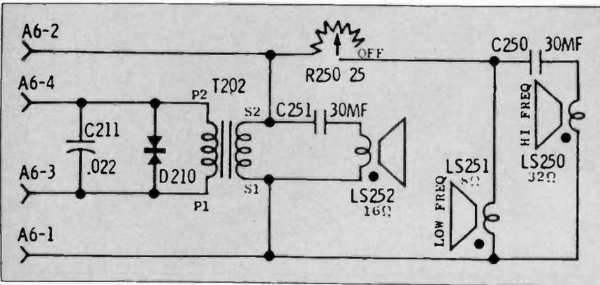
Figure 4 The "Audio Spectrum" sound circuitry
