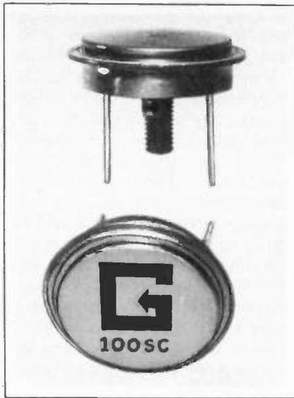
operating voltages. Typical applications are in inverters, switching regulators, power amplifiers and similar high current circuits. Being based on Germanium technology, the GPD 100SC series also is said to give high gain (HFE = 120 typical at -60A Ic, -1V VCE), high efficiency, low input voltage and, above all, very low saturation voltage.
