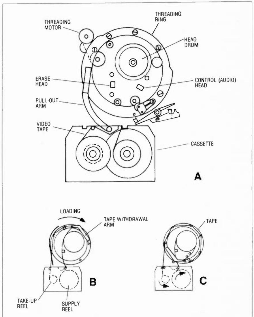
Fig. 3 - Progressive views of the tape threading operation. Figure 3A shows tape position at the start; 3B is a view of the half completed threading operation; and 3C shows the completed threading.
