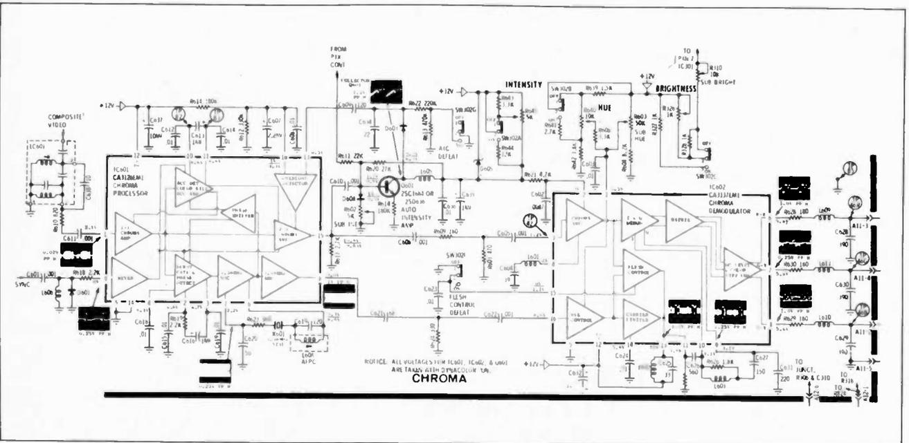
Figure 6 Quasar's redesigned color processing circuitry
