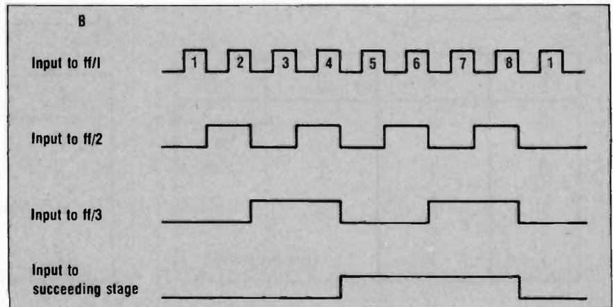
Fig 5-Timing diagram for three plus stage flip-flop circuit showing input and output wave forms.
