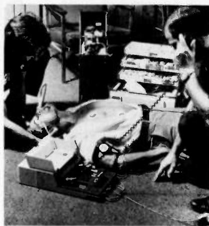
tions where additional RF power is needed, the unit can be tuned to 15 watts with a reduction in operating time.
