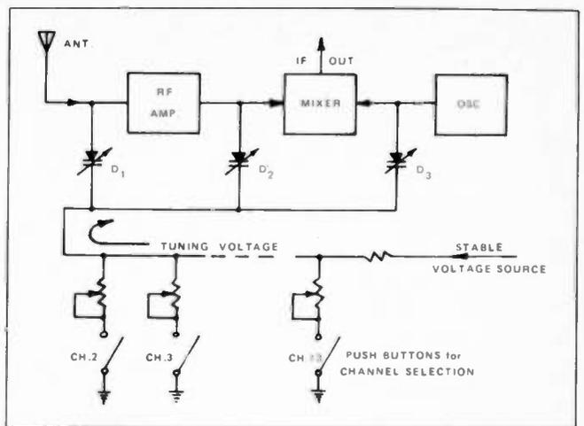
Fig. 2—A basic push-button channel selection system.
