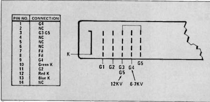
Figure 3 Circuit illustrations of the new 100 degree, tri-potential, in-line gun and pin connections.
