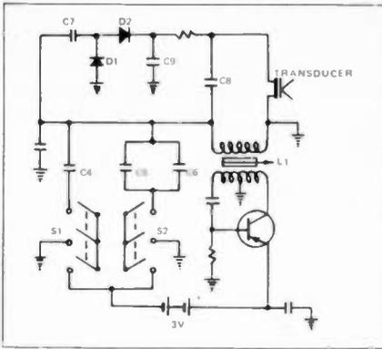
Fig. 4—A GE remote transmitter used with MB chassis.
