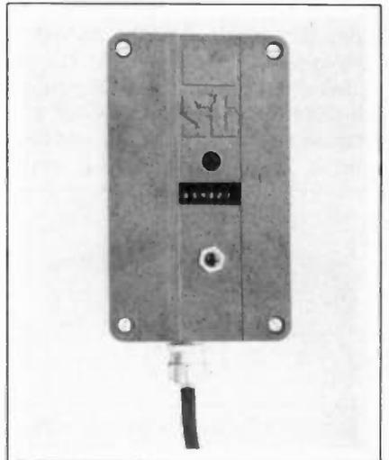
vere industrial counting applications in hostile environments with the LED display, counter circuitry and power supply mounted in an aluminum die case NEMA 4 & 12 rated enclosure. Counting rate is up to 1 MHz and input power sources from 12 VDC to 240 VAC can be accommodated. Standby battery power is also available. Priced at \$85 in single unit quantities.
