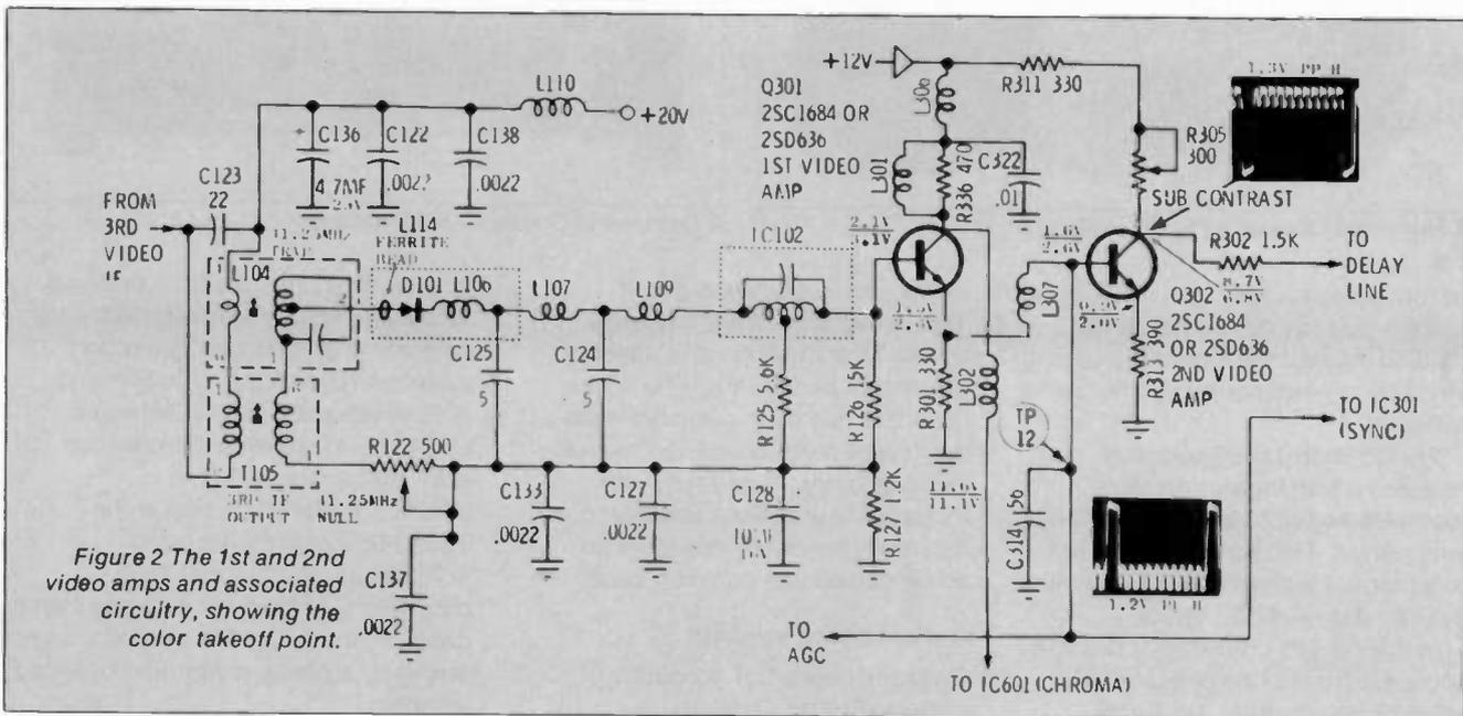
Figure 2 The 1st and 2nd video amps and associated circuitry, showing the color takeoff point.
