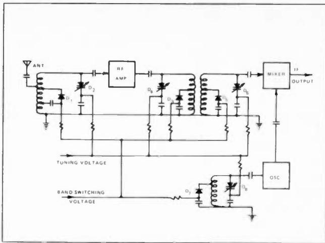
Fig. 1—A simplified schematic diagram of a varactor tuner.
