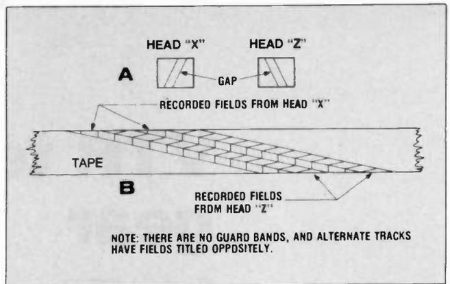
Fig. 2 - Oppositely slanted head gaps (2A) permit recording with oppositely polarized tracks (2B) which in turn reduce crosstalk action without the use of guard bands.
