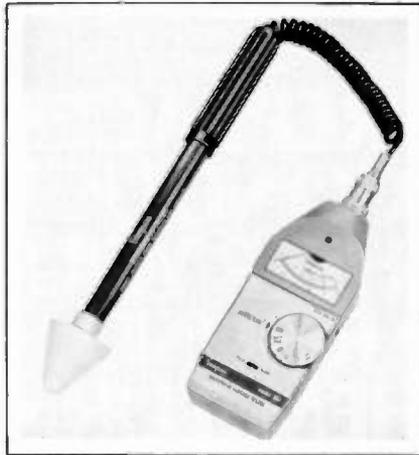
wave ovens, heaters, and dryers. It reportedly meets HEW performance standards and is suitable for service and repair use, as well as production testing. It is a hand held wide-range tester with four ranges of to 100mW/cm<sup>2</sup> with accuracy of  $\pm 1$ dB and a 1.2 second response time, according to specifications. The probe is priced at \$246.75, complete with batteries and manual.
