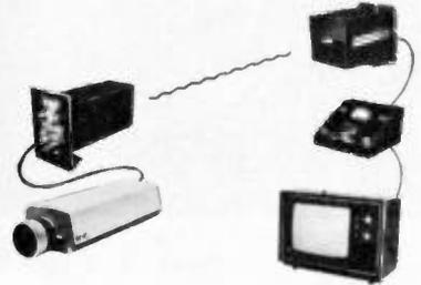
The Video Beam intrusion system transmits a microwave intrusion signal and a high quality television picture simultaneously for a distance of up to one kilometer according to the manufacturer, Visual Methods Inc. The system operates at 10.525 GHz and consists of
