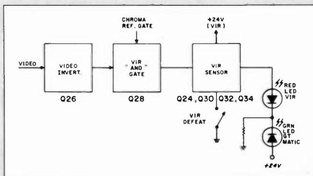
Fig. 5-Simplified schematic VIR sensor.
