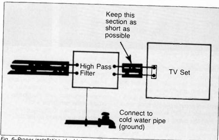
Fig. 6—Proper installation of a high pass filter
