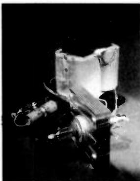
**On the cover:** Our lead feature this month deals with servicing opportunities on microwave ovens. Thus our cover is devoted to key elements of the microwave system; the magnetron (radar) electron tube, and the huge power transformer.
