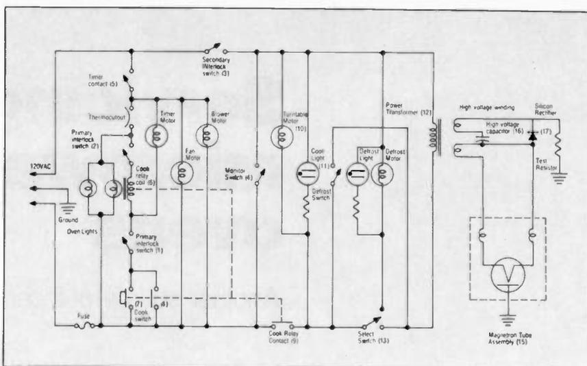
Fig. 3 A typical microwave oven schematic diagram. (Courtesy-Sharp Mfg. Co.)
