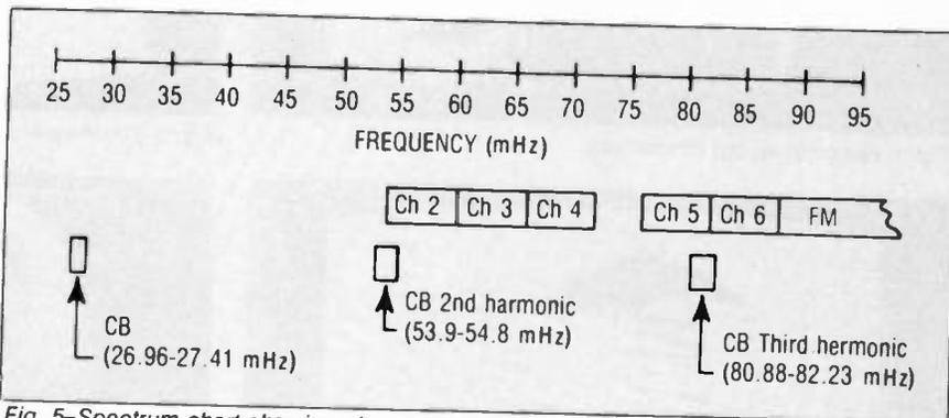
Fig. 5—Spectrum chart showing channels susceptible to interference
