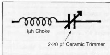
Fig. 8—Series tuned trap
