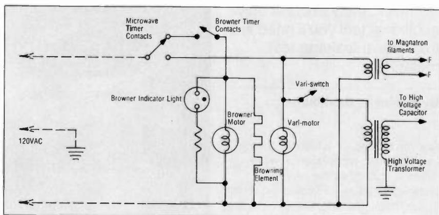
Fig. 4 A partial schematic of the browner unit.
