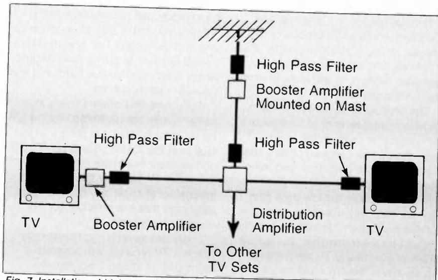
Fig. 7—Installation of high pass filters in a master antenna system
