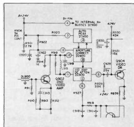
Fig. 1—Automatic peaking circuitry.
