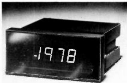
replace the popular Fairchild models 53, 75, and 78 3 1/2 digit units. The Model 78 case fits the same panel cutouts as the Fairchild, plus it has the additional feature of front mounting capability and panel locking retainers. It is available in 200mV, 2V, 20V and 200V ranges at 0.05% accuracy. Parallel BCD units are available as are 5v DC powered units. The Model 78 will be marketed at prices from 20% to 30% lower than Fairchild models in any quantity, offering improved design at low cost.
