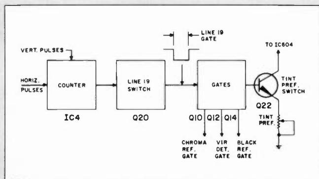
Fig. 4-Simplified schematic line 19 identifier.
