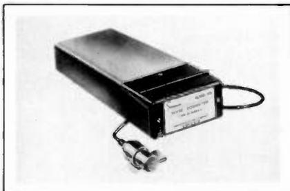
Simpson Electric Company manufactures two noise dosimeters for use in industrial areas where noise levels might be hazardous to a worker's hearing. Both instruments measure and dis-
