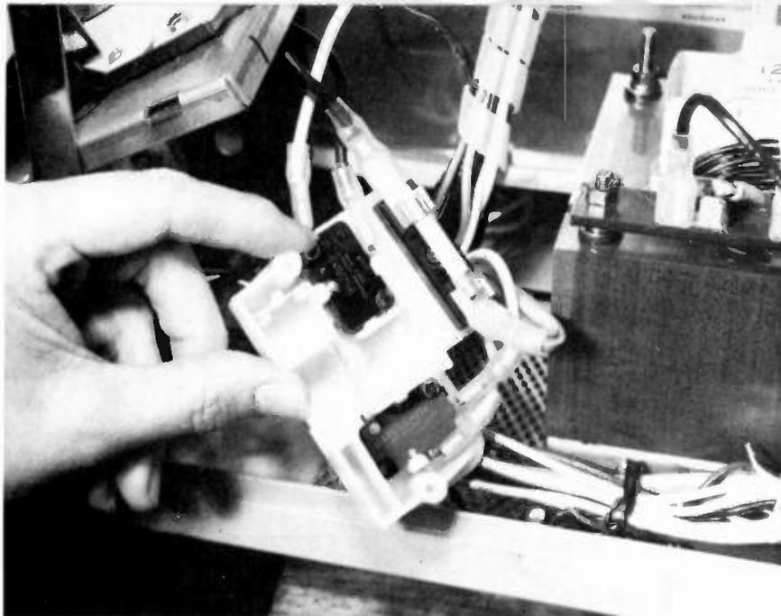
Fig. 8 Many microwave oven repair problems are caused by interlock switches. Either the switch goes bad or may need adjustment.
