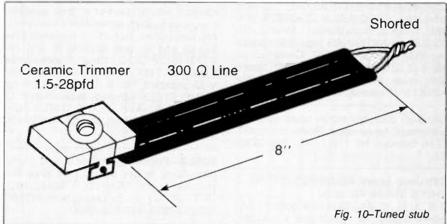
Fig. 10—Tuned stub
