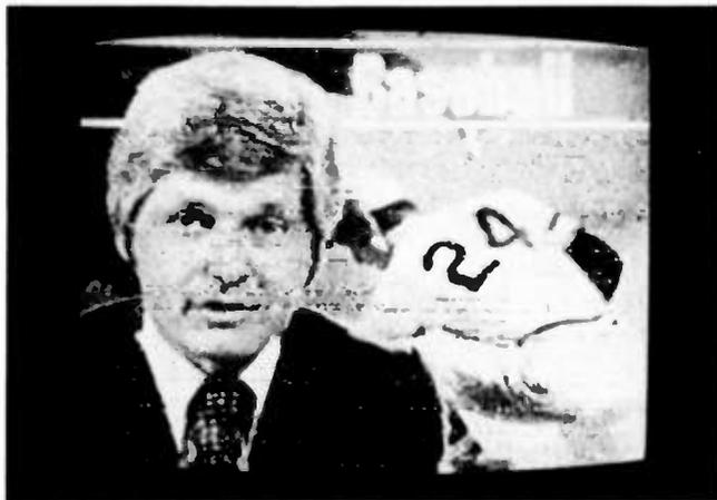
Fig. 1—Electrical arcing interference
