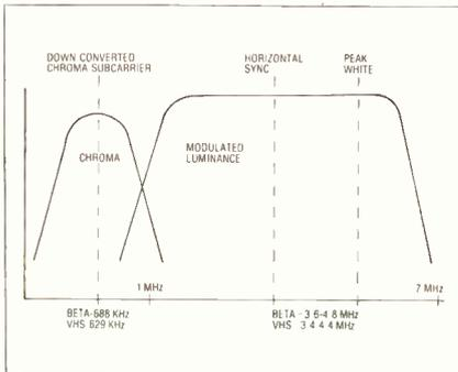
Fig 5 Heterodyning, the process by which two frequencies are beat against one another to produce their sum or difference, lowers the chroma sub carrier so that it occupies the 1MHz region below the luminance signal. The luminance signal then acts as a bias signal when the "down converted" chroma is recorded.
