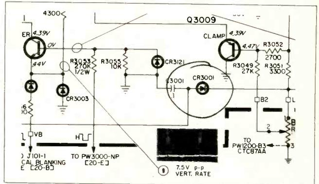
**Brightness increases until shutdown occurs.** Possible cause: leaky CR 3001 in brightness limiter circuit.
