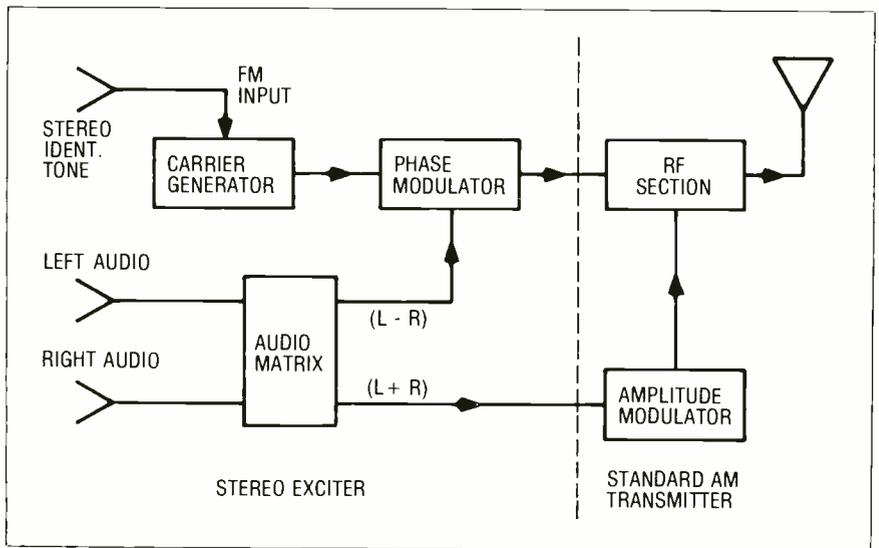
Fig. 1 Block diagram of an AM-Stereo transmitter.
