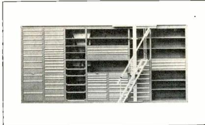
higher locations and folds flat when not in use. Featuring 11 gauge steel frame assemblies, Lista storage walls come in 28 $\frac{1}{8}$  inch, 46 $\frac{7}{8}$  inch, and 56 $\frac{1}{4}$  inch W x 28 inch D expandable units. Drawers are offered in 16 heights and can be mixed with adjustable shelves. Bottom perforations and slots on the 18 gauge inside drawer walls permit various partition combinations.
