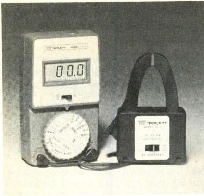
power ohms, auto-zero and auto-polarity and is overload protected up to 600 volts. Battery life is stated to be 200 hours minimum with 9V battery.
