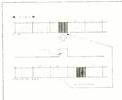
Fig 7 The drop out compensation (DOC) circuits plugs holes in horizontal lines missing video information due to tape imperfections, missing tape oxide, or dirt. The "holes" in a horizontal line are plugged with a portion of the signal from the preceding horizontal line. Most drop outs are less than one horizontal line, but VCR's can repeat a line several times.
