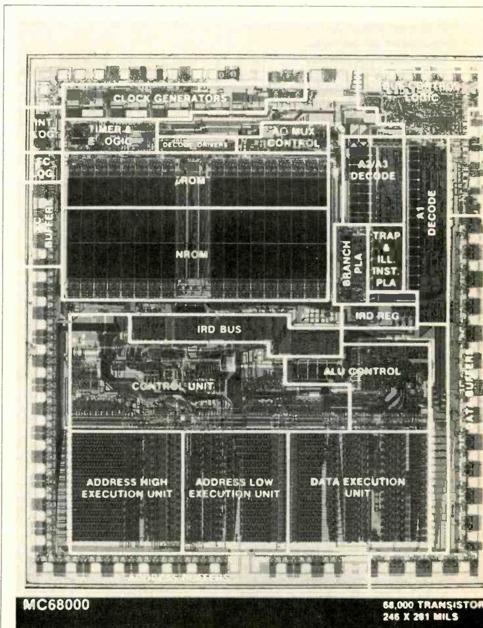
The new Motorola MC68000 is a 16 bit, high-level-language oriented microprocessor. The various functions areas are mapped out on this photo of the approximately one-fourth inch square device.
