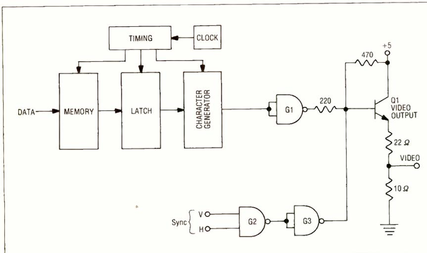
Fig. 3 The principal components of the character generator and video system are the memory, a buffer latch, the generator circuit and composite video.
