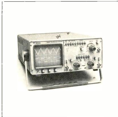
A new lightweight dual-trace 25MHz oscilloscope has recently been introduced by *Gould, Inc.* The OS1200 features a 5 inch rectangular CRT with internal
