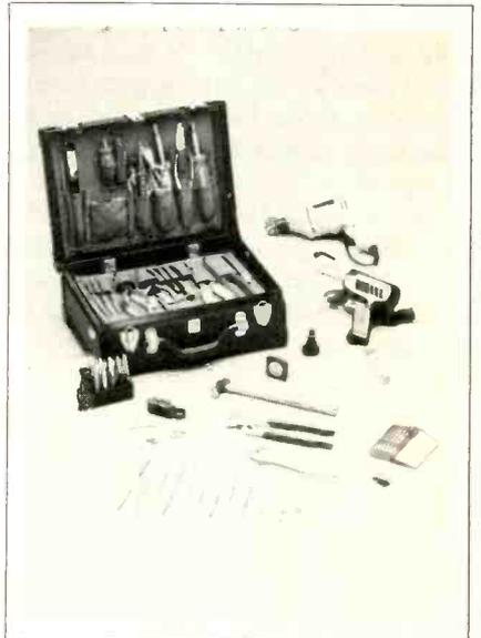
desoldering equipment, solderless terminals, 3/8 inch electric drill and more. In addition there is a selection of specialty and hard-to-find tools to reportedly handle almost any repair or service situation.
