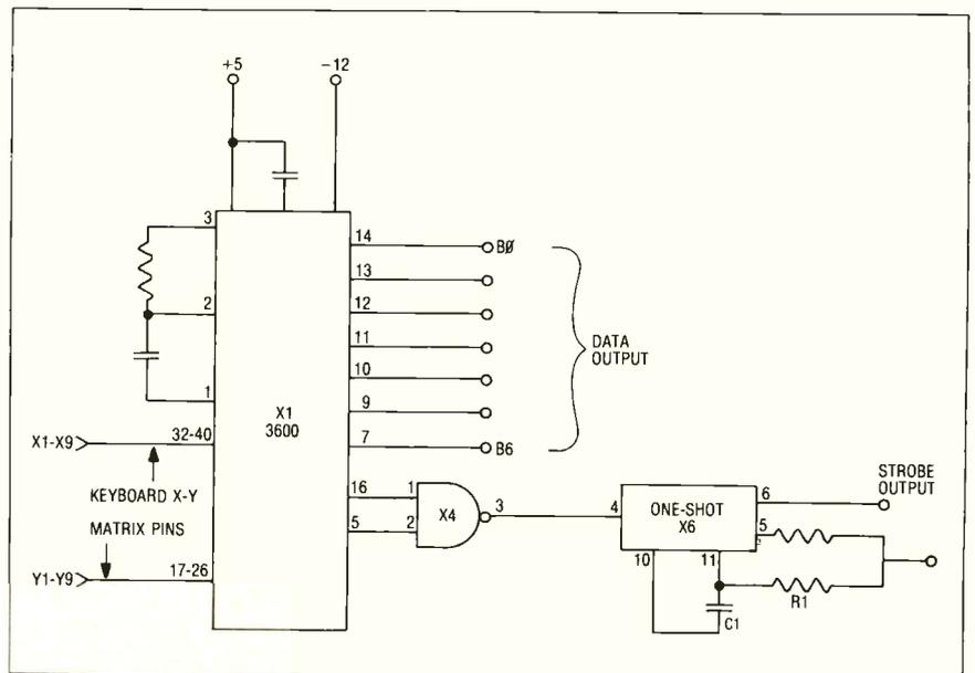
Fig. 1 One of the most popular, and simplest, of all the circuits found in the keyboard section is displayed above.
