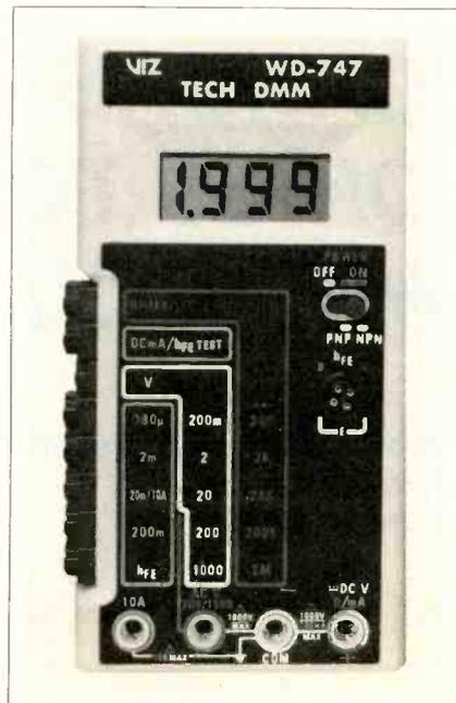
in socket and circuitry for testing transistor h<sub>fe</sub>—reportedly the only 3 1/2 DMM which does. Other features are 1/2 inch LCD readout, side buttons for one-hand operation, resolution down to 100 microvolts, accuracy reportedly better than 0.8%, dc input impedance of 10 megohms, auto-polarity, auto-decimal and full overload protection. All functions are color-coded to reduce risk of operator error. The unit comes complete with 9V battery, deluxe test probes and spare fuse.
