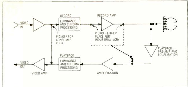
Fig 3 Unique to VCRs is the E-to-E (electronics to electronics) circuit. This circuit allows operational checks of the video input and output in consumer VCRs and most of the record and playback circuitry in industrial units.
