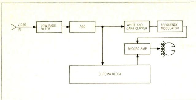
Fig 2 The luminance blocks of both the VHS and Beta recorders are about the same and consist basically of those shown above. The luminance signal recorded on tape is an FM square wave.
