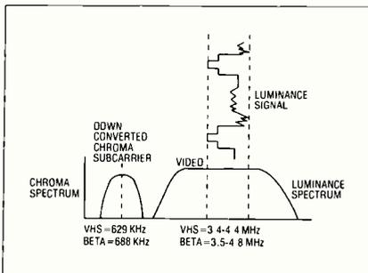
Fig 1 The information recorded on a video tape includes a "down converted" chroma subcarriers and a luminance signal. Down conversion of the chroma is necessary to record it on video tape because of the tape's response characteristics.
