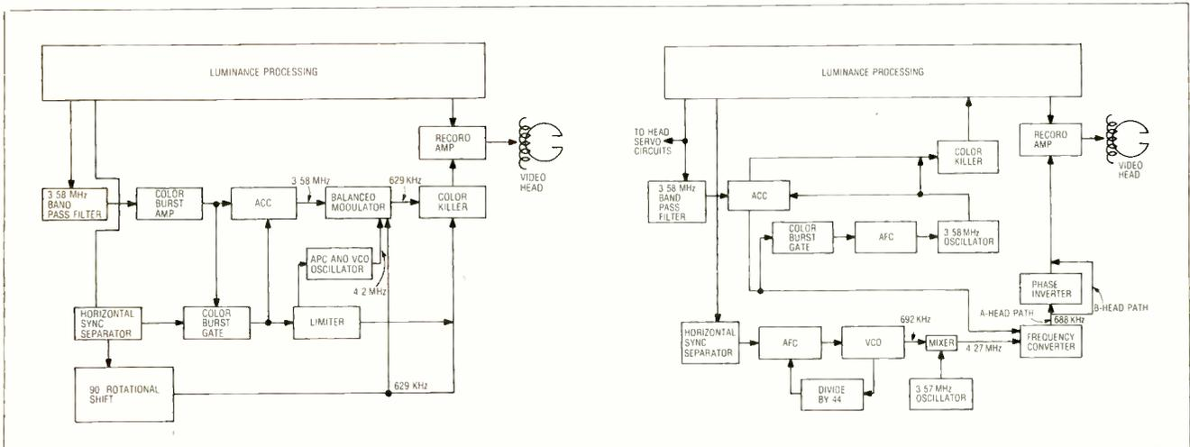
Fig 4 The simplified block diagrams shown above give a basic concept of the similarities and differences between the VHS (4A) and Beta (4B) chroma record operation.
