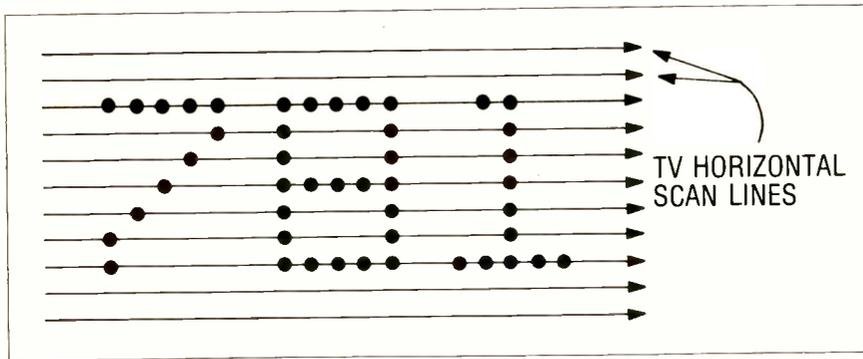
Fig. 2A & 2B Shown above are graphic representations of how the video terminal display creates the characters. At points where dots occur the terminal's electronics issues an unblanking signal that turns on the CRT to produce the spot of light.
