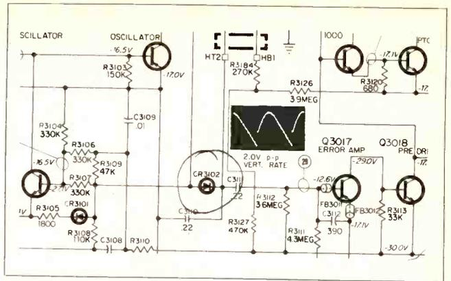
**Vertical overscan and retrace lines in top half of picture.** Possible cause: leaky CR 3102 in vertical oscillator circuit.
