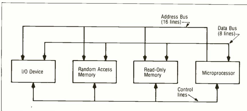
Fig. 1 Block diagram of a microprocessor system
