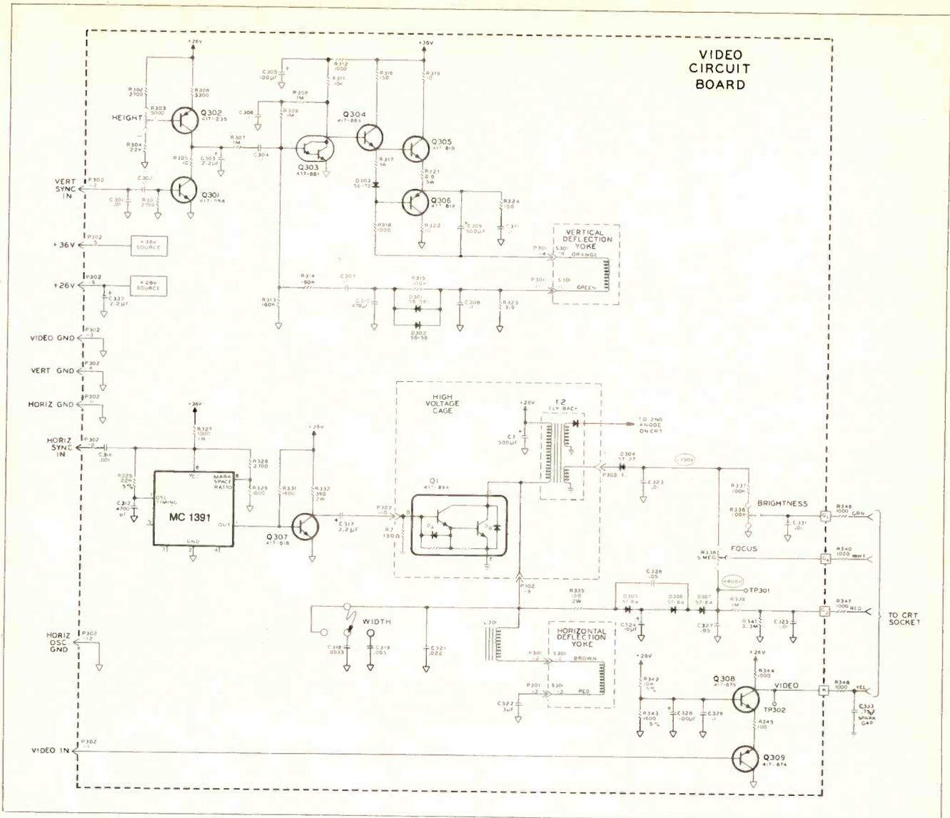
Fig. 4 Schematic drawing of the video board from a Heath model H9 video terminal.
