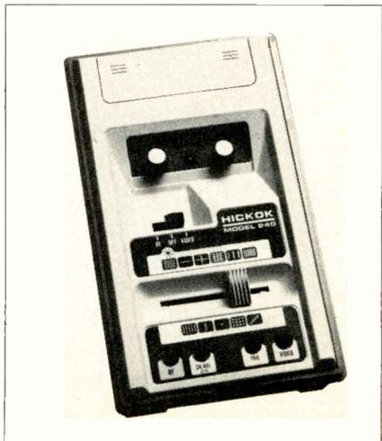
case simplifies detection of video compression, poor band-width and other problems in almost any stage. The three bar gated rainbow permits fast, easy chroma checks and is particularly useful on vectorscope measurements. Other features of the new Hickok Model 240 Video Generator include adjustable chroma levels from 0-125%, crystal controlled chroma and timing oscillators for stability from  $-20^{\circ}$  to  $125^{\circ}$ F and non-skid rubber feet that prevent marring of the work surface.
