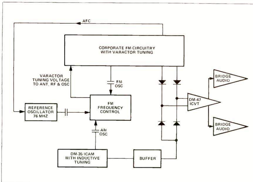
Fig. 6 This diagram of a low cost electronically tuned system uses a local AM oscillator to derive the tuning potential for the FM section.
