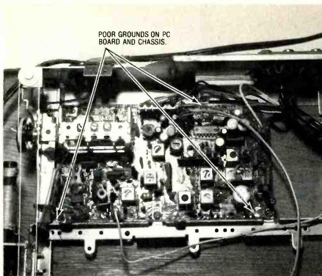
*Fig. 3 Check for poor grounded terminals between PC board and chassis ground. In audio circuits, you may have to tie all the ground cables together to prevent hum.*
