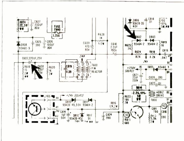
**6. Dark at top, light at bottom, no brightness control.** Possible Cause: Defective D602 (93A64-2).
