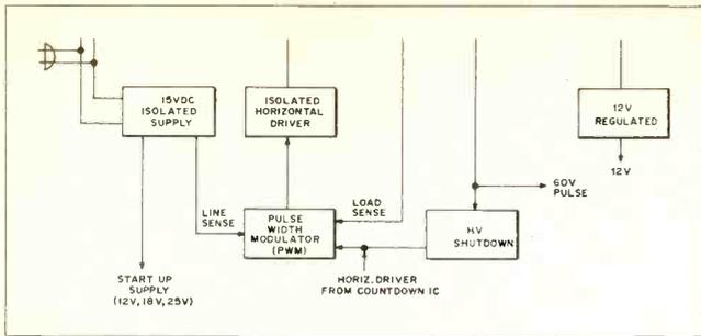
Fig. 2 Block diagram of the electronic power supply
