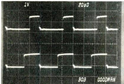
Fig. 9 Waveforms of the PWM action. Top trace shows pulse width with 130VAC while bottom trace was recorded with 75 VAC.
