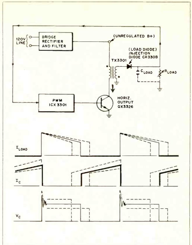
Fig. 3. The chopper circuit and waveforms
