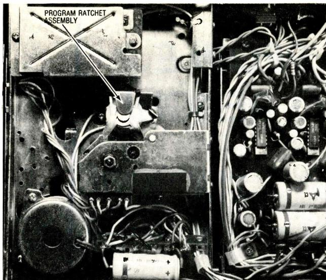
Fig. 6 A clicking or popping noise may be caused by a noisy solenoid or poor wiring connections of the solenoid ratchet assembly.
