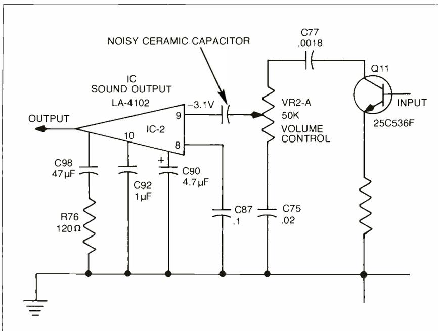
Fig. 8 The noisy amplifier circuit was produced by a defective ceramic coupling capacitor, C84 in a Penney's model 3877.
