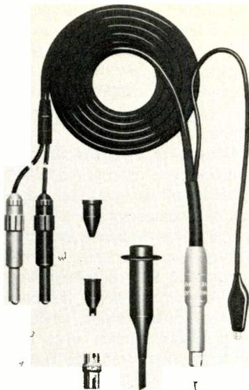
plete with sprung hook, BNC adaptor, I.C. tip and insulating tip and lists at \$45.00. The optional adaptor sleeves list for \$3.00 per set, one red, one black.
