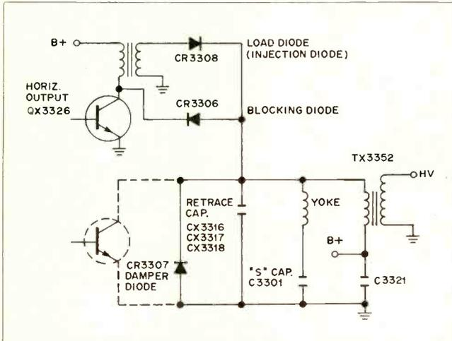
Fig. 4 The self-regulating sweep system
