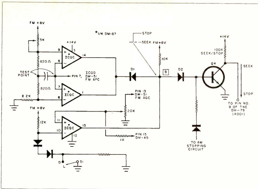
Fig. 5 Schematic of the AM stop circuit
