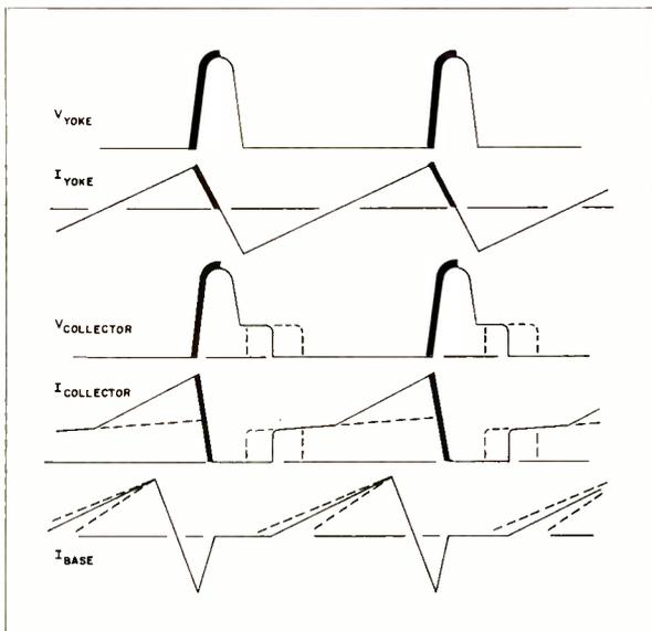
Fig. 5 Waveforms for start of retrace
