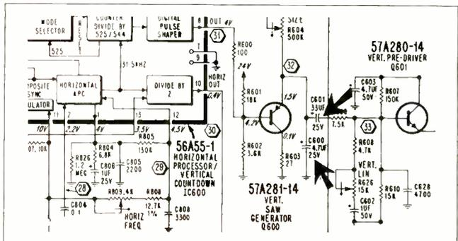
**4. Vertical foldover with drive lines.** Possible Cause: Defective C601, 33mfd, 25V (67A201-330-4).
