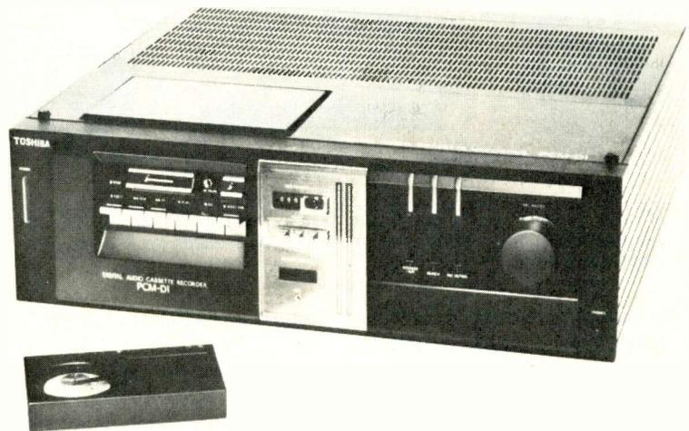
The highly compact combination pulse code modulator and Beta format VCR from Toshiba.
