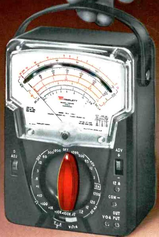
Fifty-eight VOM ranges are available at the flick of a single switch on the versatile Model 630-NA and 57 ranges on Model 630-NS. And, the 1½% DC accuracy rating makes them adaptable for exacting electronic/electrical testing in the lab or shop. Ruggedly built and field-proven for communications, utility, industrial and general service work, the 630-NA offers 20,000 ohms per volt sensitivity and the 630-NS features 200,000 ohms per volt sensitivity.
