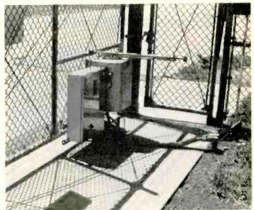
Fig. 5 Motorized gate controllers: Their installation involves excavation and laying underground cable.
