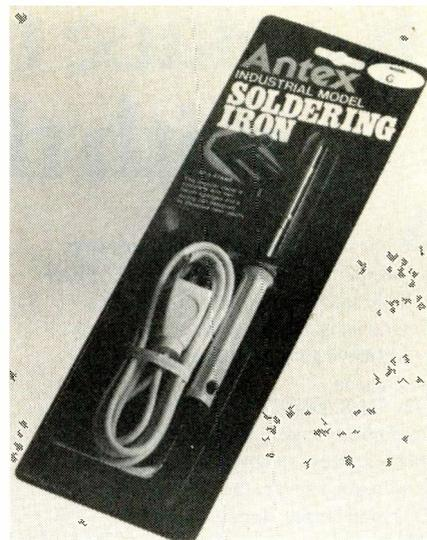
heating element for efficient power usage. The Antex Model G/3U has a flexible, 3-wire, 6 ft. cord. Weighing 3/4 oz. the 6 1/2" non-charring plastic handle reportedly remains cool even with tip temperatures of 725°F. 41 tips from 0.012" to 3/16" Dia., and a soldering stand are optional. The Antex Model G/3U is priced at \$14.95 (retail); stand is \$5.50.
