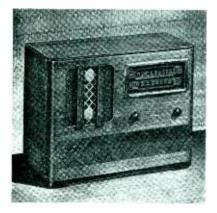
ADMIRAL 43-B4 This 4 tube, 11/2 volt, superheterodyne features a 6-inch, speaker, a tuning range from 535 to 1730 kc., iron core i.f. transformer, soft gold escutcheon and large slide rule dial with easy-to-read etched glass scale. Table type cabinet, designed to accommodate battery below chassis. List \$27.50.
