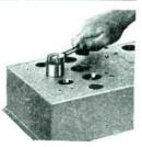
Here's a handy tool to help the radio worker save many hours of work when cutting holes for sockets, plugs, connectors, and other receptacles in radio chassis. No tedious drilling, reaming or filing is necessary. A cap screw is inserted in a small drilled hole, and the punch is easily forced into the die by a few turns of the cap screw with an ordinary wrench. Smooth holes up to 21/4 inches can be cut in metal up to 1/6-inch thick in 11/2 minutes or less.
