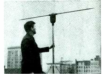
Engineer Virgil Bowman checks remote controlled tele antenna designed for the purpose of eliminating reflected shadows.
