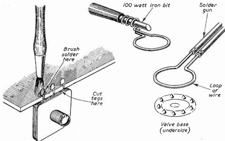
Fig. 3: Methods of removing tagged controls and valve bases.
