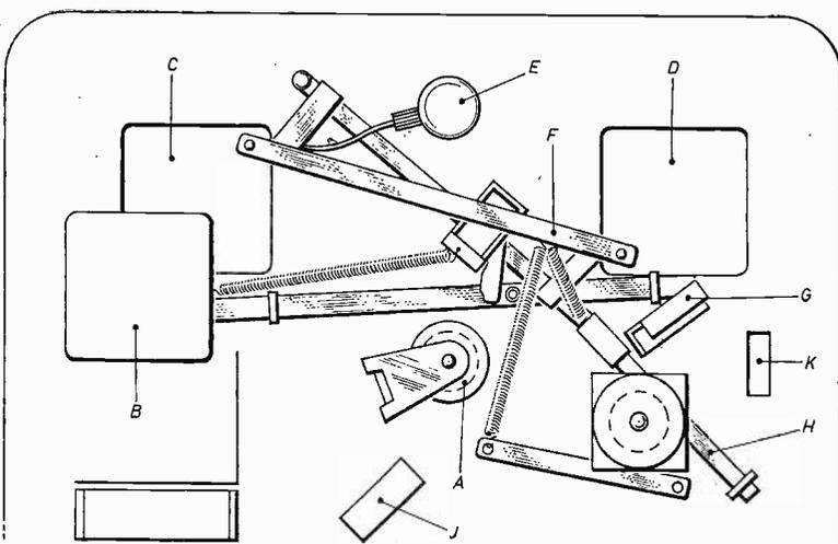
Fig. 2: Sketch showing a general view of the underside of the Wearite 4 tape deck. For key to reference letters, refer to text.
