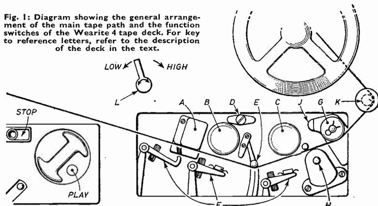
effected by selecting a step on the motor spindle capstan, which engages an idler pulley, in turn driving the heavy flywheel, with a direct shaft tape drive.
