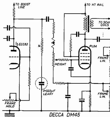
Close inspection of the raster showed that sync was arriving, and with reduced height it was possible to control the frame speed but not
