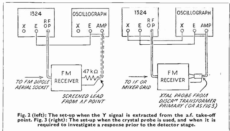
Fig. 2 (left): The set-up when the Y signal is extracted from the a.f. take-off point. Fig. 3 (right): The set-up when the crystal probe is used, and when it is required to investigate a response prior to the detector stage.
