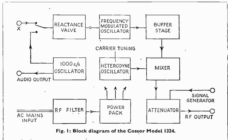
Fig. 1: Block diagram of the Cossor Model 1324.
