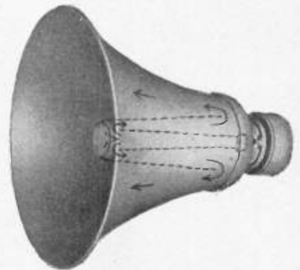
Left —MARINE SPEAKER; approved by the U. S. Coast Guard, for all emergency loudspeaker systems on ships. Re-entrant type horn. Models up to 50 watts. May be used as both speaker and microphone.
