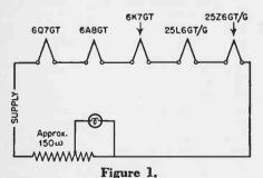
resistor is shown as a tapped resistor since in many cases ballast resistors with the tap were used. In this case the pilot lamp rating will
