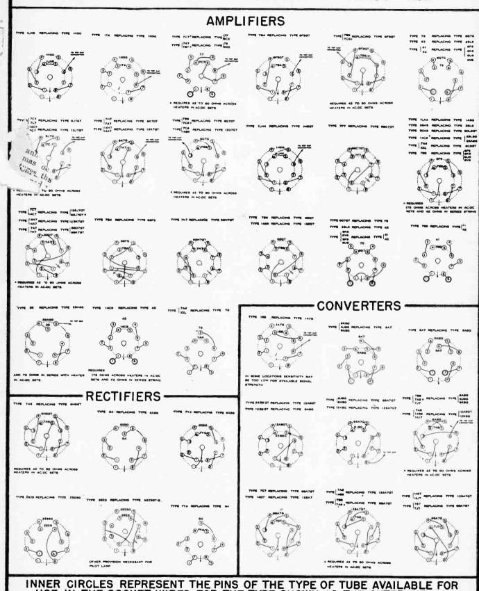
INNER CIRCLES REPRESENT THE PINS OF THE TYPE OF TUBE AVAILABLE FOR USE IN THE SOCKET WIRED FOR THE TYPE SHOWN AS THE OUTER CIRCLE. THE SOLID LINES SHOW THE WIRING FOR EITHER AN ADAPTOR OR FOR RECONNECTING TO THE SAME OR TO DIFFERENT SOCKETS.
