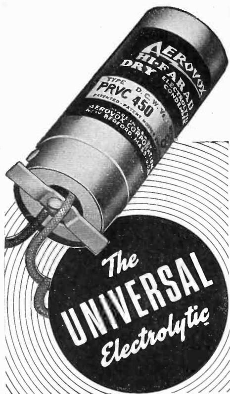
• Now available in aluminum-can construction—the postwar Aerovox Type PRVC cleat-mounting universal replacement electrolytic. Readily doubles for twist-prong, spade-lug and screw-base types. Insulated positive and negative wire leads. Multiple sections have concentrically-wound sections with common negative. In all popular voltages and capacitances.
