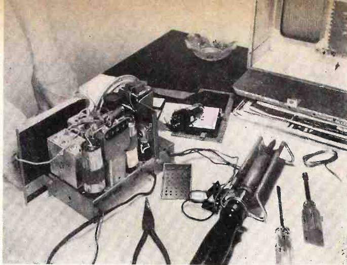
Figure 2. Selenium rectifier in typical 3-way set.
