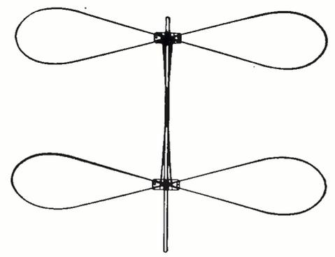
radical departures in TV antenna design. High gain and signal to noise ratio are obtained over the entire TV and FM bands, and especially at the high frequency channels, due to the flat impedance characteristics and complete absence of "lobe-splitting" over the full frequency range.
