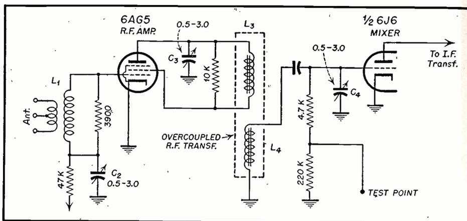
Fig. 3-14: Simplified schematic of r-f stage of Standard Tuner, illustrating simple overcoupled r-f transformer.
