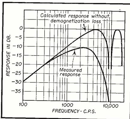
Fig. 7. Curves showing effect of demagnetization upon frequency response.
