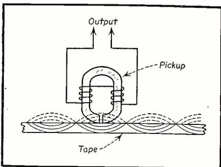
Fig. 6. Interception of tape recording of a sine wave. (From Wetzel)
