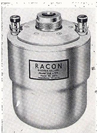
The voice coil is wound with aluminum wire for greatest efficiency and coil terminals are welded instead of soldered. The voice coil lead is a strip of fatigue-resistant beryllium copper to withstand abnormal diaphragm excursion. The voice coil suspension is made of bakelized linen firmly cemented to the phenolic diaphragm
