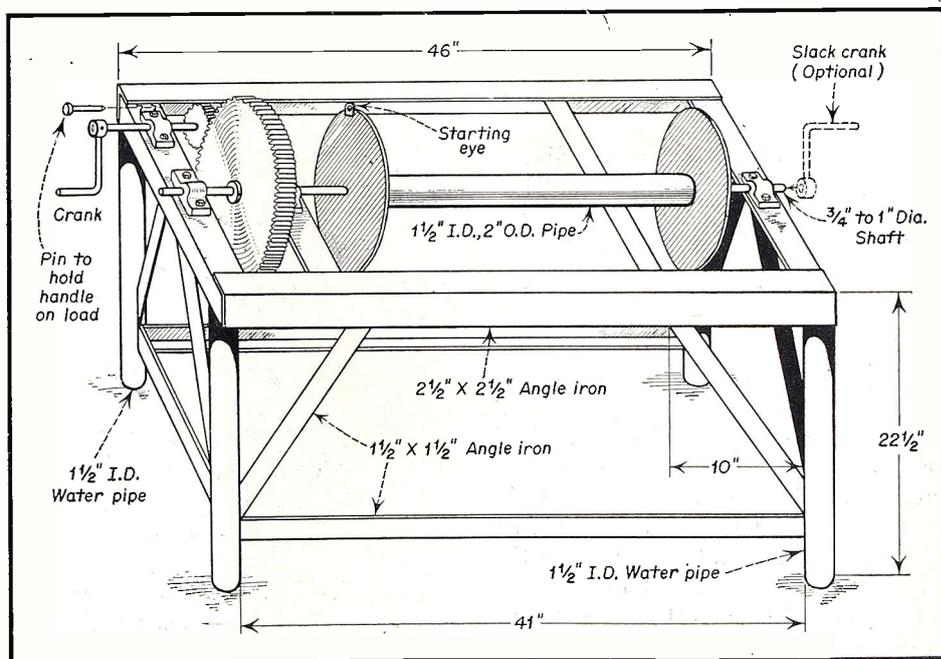
**Fig. 1.** Illustrating winch described in this article. Parts were made from discarded farm implements, etc.
