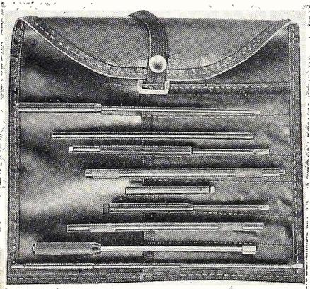
The tools will fit the adjusting screws of all types of r-f and i-f transformers, solder and trimmer condensers, used in most every TV receiver.
