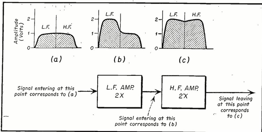
Fig. 3-17. Illustrating the manner in which the output of a stagger-tuned amplifier contains equal values of amplified high and low frequencies.
