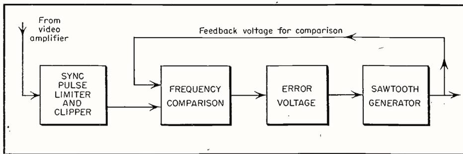
Fig. 2. Basic elements of horizontal a.f.c.
