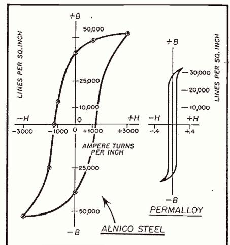
Fig. 2. Hysteresis curves of Alnico steel and Permalloy.
