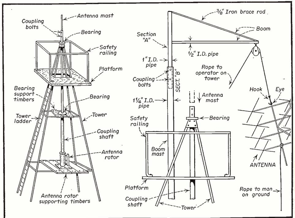
Fig. 4 (left). Position of railing around platform. Fig. 5 (right). Using a small boom for erecting or taking down a heavy array from a windmill tower.
