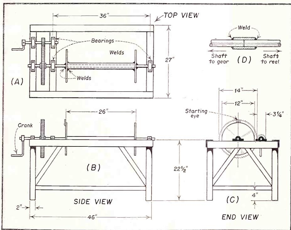
Fig. 2. Side and end views of winch shown in Fig. 1. Reel details are also given in this figure.
