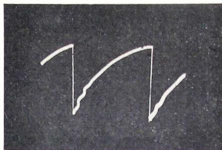
Fig. 4. Output wave shape from synchrolock circuit in Fig. 3. (60 volts peak to peak)
