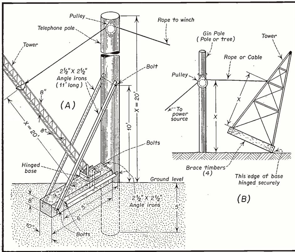
Fig. 3. Gin pole details, showing dimensions and relative position of gin pole and mast to be raised.
