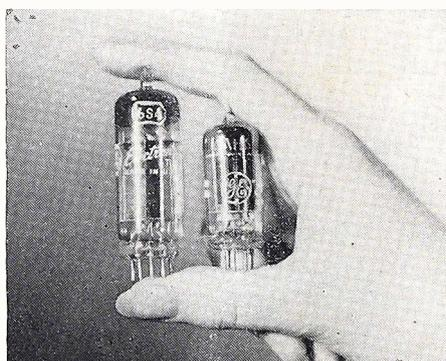
The 6AH6 is a sharp-cutoff amplifier pentode. Its high transconductance and low input and output capacitances adapt it to use as a wide-band amplifier and as a reactance tube for television and radio receivers. Under typical operating conditions it has a transconductance of 9000 microhms and plate current of 10 milliamperes.
