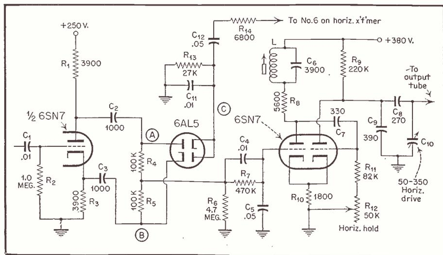
Fig. 5. Phase detector—a-f-c.
