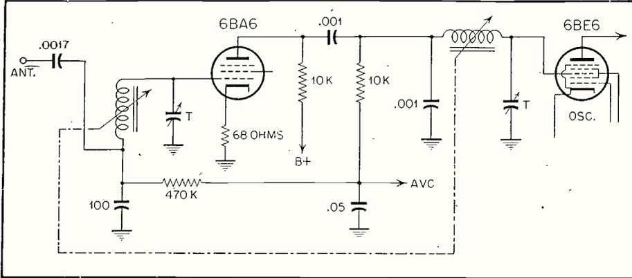
Truetone Model D 4842. Variable inductance tuning by means of iron cores is used in antenna, mixer, and osc. stages.
