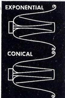
Only Racon re-entrant trumpets incorporate true exponential design for their complete length! Well-established acoustical fact, as the curves graphically show, proves the superiority of exponentially designed Racon trumpets. This means greater efficiency, greater power output, greater projection distance and better low frequency response. That's why, dollar for dollar, the RE-35 is truly America's greatest 3½" trumpet value!
