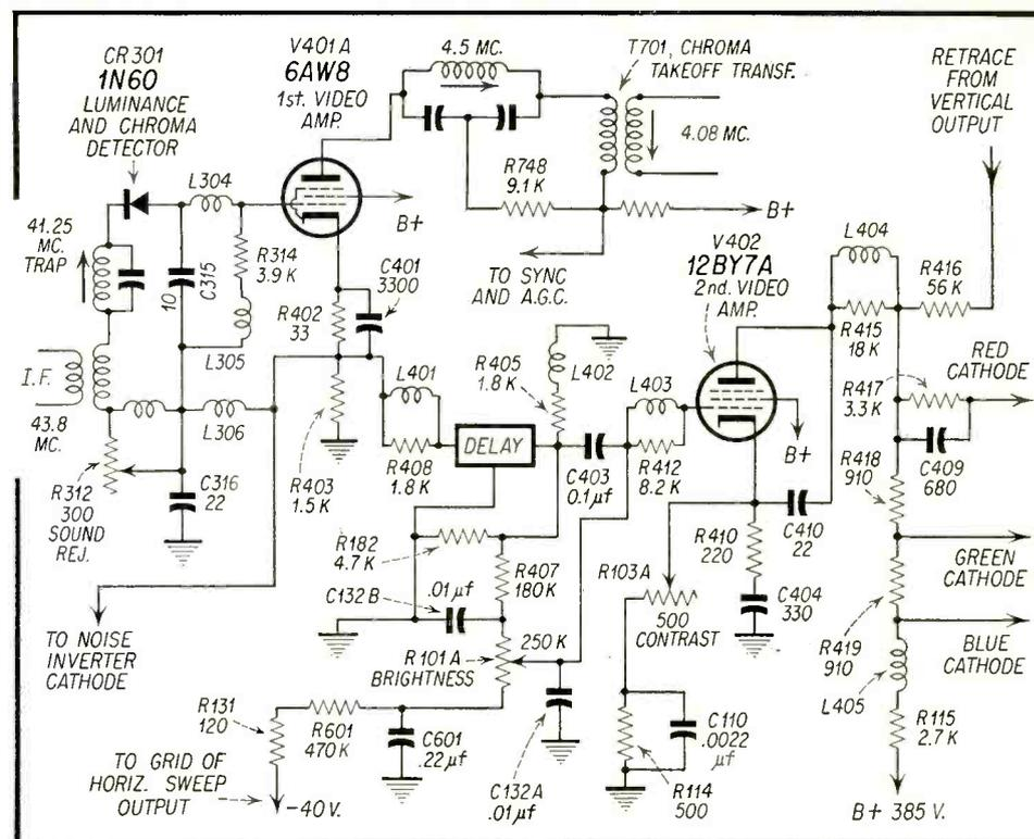
Fig. 3—The circuit diagram corresponding to the block diagram of Fig. 1B. The picture polarity is positive as applied to the first video amplifier.
