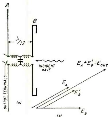
Fig. 5—The basic elements and a vector relationship for low band operation without signal delay.
