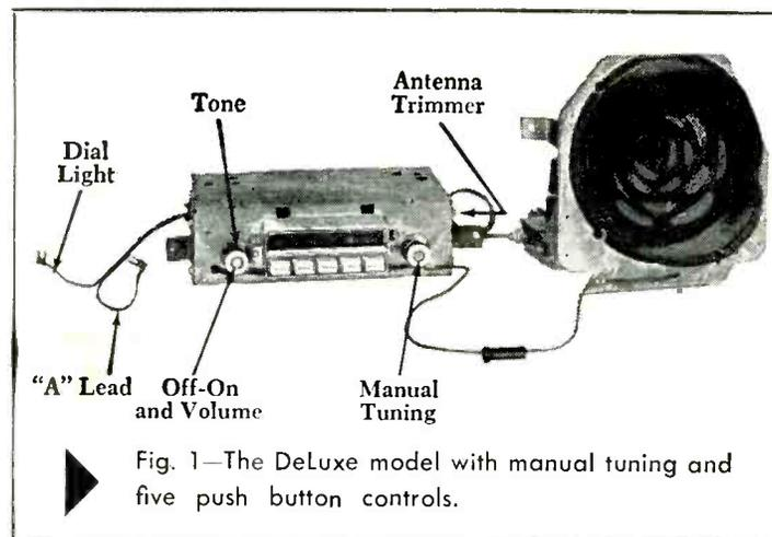
Fig. 1—The DeLuxe model with manual tuning and five push button controls.
