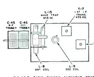
FIG. NO. 3 RADIO CHASSIS ALIGNMENT POINTS
