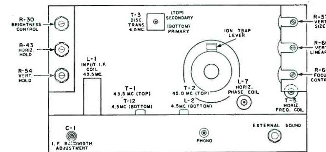
FIG. NO. 4 T.V. CHASSIS ALIGNMENT POINTS
