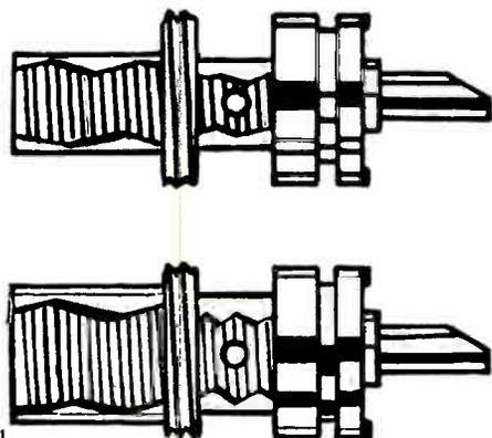
Fig. 8—Blonder-Tongue solderless cable connectors.
