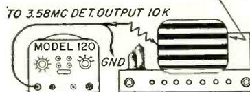
Fig. 5—Hookup to check and align reference oscillator.
