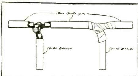
Fig. 1—Original method of tapping transmission lines.
