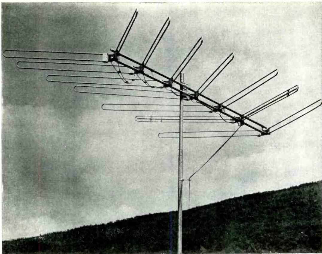
► Fig. 1—Seven element terminated travelling wave antenna.
