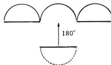
Fig. 4—Phase of current in high band dipole changes 180 degrees.
