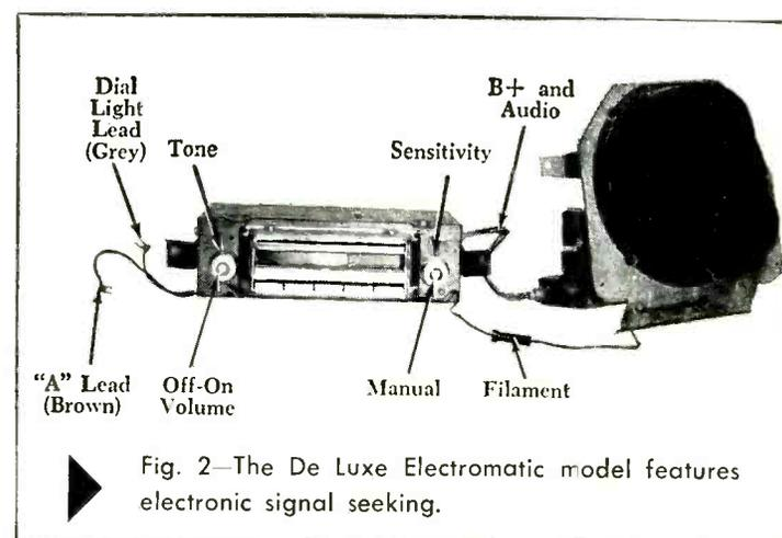
Fig. 2—The De Luxe Electromatic model features electronic signal seeking.
