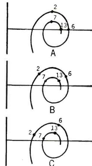
Fig. 7— $Z$  of dipole nearest feed point is at (A); second dipole (B); and third dipole is shown at (C).
