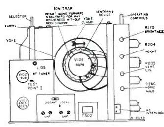
Fig. 1. Rear View of Chassis Cabinet Removed
