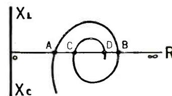
Fig. 6—Typical spiral curve of the impedance of a dipole.
