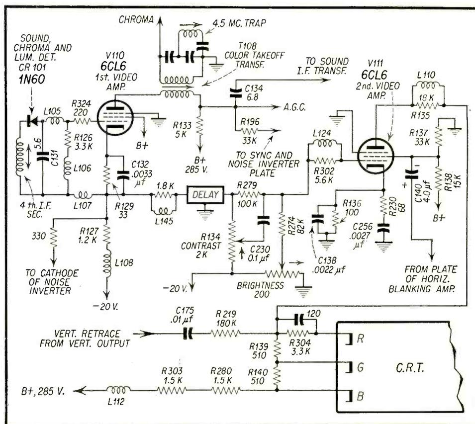
Fig. 4—The circuit diagram corresponding to the block diagram of Fig. 1C. The detector output circuit contains sound, chroma, and luminance signals.
