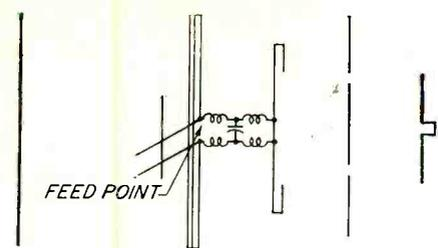
Fig. 1—Schematic drawing of a controlled drive type of antenna showing connecting delay network.
