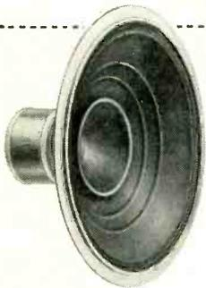
Norelco's twin-cone speakers are designed to meet the problem of high and low frequency dispersion in a single speaker. The large (heavy) cone is designed to produce good bass while the small (light) cone radiates higher frequencies.
