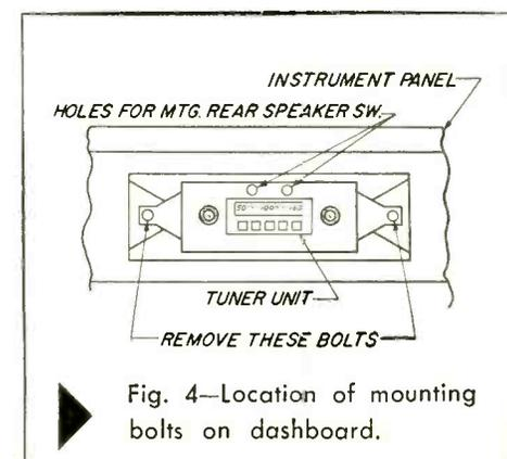
Fig. 4—Location of mounting bolts on dashboard.
