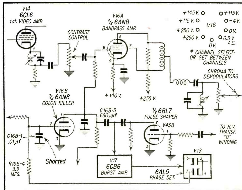
Fig. 1—Partial schematic of CBS TV receiver showing bandpass amplifier, color killer, pulse shaper, video amplifier and connecting circuitry.
