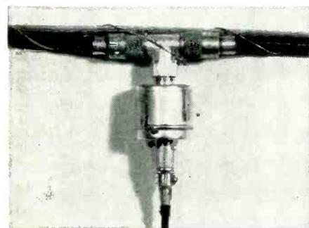
Fig. 3—Lynmar transmission line tapping device.
