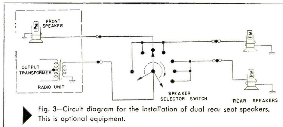
Fig. 3—Circuit diagram for the installation of dual rear seat speakers. This is optional equipment.
