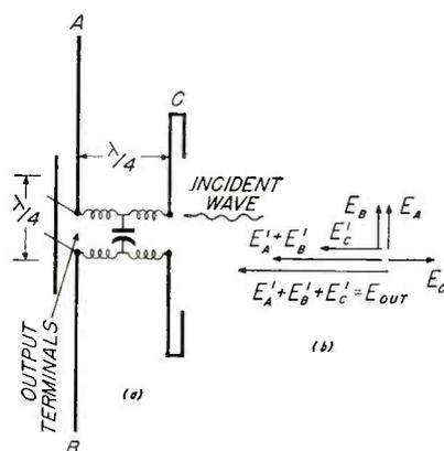
Fig. 4—The frequency selective delay line insures additive in-phase signals at the output.
