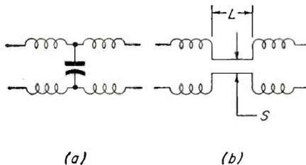
Fig. 6—(a) Delay line schematic. (b) Design considerations are length  $L$ , space  $S$ , and diameter.
