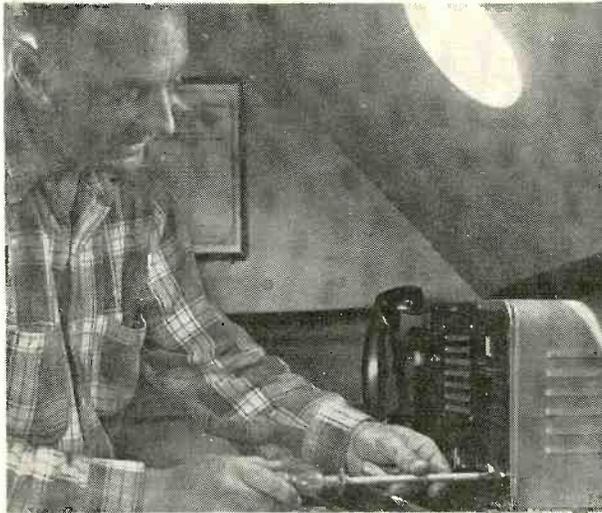
▶ Place equipment so that it is accessible for servicing. Heavy paper or a towel should be used to protect varnish finishes.
