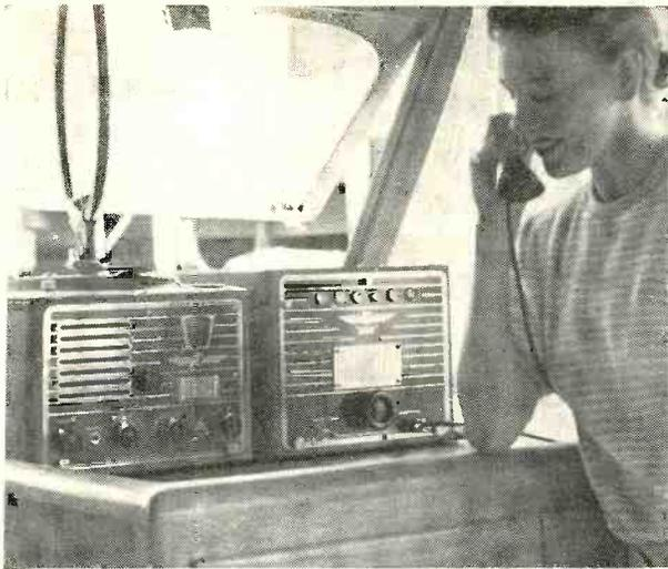
▶ Placing equipment as shown allows concealed wiring within cabinet. It should also be convenient to batteries, antenna, and ground.
