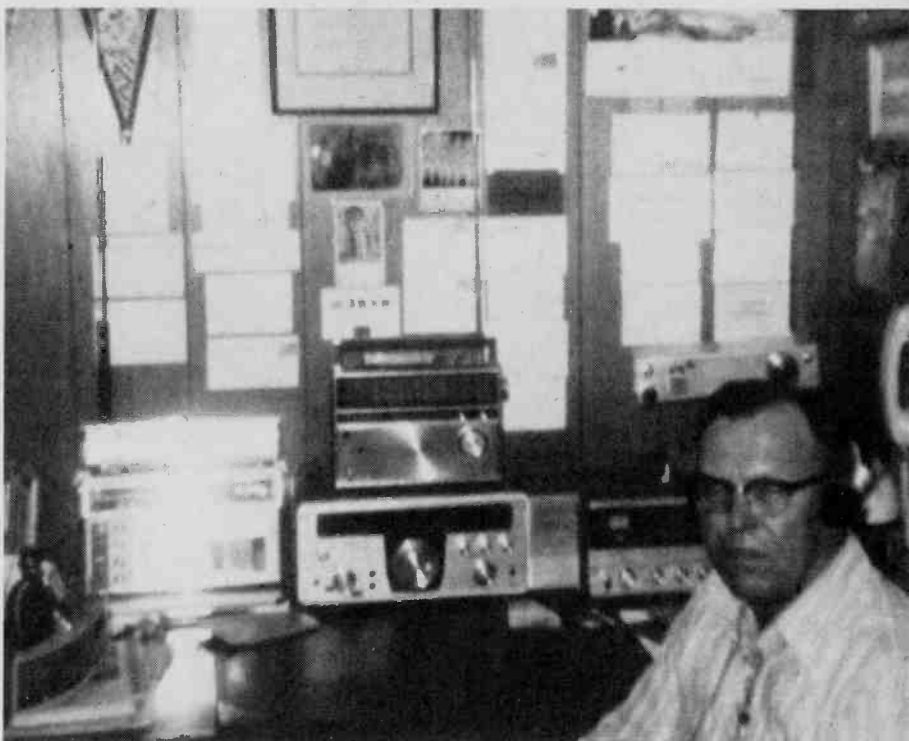
This attractively paneled DX den belongs to Leland Swenson of Scandinavia, WI. A DXer for about five years, Leland's listening gear includes, from left, a Zenith Transoceanic portable, a Radio Shack DX-190 with a Realistic Patrolman 6 on top, and a Realistic DX150A communications set.
