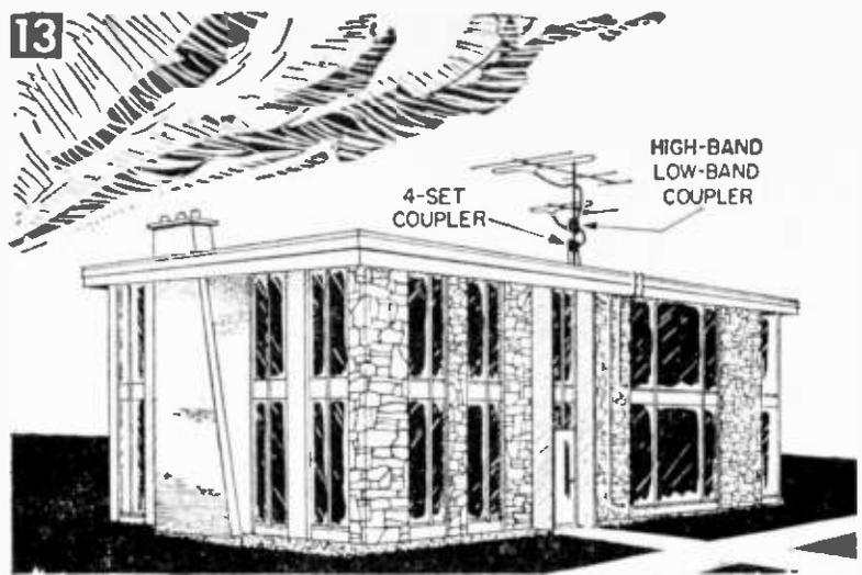
ting, you can couple the two lines together and run one line only by using a high-band, low-band VHF coupler (Fig. 13). This requires that you bring in only one wire to the 2-set or 4-set couplers in various apartments. Cost per outlet will be less. Also, couplers are available for connecting separate VHF and UHF antennas to a single line. These couplers are also excellent for homes.
