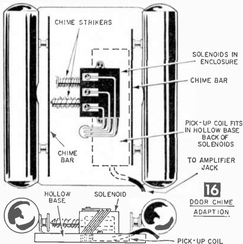
you are ready for the final test. Place the pick-up baseboard in position, telephone a friend and ask him to call you back. Then stand aside and see your first call come in. If light does not operate properly, experiment by moving pick-up coil baseboard a bit.
