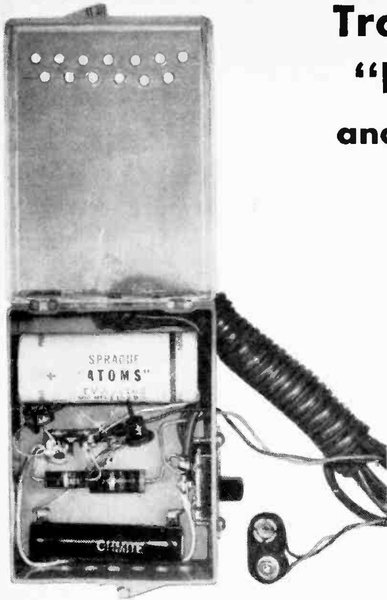
House-current is converted by this unit to power transistor radios. If battery is left in radio, unit will charge it while powering the radio.
