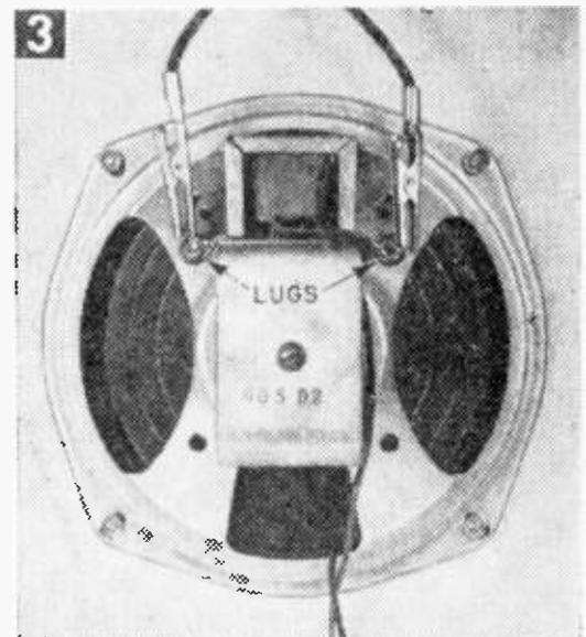
Left, doorbell button, plastic coaster and cord are dime store items. Auto shops have clips. Right, Some sets have output transformer mounted on speaker; concealed in others. Regardless, attach clips to the lugs on speaker.
