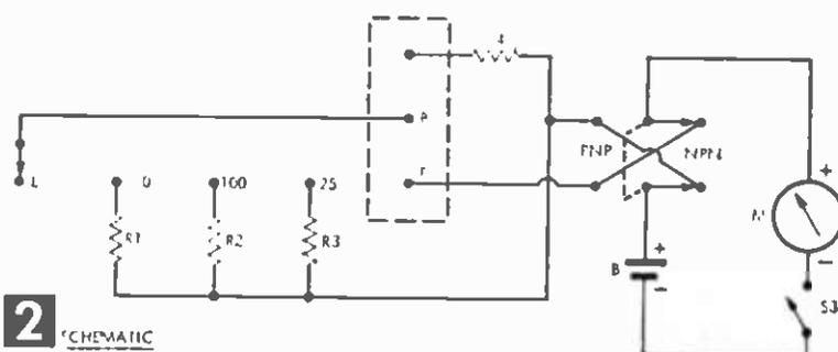
This compact transistor tester has these features, and in addition is small enough to fit in your pocket (case is only  $1\frac{5}{8} \times 2\frac{1}{8} \times 4$  in.). The case is a rugged aluminum box that can stand rough handling. And the batteries are penlite cells—easy to obtain anywhere.
