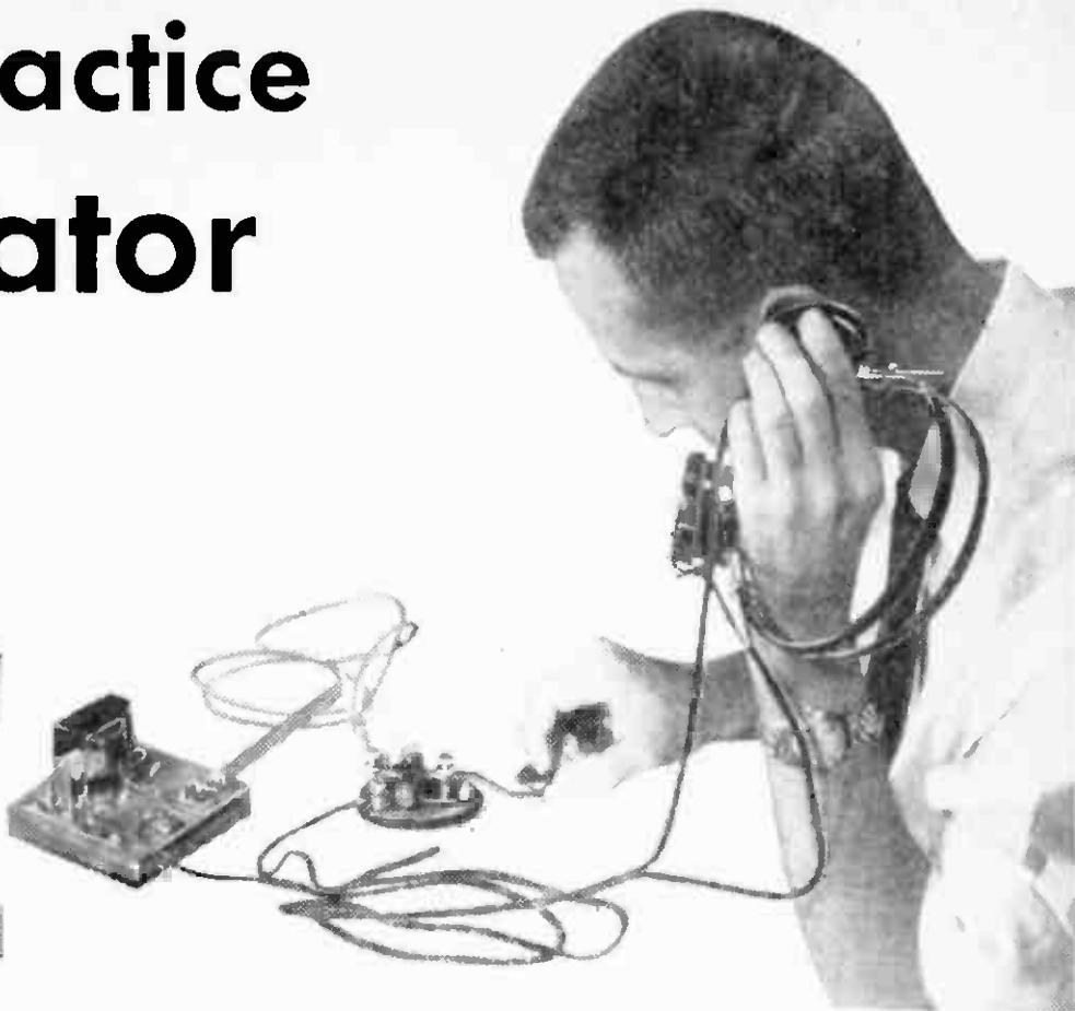
A quick dip of the blotting paper, place it between the brackets, and you've set the set to buzzing, ready to key off for code practice.
