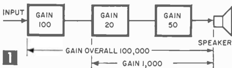
Hum introduced in first stage is amplified more than hum introduced in subsequent stages.
