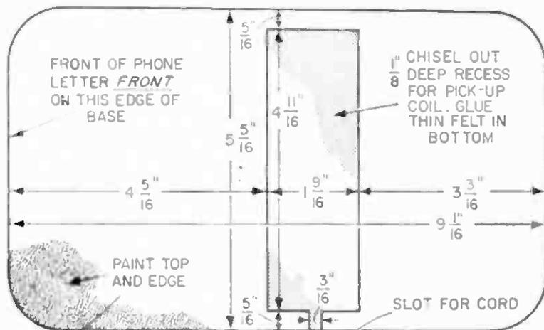
PICK-UP BASE TO FIT NEW STYLE PHONES THIN FELT GLUED ON BOTTOM
