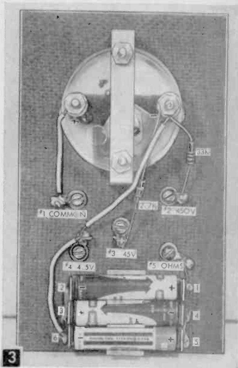
Parts mounting. Piece of #18 wire (arrow) supports battery holder.
