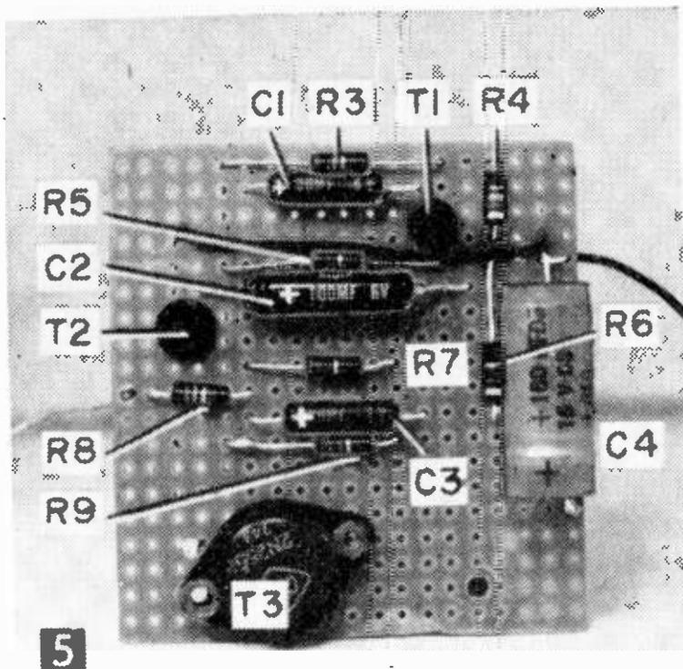
Amplifier parts are mounted on Bakelite piece.
