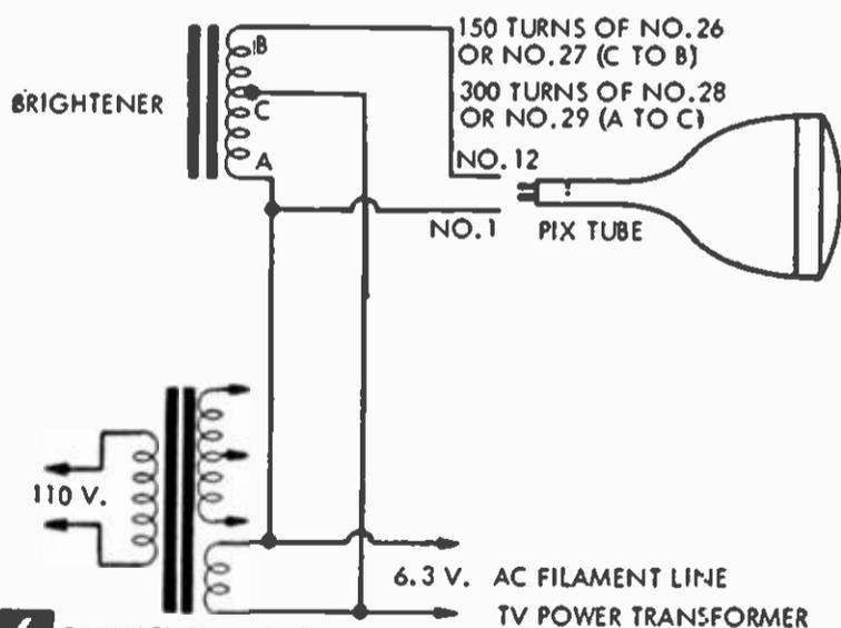
6 PARALLEL FILAMENTS SCHEMATIC
