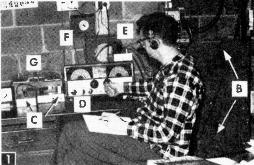
Here Walter Bain demonstrates the equipment needed to get into meteor trail work: A) transmitter; B) transmitter power supply; C) frequency marker; D) communications receiver; E) crystal controlled converter; F) clock with sweep second hand; G) tape recorder (optional).
