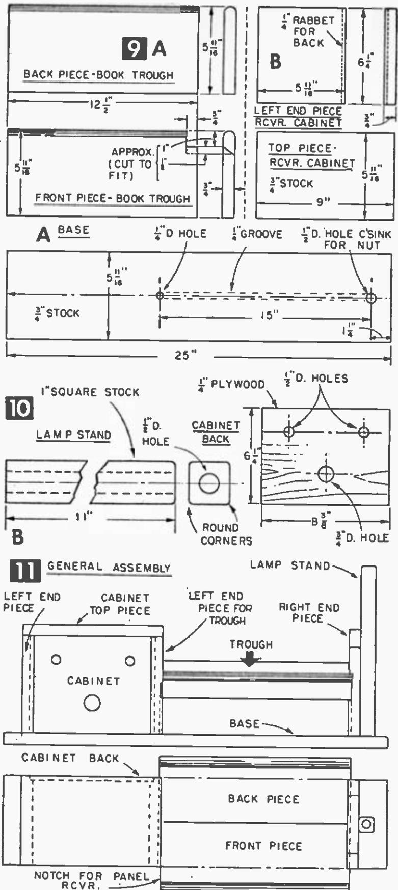
nect about 3 ft. of rubber-covered lamp cord to the socket and assemble after passing the cord down through the lamp tubing to the bottom of the base. Run the lamp cord through the groove and pass it up through the  $\frac{1}{4}$ -in. hole into the cabinet.
