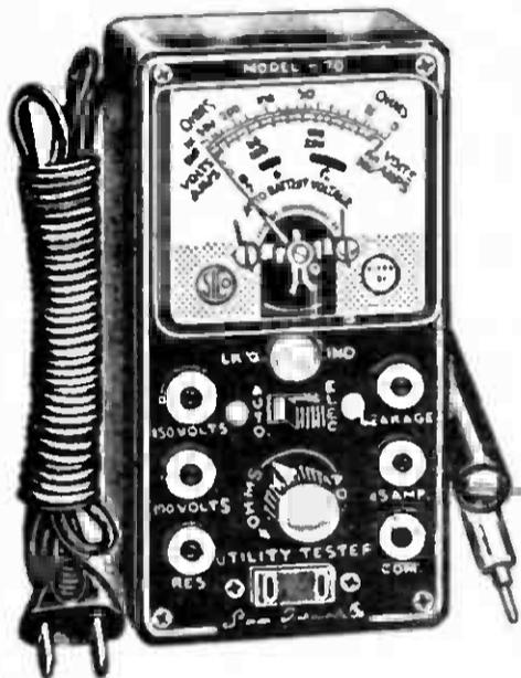
All electricity is measured by (1) voltage, (2) current, (3) resistance. You can test either, any or all by merely touching 2 points of contact on any electrical device with our prod and clip. Results are indicated on the meter of our new Model 70 Utility Tester. Repair procedure is outlined in our Tester Use Book.
