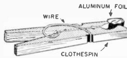
• If you run out of battery clips while doing an electrical project, make a substitute clip by wrapping aluminum foil around the tips of a spring-type clothespin. Wrap wire around foil.—J. HARVEY.
