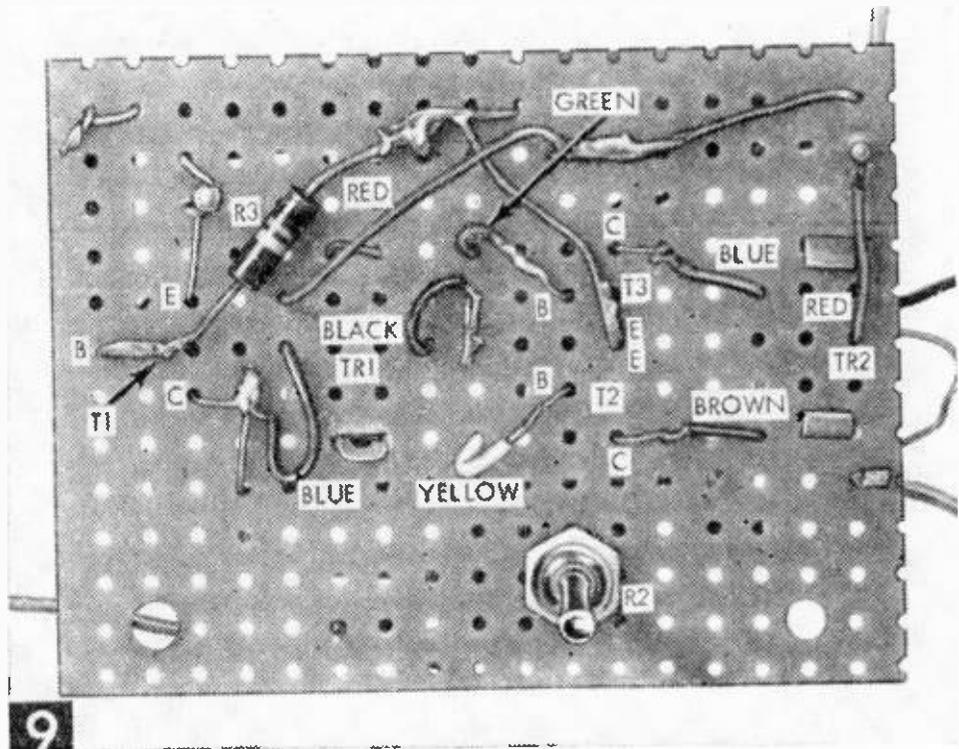
Bottom view of amplifier shows wiring.
