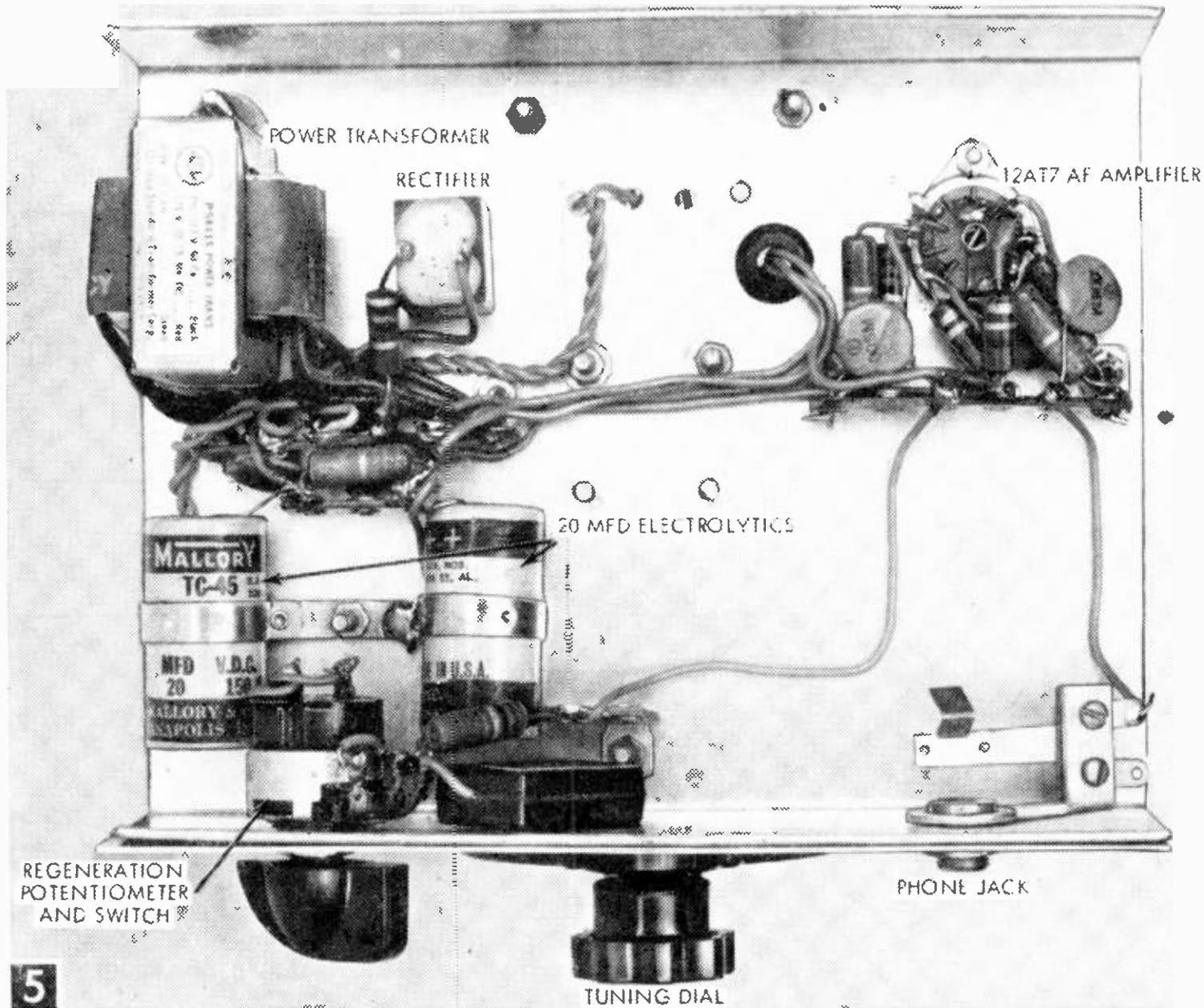
Now, wire the audio amplifier. Temporarily install the 'phone jack, and wire the output audio amplifier stage.
