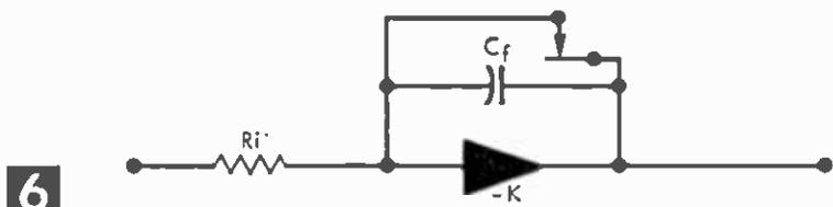
**6** When initial condition is zero, the integrator capacitor is shorted by a relay until computation begins.
