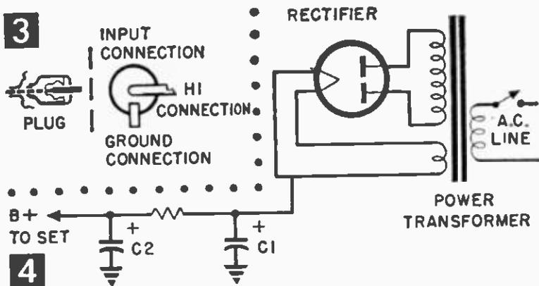
3. A broken shield or disconnection from plug ground or a faulty or open input jack can cause hum pickup.
