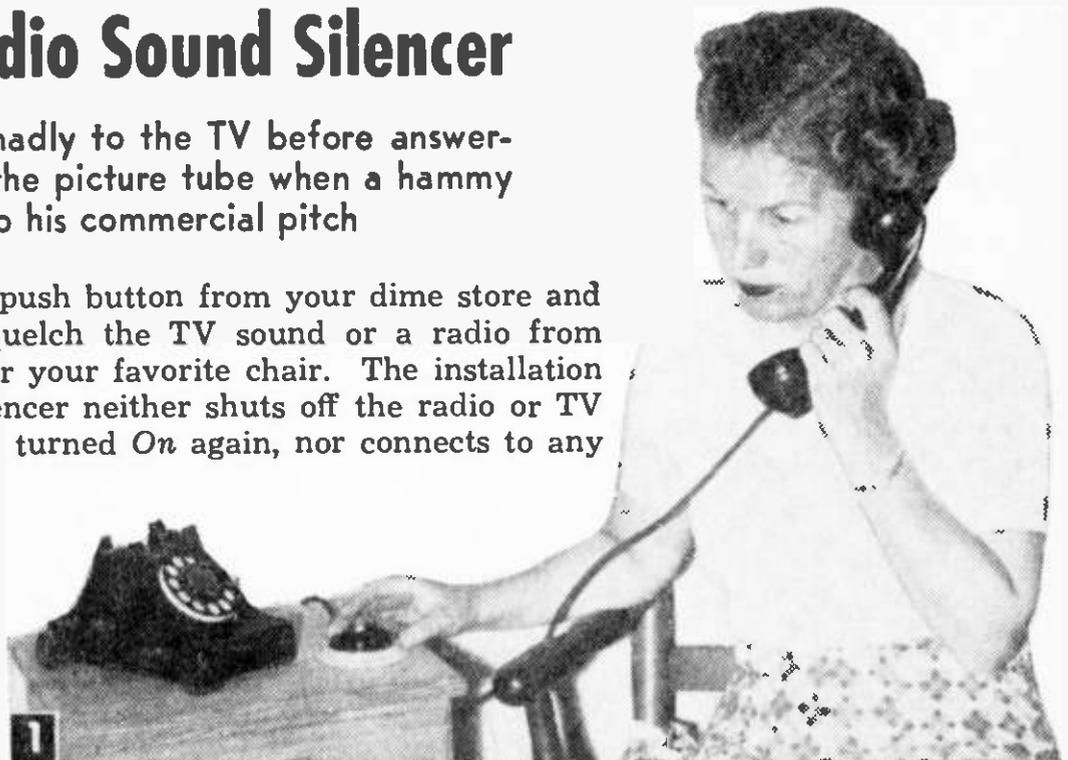
1 Silencer button by telephone eliminates conversation being drowned out by radio or TV set.
