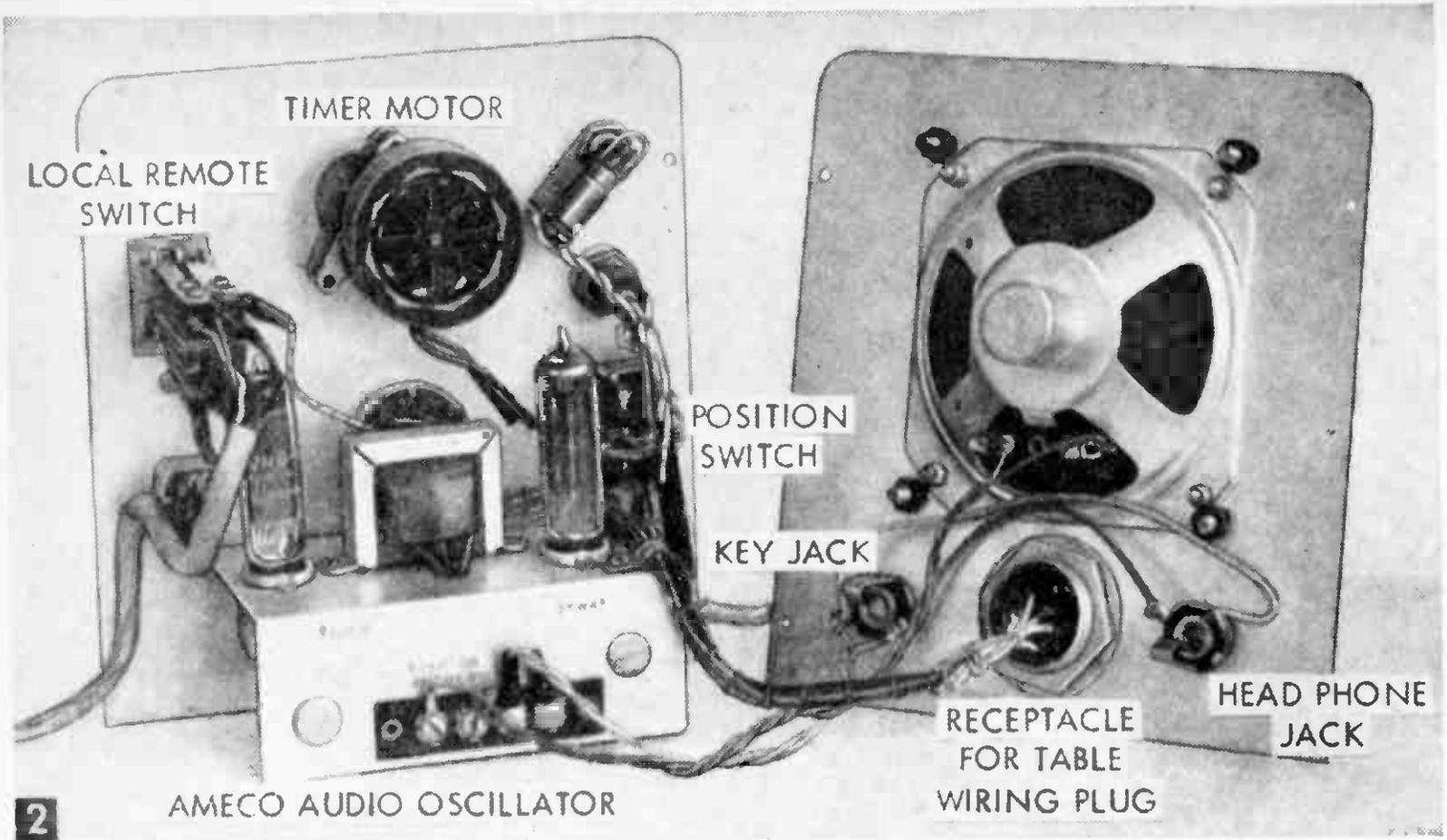
Parts layout and wiring of instructor's control panel
