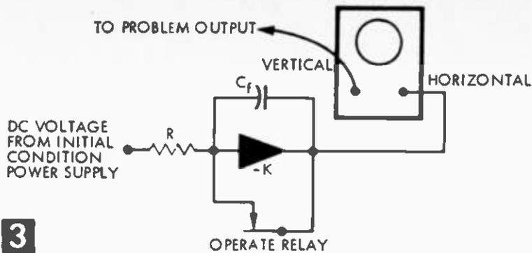
**3** An integrator can generate sweep voltage for CRO display.
