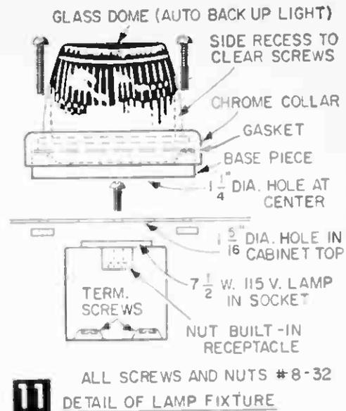
Finish top and edge of base to blend with unit or phone, after first masking bottom of recess to keep paint out. We used a ham-
