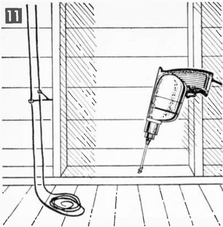
hole through the wall all the way. Insert the Wall-Thru fitting (Mosley Electronics, Inc.) mark it for length, and cut off the excess. A socket mounts directly to the fitting on the inside wall. Re-insert the wall-thru, run the wire through and trim as in Fig. 3. Connect the wires to the socket, and then mount the socket to plate of the wall-thru fitting. Connect to your outlet plug.
