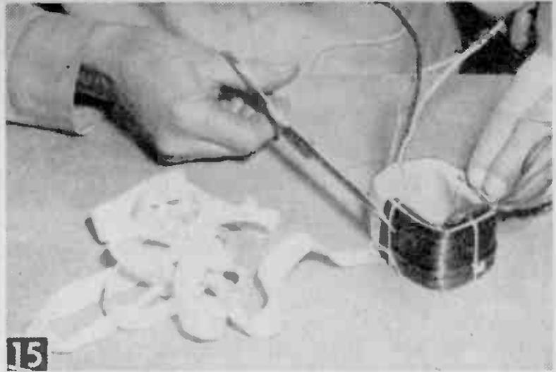
15 Pull each turn of the cotton coil tape tightly, and avoid bunching the tape at the corners.
