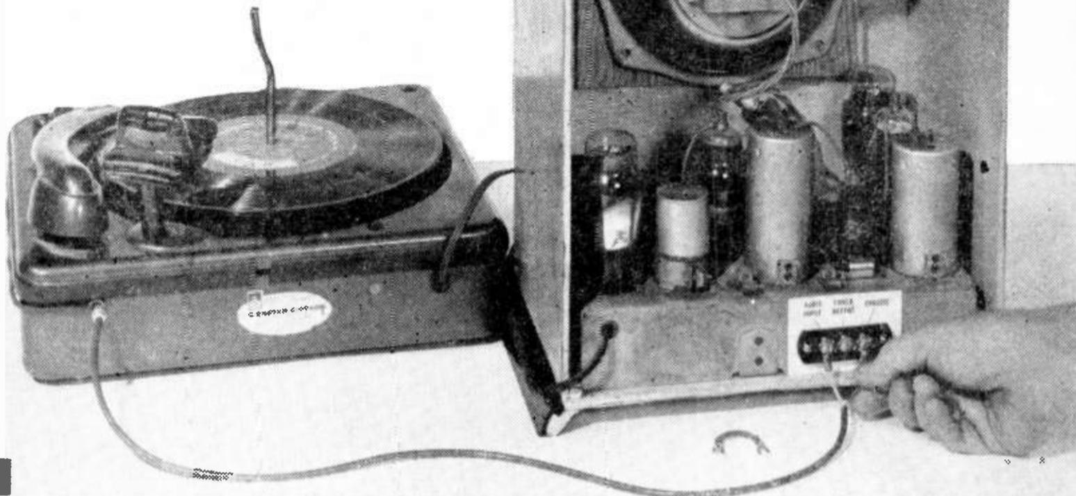
**How to modify your a-c radio for 20¢ to produce a crystal set amp, earphone radio, AM/FM tuner, record amp, or signal tracer**
