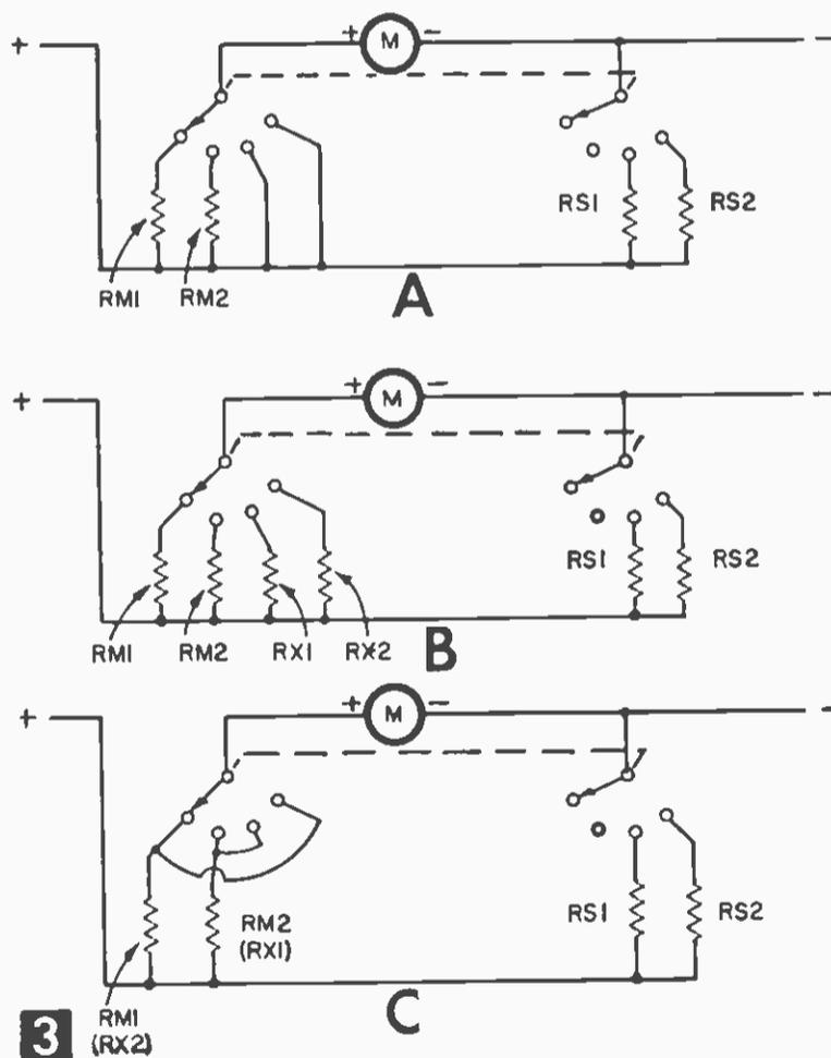
3 Means of switching various multipliers and shunts into meter circuits: (A) when only multipliers and shunts are used, (B) for extending the voltage rating by using special multipliers, and (C) for extending voltage by using the voltage multipliers themselves.
