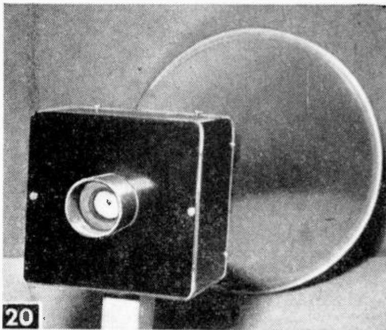
Mouthpiece with mike and its rubber ring inserted, mounted to Bakelite panel.
