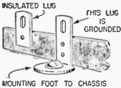
Terminal strips 55-C and 51-A have grounded lugs as shown above for connection of leads going to ground. If strips with all lugs insulated are used, simply use solder lugs under chassis screws for ground connections, as at AR-109 transformer feet.
