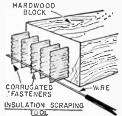
• This simple and long-lasting tool is practical for scraping and cleaning insulated wire to make firm solder connections. To make it, simply drive several corrugated fasteners into the end of a hardwood block.—G. E. HENDRICKSON.
