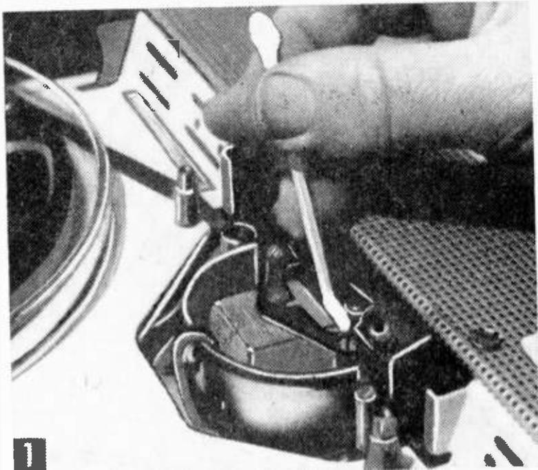
**1** Every so often, clean your recording head, rollers and pads with a cotton medical swab. Use alcohol or tape-head cleaner to dissolve deposits of tape oxide.
