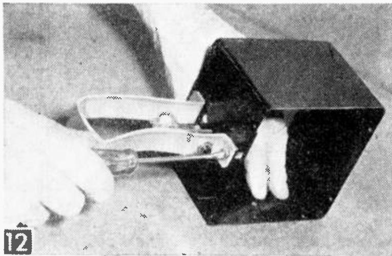
12 After fastening switch through its hole in handle with locknuts, attach handle frame to amplifier housing. Note that housing has been finished with primer, then black enamel lightly rubbed with steel wool.
