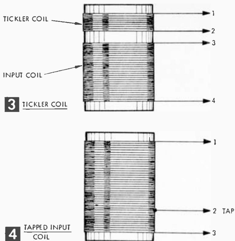
higher frequency circuitry of a receiver, since the bandwidth-limiting action makes its use in the audio section inadvisable. While most often employed in the detector circuit, regeneration often also improves the operation of if or rf amplifiers; here it increases both sensitivity and sharpness of tuning to a marked degree.
