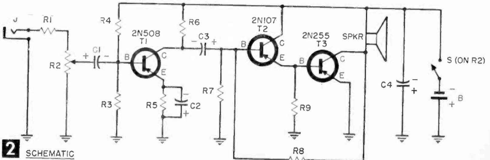
of the 2N255 from overloading the preamp. The driver output from the emitter of the 2N107 is directly coupled to the 2N255. R8 provides dc stabilization and a considerable amount of audio feedback.
