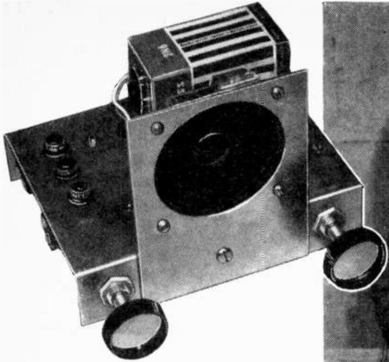
Here's a complete sound system that operates without a-c power. A built-in pre-amp permits use of dynamic mikes, reluctance type pickups as well as crystal phono pickups.
