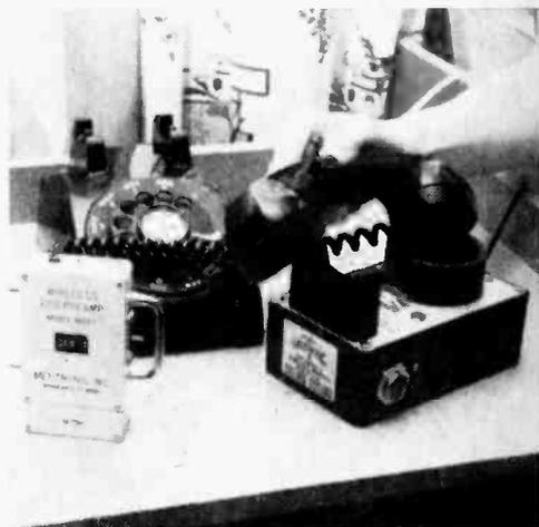
3: THE WIRELESS ECG preamp (left) picks up patient's heartbeat and transfers it to the monitoring equipment. Gadget on right converts the signal to an audio frequency and sends it into the phone mike.
