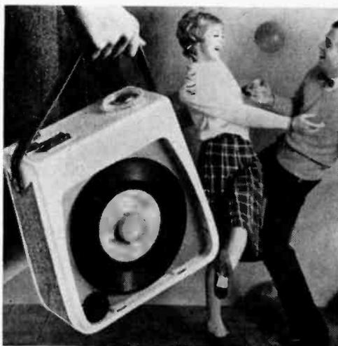
ture of permitting the record to be played while the unit is in any position, or even while it is being carried. The mechanism which accomplishes this trick includes a tone arm which plays from *underneath* the record (it contains a sapphire needle). Known as the "Swing Along," the unit is claimed to have what the manufacturer calls "remarkably big audio." The unit weighs 6 lbs., operates from four *D* batteries. Price: \$79.95. (Channel Master, Ellenville, N. Y.)
