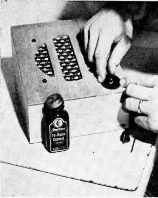
**IF Baffle Panel** is too thick, counterbore mounting hole and attach dial plate to L-Pad with radio cement or Duco.
