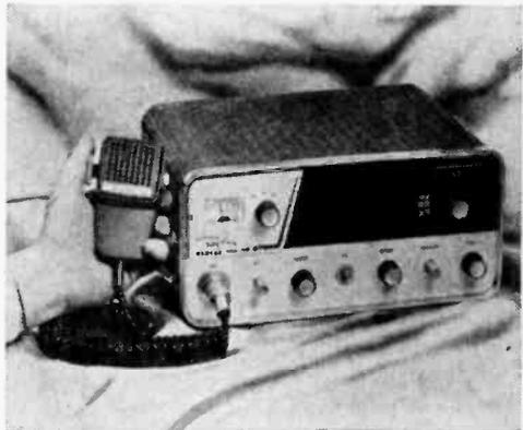
**Regency Range Gain** CB unit mentioned in text tunes in any of the 23 CB channels. Frequency synthesis provides crystal-control operation for the transmitter and receiver. A 3.5-kc. vernier control on the front panel can be used to zero in on those CB signals that are "off channel." Ready to operate, the unit sells for \$269.95.
