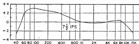
high frequency equalization at the 7½ ips speed set the equalization to maximum and very slowly adjust the bias current for flat playback response. While this adjustment may appear complex keep in mind that this is how professionals compensate for different tapes—you can pull this trick with few budget recorders.
