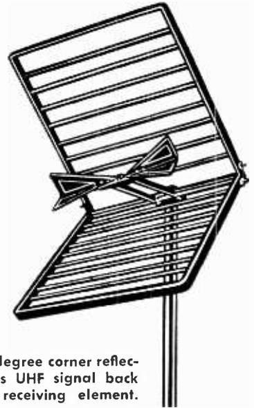
Fig. 5. 90-degree corner reflector bounces UHF signal back to dipole receiving element.
