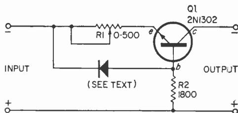
Schematic diagram for the Current Clamp shows output current passing through Q1's emitter-collector circuit. Graph at left shows current limiting for 1.5-volt input.
