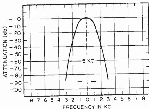
Fig. 2. Bandpass of mechanical filter is only 5 kc. wide at 60 db down. Note steep sides of curve block out side band pickup.
