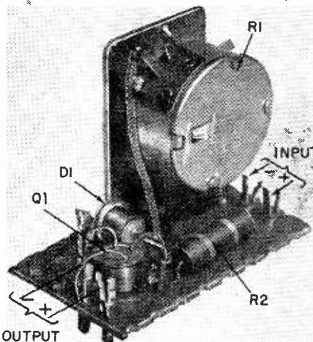
supply would *not* be correct for clamping at 25 ma. with a 30-volt supply. The variations can be minimized by running a fairly stiff current through the diode, on the order of 100 ma., but it has been found more convenient to run from 1 to 10 ma. through the diode and to simply live with the variations in setting of  $R_1$ .
