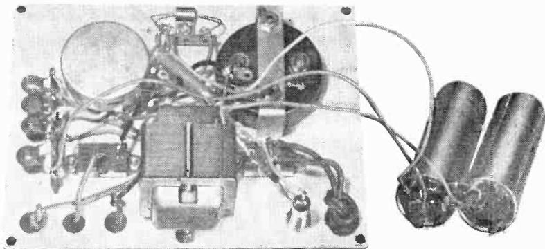
All the parts are assembled on an aluminum panel cut to size of plastic case.
