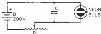
When the neon lamp is in the circuit, the supply voltage and the lamp characteristics have an effect on the period of the circuit. Suppose the neon lamp fires at 100 volts and extinguishes at 70 volts. If the supply potential ( $B$ ) is 200 volts,  $C$  will not charge to 63 per cent of the supply voltage (126 volts) because the neon lamp will fire when the
