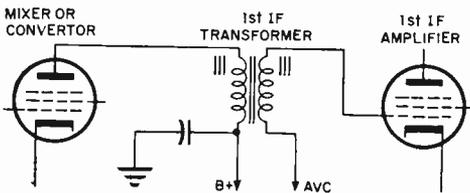
Fig. 4. Typical mixer or converter stage of a receiver showing 1st IF tunable transformer.
