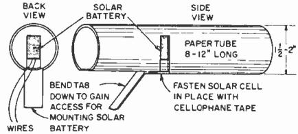
Paper tube from 8 to 12-inches long serves as shield for photo cell—conserves gain.
