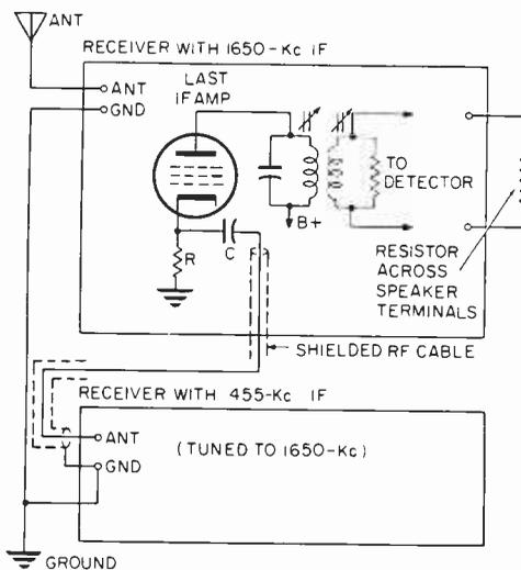
resistor should have the same value as the speaker impedance. Tune the second receiver to 1650-kc and tune in the stations with the first receiver. The audio volume control of the first receiver will have no
