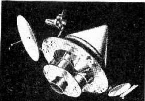
Avco's concept of a Mars Voyager spacecraft shown in transit (above). The vehicle is oriented to keep the solar panels facing the sun. The lander will be separated and sent on an impact course to Mars. Space bus will then orbit Mars sending back to earth TV and other data. Below, Mars lander is shown after impact. Folding panels have been opened to expose scientific instruments and to allow communications antenna to aim at earth for data transmission.
