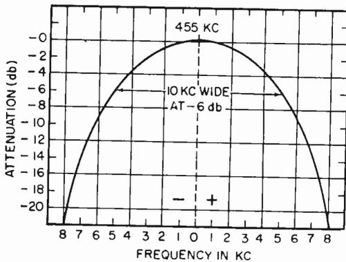
Fig. 1. In (A) above, graph shows bandpass of a simple stage of IF amplification permitting severe QRM by stations up to 5 kc. either side of center frequency. Even stations further out can cause trouble. In (B) below, tuned cascaded IF stages can give -60 db attenuation 10 kc. from center frequency—still not good for nit-picking DX AM-SW stations.
