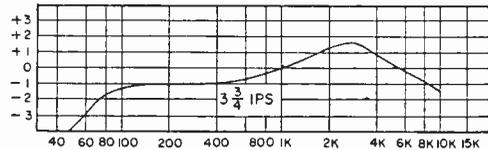
Typical response curves for the Knight-kit KP-70 record/playback stereo preamp are shown for both 7½ ips and 3¾ ips. Actual response curves for individual units will vary slightly and will also depend on particular tape, bias adjustment and high frequency boost adjustments. Always use quality tapes.
