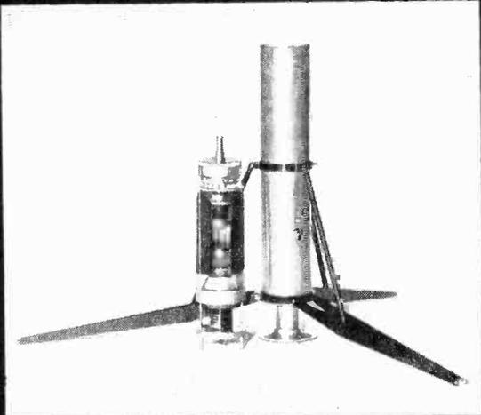
Multivibrator, a biological Mars probe, is designed to seek out basic carbon compounds of life. Left, unit and container; below, fluorescent light test chamber.
