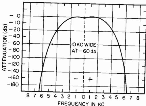
**The Mechanical Filter.** One of the best ways to achieve razor sharp selectivity is through the use of a mechanical filter. The filter consists of several sections made of nickel alloy resonators which pass virtually only the frequency to which they're tuned. Transformers at both ends couples the signal in and out.
