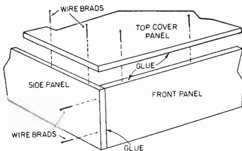
**Cabinet Detail Drawing #1—Cover for unit is glued—brads hold pieces while glue sets.**
