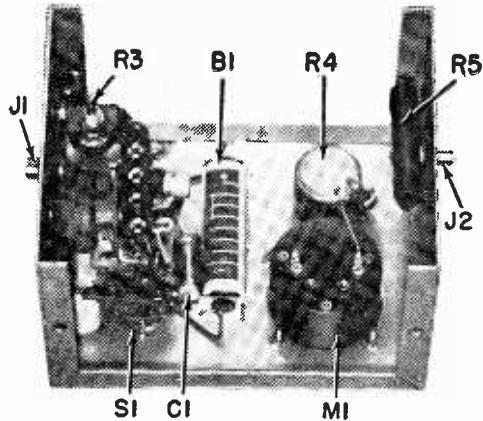
Inside view of the Tape Tester is uncluttered and easy to wire. Note that VU meter circuit is physically isolated from the oscillator.
