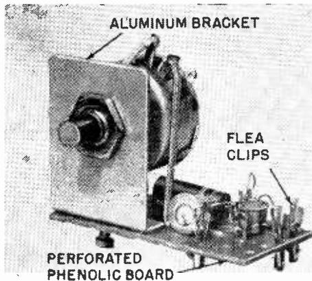
Front view (top photo) and rear view (bottom photo) of the Current Clamp showing location of parts and method of assembly. Entire unit can be installed in a plastic case.
