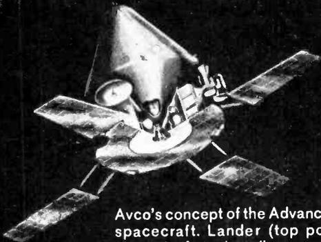
Inner sphere in Advanced Mariner lander contains scientific payload and communications, and is protected by impact crush-up case.
