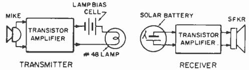
Block diagram for a simple light transmission system. No need for exotic lenses.
