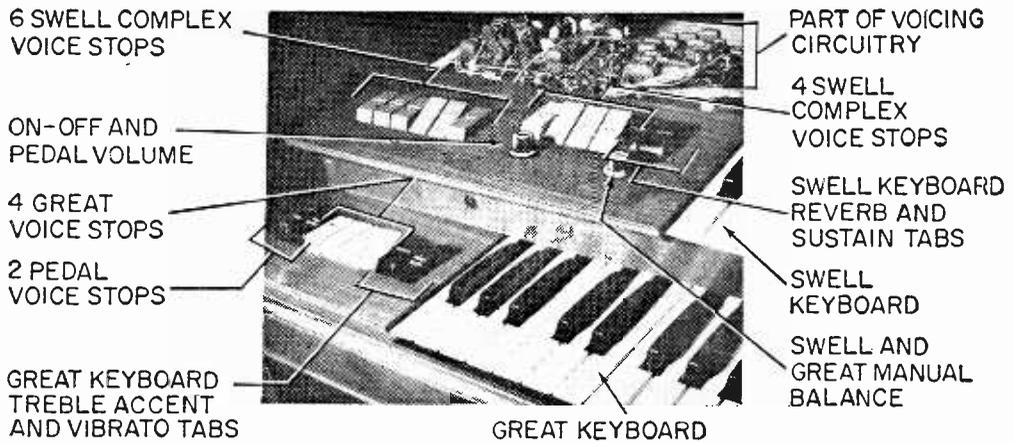
Fig. 9. Photo of left side of keyboards shows complex switching used to get voicing.
