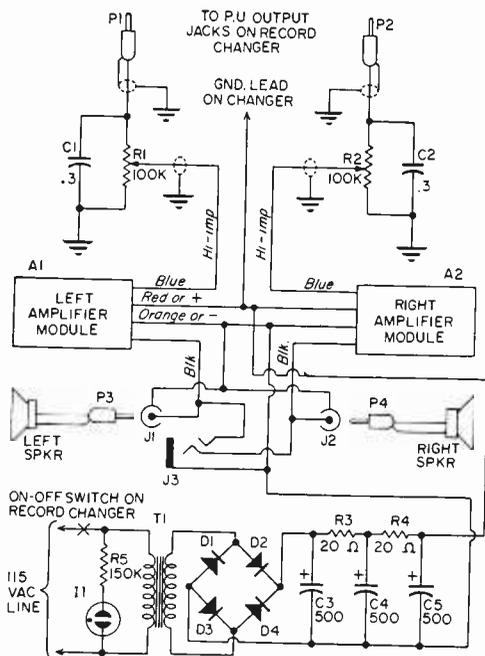
Schematic diagram for the Stereo Compact does not show amplifier details because these circuit sections are purchased modules. Note use of shielded cables on input circuits—dress these leads away from AC.
