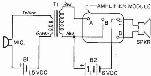
Schematic diagram does not show amplifier details—not necessary for moduled part.
