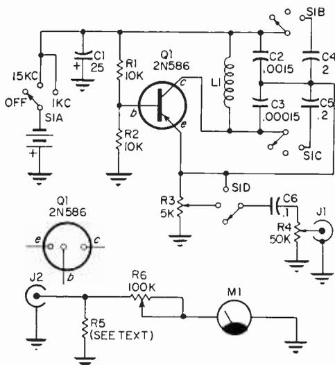
Schematic diagram for the Tape Tester—keep S1 set at off during playback of test tape.
