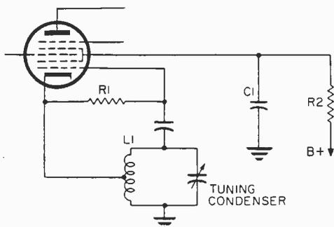
range. The trouble is usually due to a defective converter tube, change in the value of the oscillator grip leak (R1) or in the value of the screen voltage dropping resistor (R2). It could be that by-pass capacitor C1 may be leaky causing the screen voltage to drop. Try a new grid leak (R1) of the same value as the original. If that doesn't do it, change R2 and
