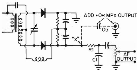
If your tuner does not have a multiplex jack, you will have to provide your own by tying into the FM tuner audio output circuit immediately before the de-emphasis network. How it is done schematically is shown above for the ratio detector and below for the discriminator detector. Actual detector circuits may vary from unit to unit, but R1-C1 network is always used to provide de-emphasis effect.
