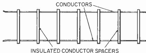
Fig. 9. Open-wire type TV lead-in is best when losses must be minimized. Spacers between conductors are made of porcelain glass.
