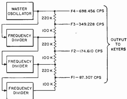
Fig. 6. Master-oscillator/triple-divider circuitry used in Heathkit/Thomas organ.
