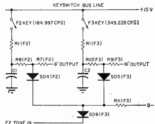
**Fig. 8.** Simplified schematic showing the diode switching used in the Heathkit organ.
