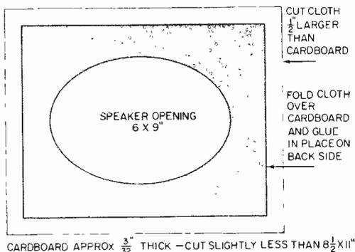
**Speaker Grille Detail Drawing—Using materials found at home can reduce cost to zero.**
