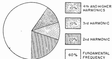
Fig. 2. Breakdown of the fundamental frequency and harmonics in a violin's sound.
