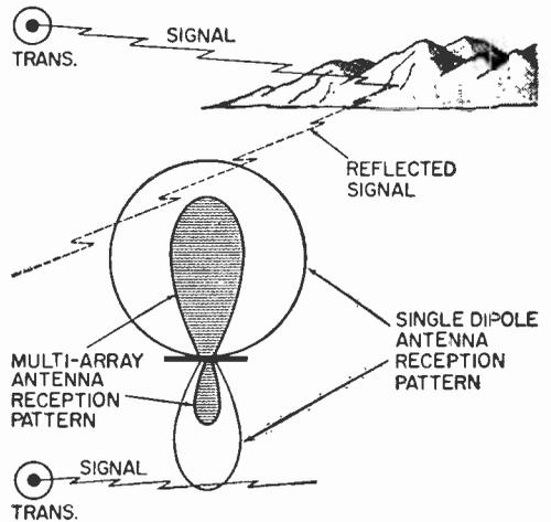
Fig. 6. Multi-array UHF antennas can eliminate ghosts caused by multi-reflections.
