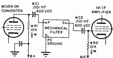
Fig. 5. Circuit modification for mechanical filter—\* indicates added circuit components.
