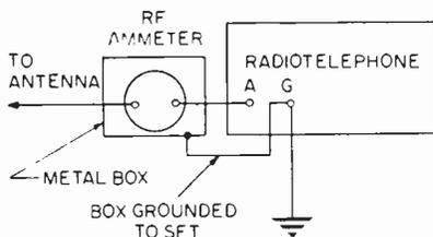
the antenna lead-in and the antenna binding post. Then tune the transmitter for maximum antenna current on 2182 kc, the most important channel. If the transmitter is designed so that it can be tuned for optimum performance on each channel, follow the procedures in the rig's instruction book. Some sets, like the Hartman, have a front panel antenna tuner with which the set can be adjusted for best performance after selecting a channel.
