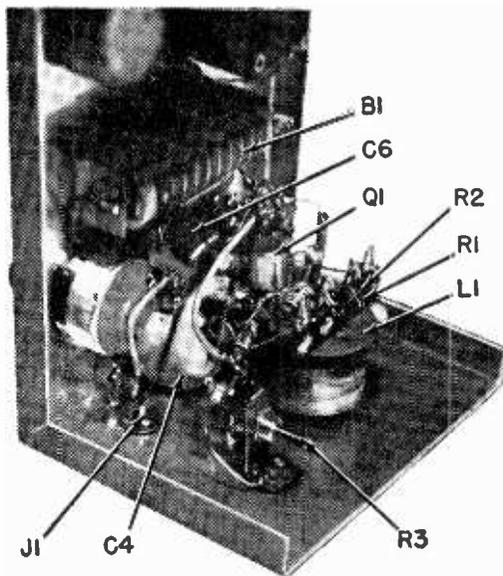
R3 is mounted to the cabinet with an L bracket made from straightened cable clamp.
