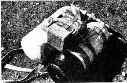
Six-volt battery pack is strapped to diver's air tanks (top photo). Aqua-Com is attached to diver's belt except in bottom photo where it can be strapped to tanks.
