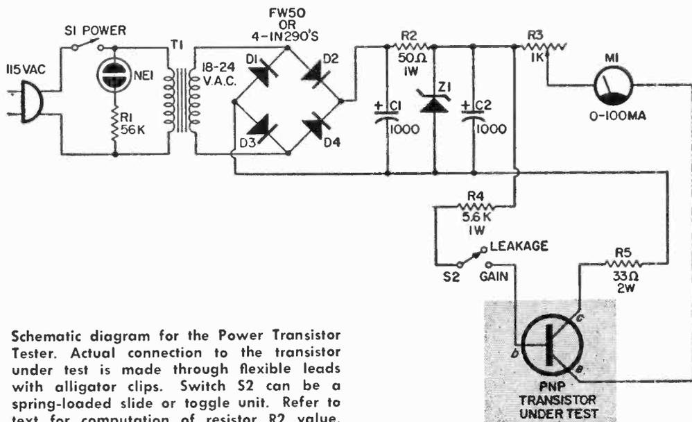
Schematic diagram for the Power Transistor Tester. Actual connection to the transistor under test is made through flexible leads with alligator clips. Switch S2 can be a spring-loaded slide or toggle unit. Refer to text for computation of resistor R2 value.
