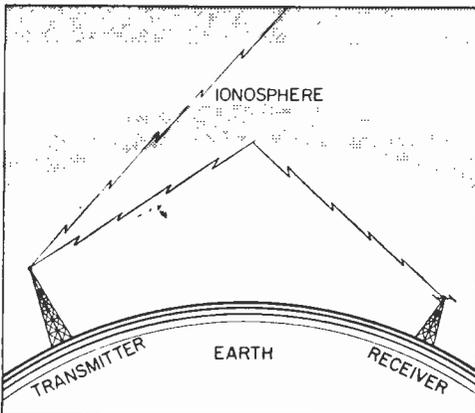
Fig. 1. VHF signals skip to distant receivers—UHF signals pass through ionosphere.
