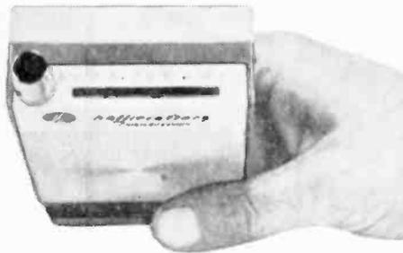
Top of the CB-15 reveals the AM tuning dial. The whip antenna for CB communications telescopes out of the case. Neat packaging of the receiver/walkie-talkie is shown at the right. CB crystals plug in for receive and transmit; AM antenna is built in; and battery holder is spring loaded.
