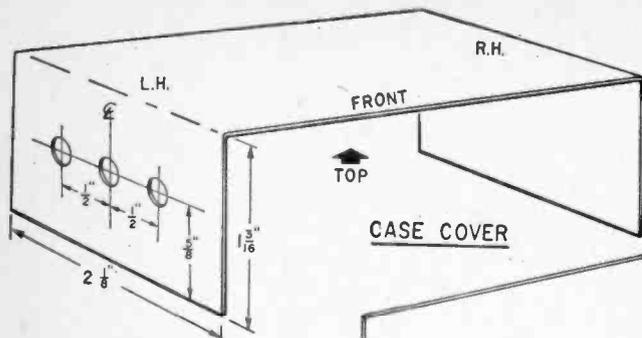
Layout of chassis box is not critical. Holes in case cover can be either on right or on left. Placement of front-panel controls is also subject to a change in spacing and position.
