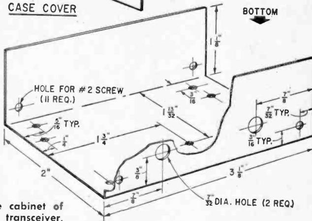
Compressor was installed inside cabinet of this Lafayette HA-650 6-meter transceiver.
