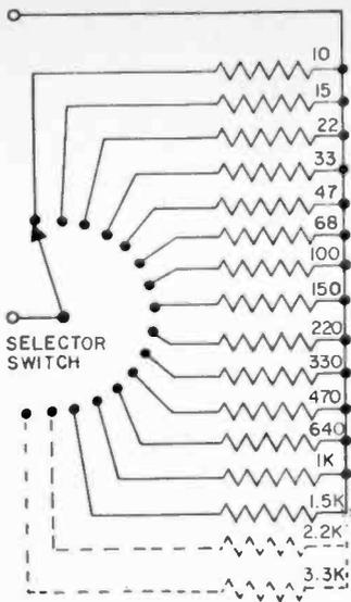
tolerance nearest the indicated resistance reading and readjust the variable decade to the standard value you intend using and make certain the circuit still functions properly, if not perhaps a closer tolerance resistor must be used.
