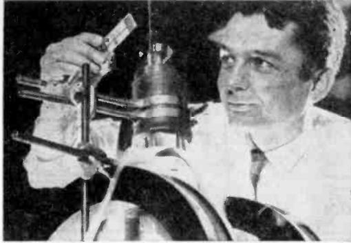
■ Working with extremely thin films of tin deposited on a glass slide, a General Electric scientist has built and operated a laboratory model of a direct current (DC) transformer—long considered an “unachievable” scientific goal. The device is a result of research on superconducting materials—metals and alloys that have zero electrical resistance and unique magnetic properties at very low temperatures of liquid helium.
