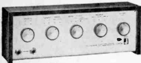
Five controls are spaced across the CC-1's front panel. From left to right: Speakers (On-Off); Channel/Stereo (left, right, reverse, normal); Mono/Stereo (mono, regular, space perspective); Balance (increase left, normal, increase right); and Volume control. See text for operation of space perspective.
