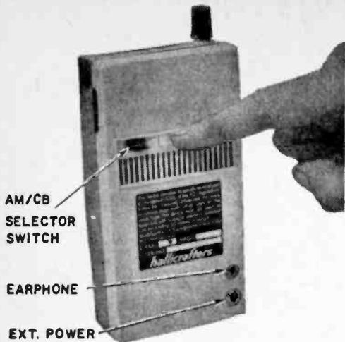
Small slide switch on the back of the case selects CB or AM operation. Jack is provided for earphone which comes with CB-15.
