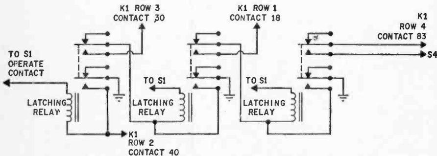
This alternate latching-relay circuit can be carried out still further by adding even more relays. Complex contact combinations can be made with just a little time for experimenting.
