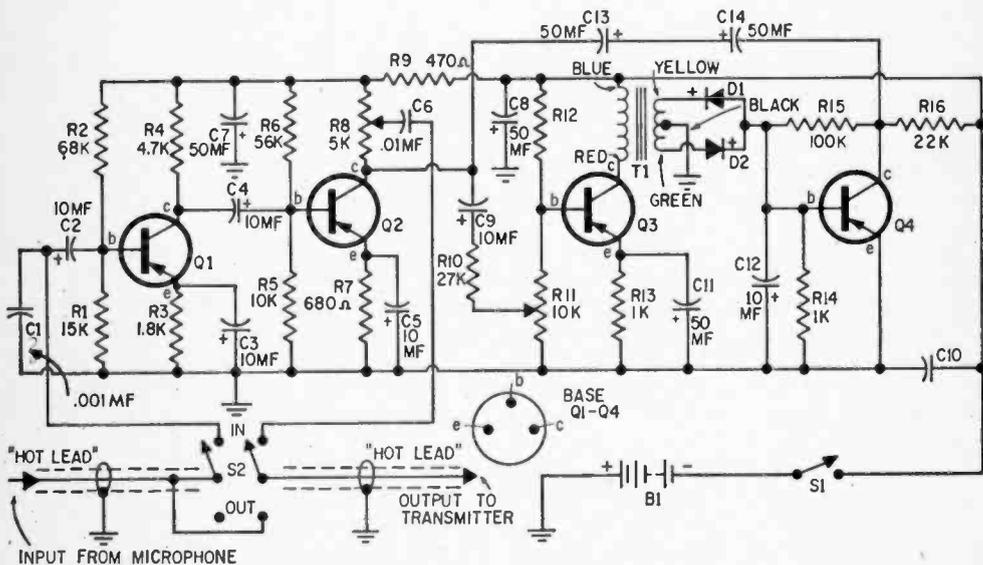
Switch S2 can be eliminated if you want the Compressor to be in the circuit at all times.
