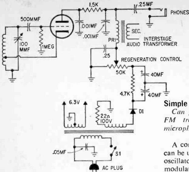
plugged in and connected to a ground. Reverse the AC plug prongs so the lamp does not light. Keep the regeneration control so that the circuit won't oscillate and cause interference. The set will be most sensitive just below the point where oscillation begins.
