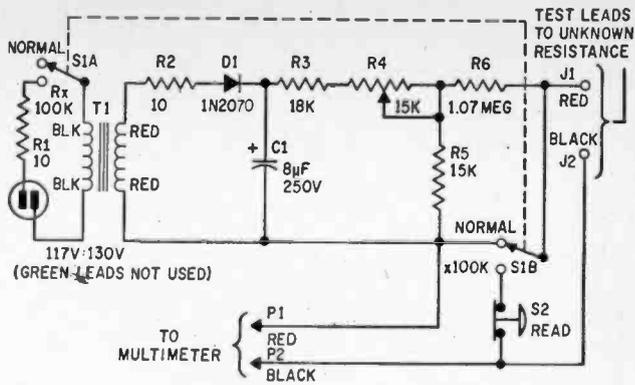
For portable use transformer, rectifier and filter can be replaced with 67½-volt battery. Rewire S1A into battery circuit to prevent continuous current drain in normal position.
