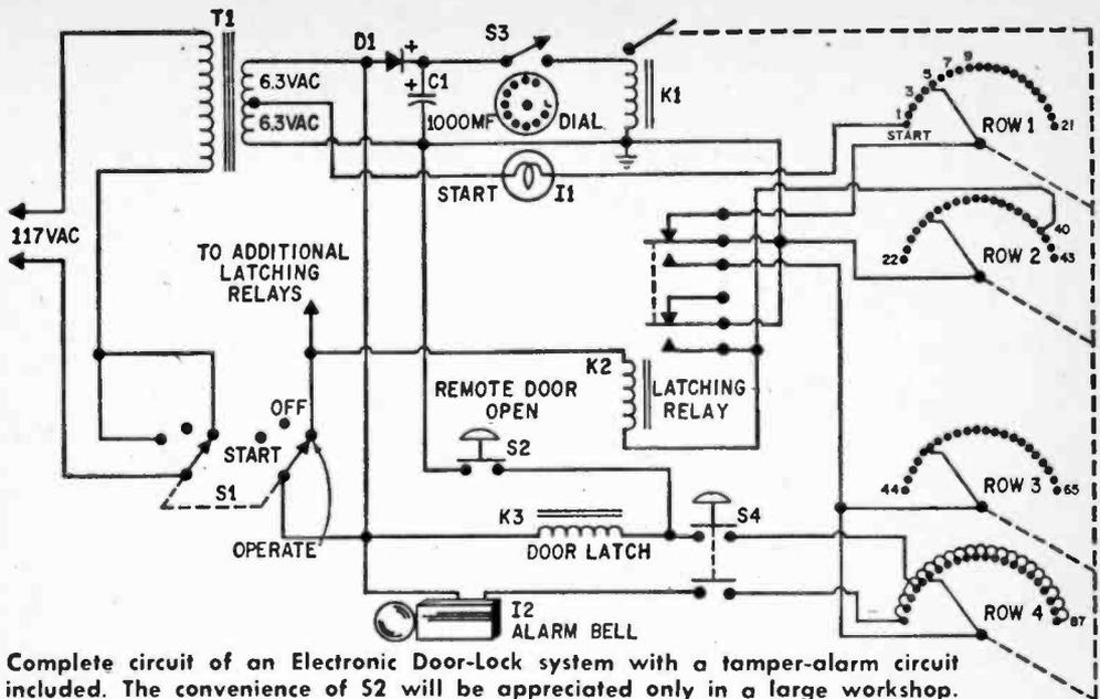
Complete circuit of an Electronic Door-Lock system with a tamper-alarm circuit included. The convenience of S2 will be appreciated only in a large workshop.
