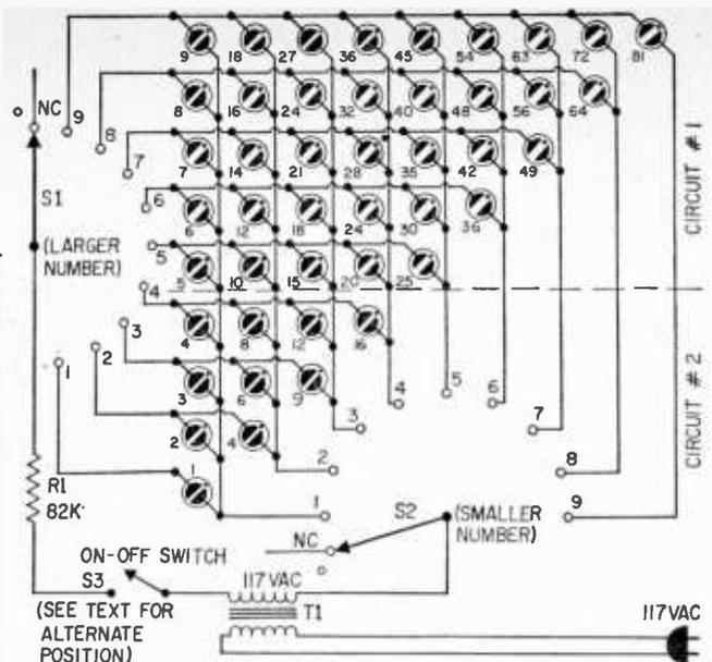
**Wiring of Calculator** is quite simple. The ten lamps of Circuit #2 are physically fitted into the vacant triangle in the lower-right corner of Circuit #1. S3 can be replaced with a pushbutton or eliminated since the NC positions of S1 and S2 have the same effect. For a much brighter display use 6-volt pilot lamps—replace T1 with 6.3-volt filament transformer and eliminate R1. S3 should be a momentary contact pushbutton to give long life to pilot lamps.
