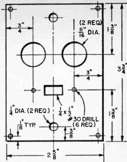
Complete circuit is mounted on this cover using lamp and switch lugs as tie points.
