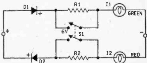
Circuit is simple. R1, R2 limit current through 6-volt lamps when used on 12-volts.
