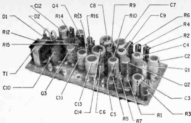
Mounted vertically the components resemble the skyline of a large city. This technique allows more components to be packed into each square inch of perforated board. Wafer-thin C1 is mounted against underside of board.
