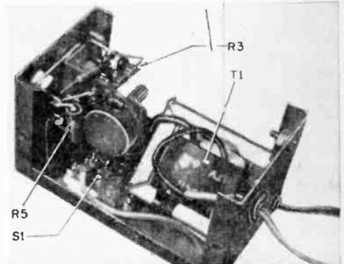
to *Normal*. Adjust the multimeter *Ohms-Adjust* knob for a reading of zero ohms. Set the Expander to *X100K*. With a screwdriver, set R4 so that the multimeter again reads zero ohms (this adjusts the voltage to 67.5 volts and shouldn't have to be touched again unless the line voltage changes). Plug the meter leads into the Expander, connect a resistor, press the *Read* button, and read. ■
