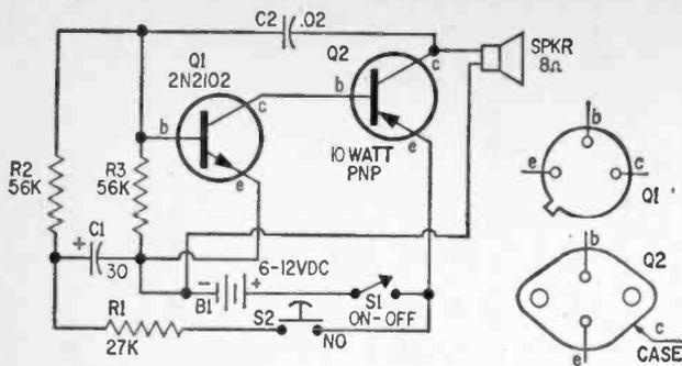
Capacitor C2 provides the necessary feedback to bring the audio amplifier circuit into oscillation. Try different values for C2 (see text) to alter the Screamer's output pitch.
