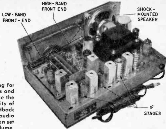
Shock-mounting for dual front-ends and speaker reduce the possibility of mechanical feedback causing the audio to howl when set for high volume.
