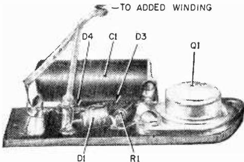
Dry-cell eliminator is about same length as two power transformers. Its thickness is about that of penlight cell and can be fitted into most metal-cased VTVMs.
