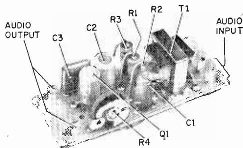
This is just about the most compact layout possible. Transformer T1 is the largest component perforated board. Resistors and capacitors could be wired flat instead.
