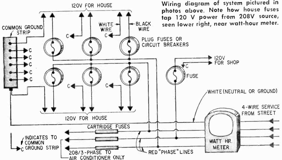
Wiring diagram of system pictured in photos above. Note how house fuses tap 120 V power from 208V source, seen lower right, near watt-hour meter.
