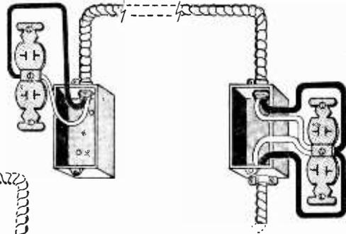
Machine screw tightens clamp to hold BX cable in Gem box—BX connectors are needed for square and round boxes that are used with BX or conduit (pipe) since these do not have built-in clamps of any sort.
