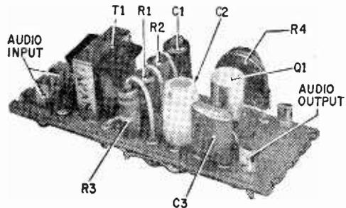
Completed perforated board showing components in place; note spaghetti on the leads.
