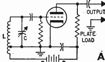
Fig. 3. In vacuum-tube oscillator (above) feedback is through induction by cathode current through bottom turns of inductor  $L$ . Common-base transistor circuit (below) has separate windings for emitter, collector circuits wound on same transformer core.
