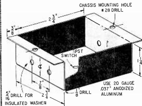
The adapter circuit may be built into a commercially available "Minibox" or you can construct your own aluminum enclosure, using the dimensions given here and instructions given in text.
