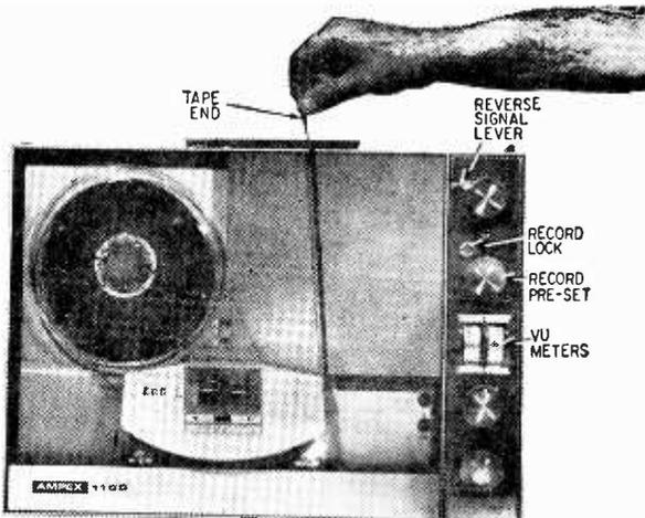
To thread the 1100, pass tape against heads and into slot. Motor starts; tape threads.
