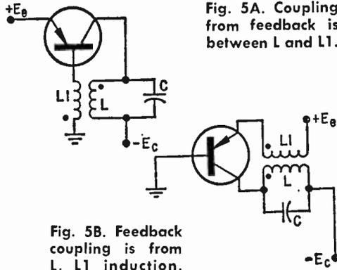
Fig. 5A. Coupling from feedback is between  $L$  and  $L1$ .
