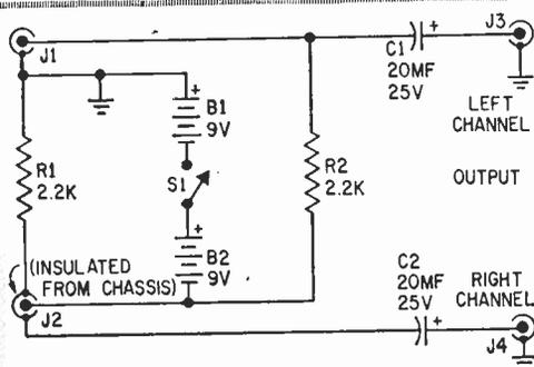
**Fig. 1.** Follow this schematic if you want the better circuit, which includes a phase inverter. Since it reverses the phase of one output signal, final set-up of speakers is somewhat simpler. Note that J2 must be insulated.
