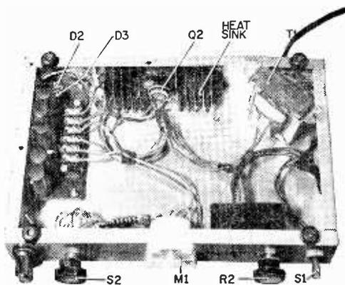
Here the inside of DC supply is seen from bottom. There's no crowding of components. Make good solid connections for all wiring that carries current from T1 to the output.
