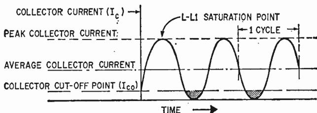
Fig. 4. Graph of the collector-current flow in circuit of Fig. 3.
