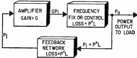
Fig. 2. The block diagram above shows one configuration of an oscillator. Feedback and frequency-control networks may be in either the input or output of the amplifier.
