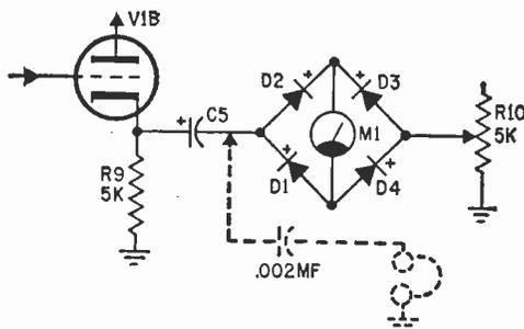
A single earphone, or a set of high-impedance headphones, can be permanently connected to C5 through a small capacitance without upsetting the calibration of the meter.
