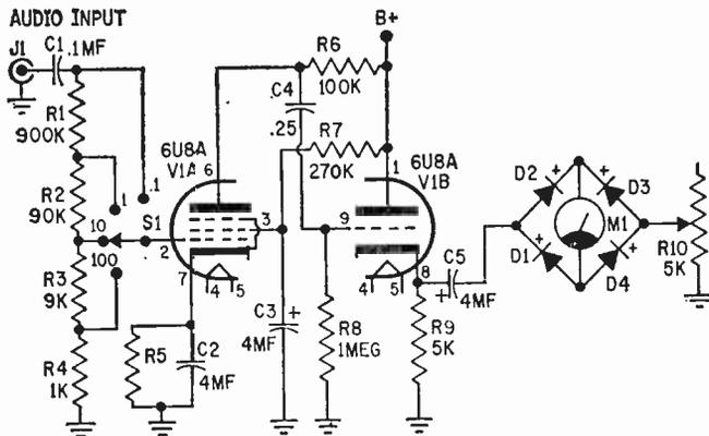
Voltmeter-section circuit (right) is a 2-stage amplifier with bridge-type meter rectifier across output. Watch polarity of C5, diodes and meter.
