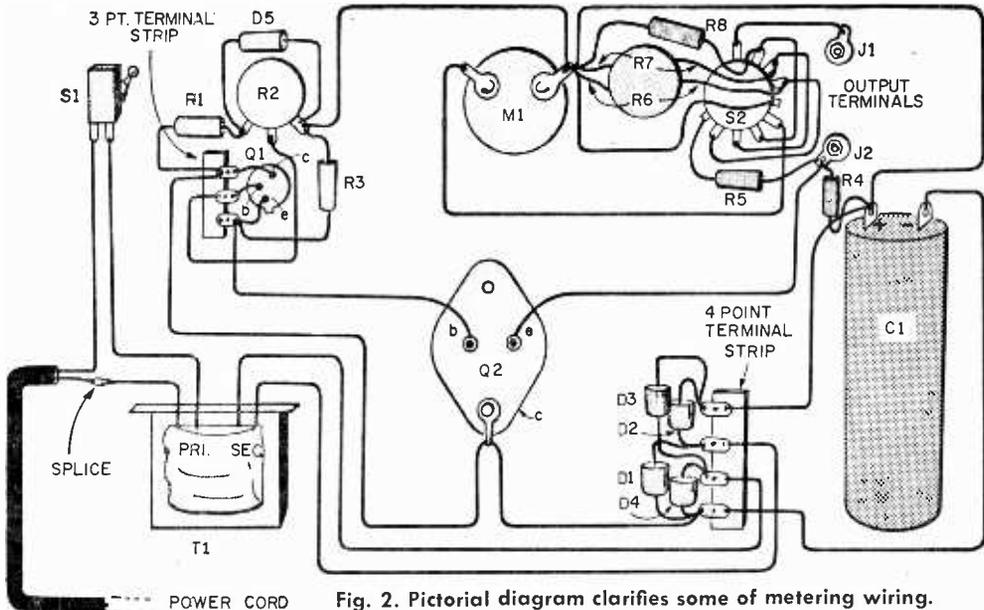
Fig. 2. Pictorial diagram clarifies some of metering wiring.
