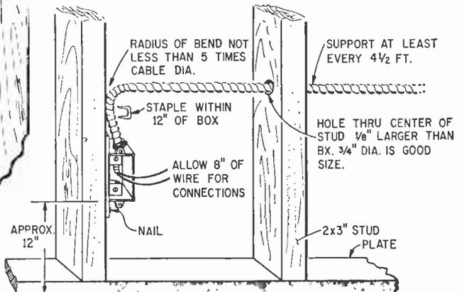
How you Add-A-Outlet depends on location of existing wiring and outlet boxes. The connections are simple. Running the cable through finished walls and ceilings can be a big problem.
