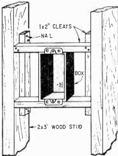
Cleats of 1 x 2-inch furring strip substitute for manufactured brackets, that are spot-welded at factory or attached with machine screws, to side or back of electrical boxes.
