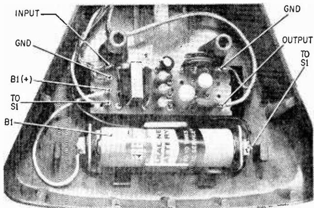
All desk-stand microphones do not have as much space in the base as this Electro-Voice. A change in the perforated-board layout may be necessary to fit components in space.
