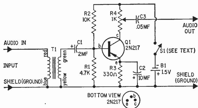
Circuit of Booster is simple and should present few problems even as a first project. If there is too much gain in amplifier C2 can be removed.
