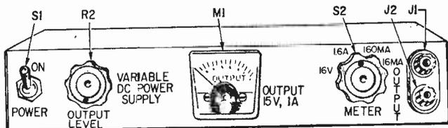
Front panel is actually side of a 2-inch deep metal chassis which is used as the cabinet.
