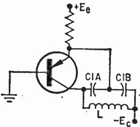
Fig. 5C is basically the same as Fig. 5A except that the tank (LC) circuit is AC-coupled (shunt-fed) to the collector with a capacitor. The current in Fig. 5D can be compared to that in 5B. The autotransformer action of the tank circuit is used as the feedback circuit with capacitor C1 used to block DC between the collector and the emitter. Fig. 5E is similar to 5A and 5D except series capacitors are used, in place of a tapped inductor, to provide the feedback path.
