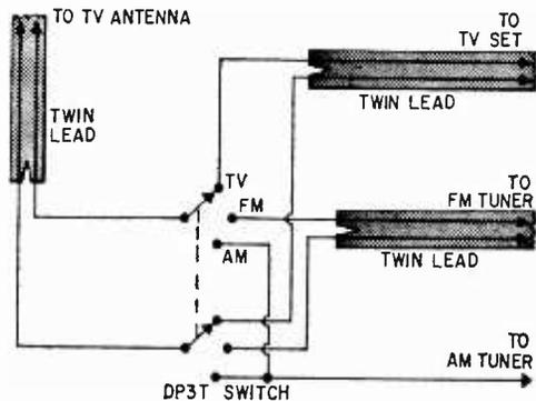
ly-polarized directional antenna as normally intended. For AM, the antenna assembly and the twin-lead form a capacitance-top, vertical antenna.
