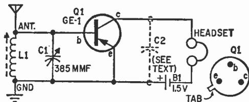
Even parts are not critical. C1 and L1 can be salvaged from any broadcast-band receiver. Q1: any general purpose unit.
