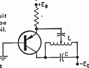
Fig. 5E. Colpitts circuit has series capacitors in LC.
