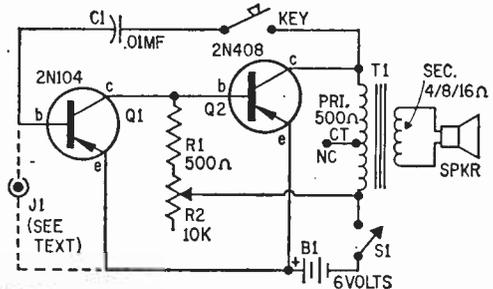
Fig. 6. Code-practice oscillator has standard parts. R2 controls volume. With key open, J1 can be used as an input to amplifier circuit.
