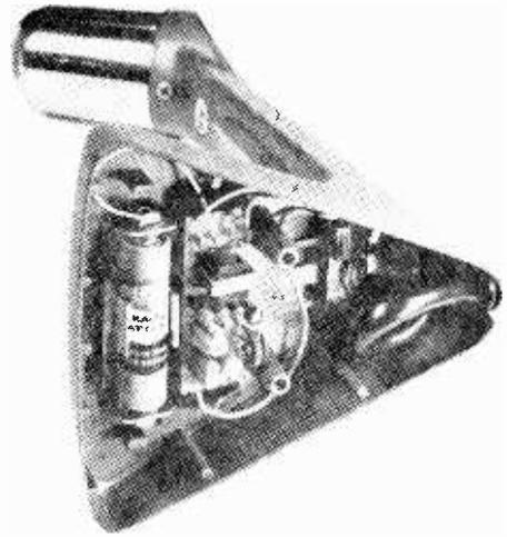
Booster, complete with dry cell, fits into base of this desk-stand microphone. Make sure you have room to accept dry cell and circuit board—just change layout to fit.
