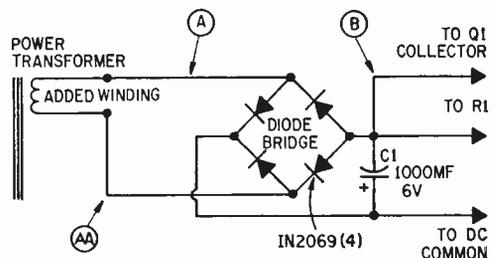
Fig. 4. Bridge rectifier circuit doubles ripple frequency and improves filtering.
