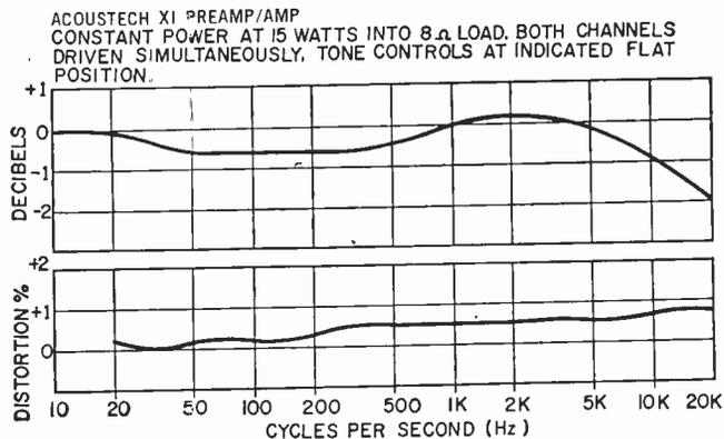
Fig. 2. With the preamp module added, the Acoustech XI becomes a first rate integrated amplifier. Curves prove that the unit can stand up against any other product on the market today. Bottom curve is for total harmonic distortion—IM distortion was buried in test-instrument noise level and cannot be measured because it is low.
