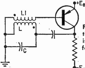
Fig. 5C. The DC through L and L1 is kept to just a few microamperes.
