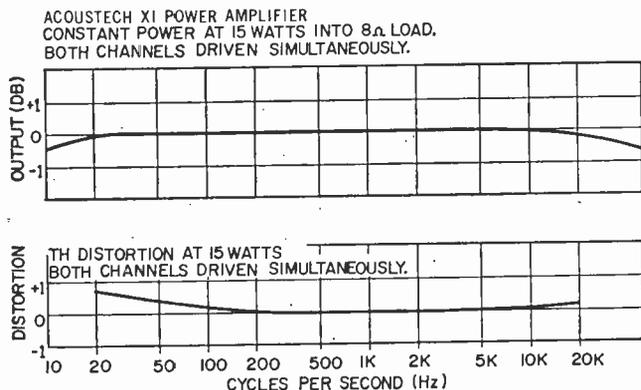
Fig. 1. You will have to squint to see the fraction of a db the constant-power curve drops at 20 Hz and at 20,000 Hz—the drop is less than .2 db. Percent total harmonic distortion never exceeded .7 db (at 20 Hz) and averaged about .25 db throughout the listening range. To make the tests valid, both channels were driven at full 15 watts out.
