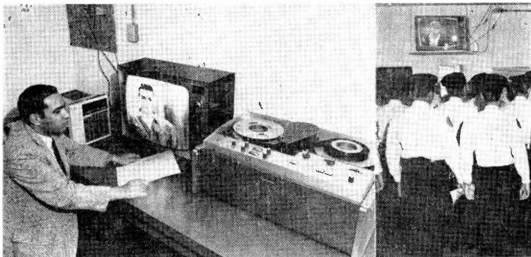
Ampex video tape system is used in experimental setup by Miami Police Department. Detective here is watching pre-recorded interview.
