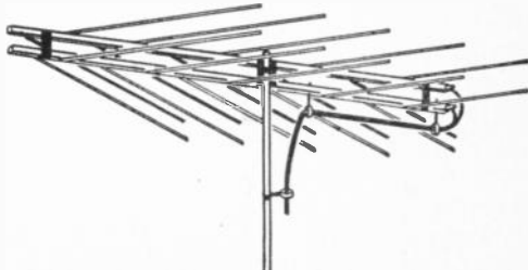
Basic log-periodic design is modified for color-TV and gives appearance of an entirely different type.
