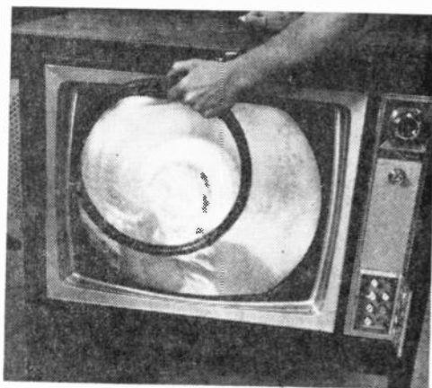
Fig. 4. Degaussing rids picture tube and other parts of stray magnetism that affects color.
