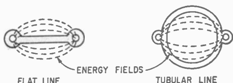
Fig. 25. Tubular line (right) keeps dust, soot deposits and water film (from rain, dew) out of field.
