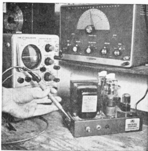
Fig. 6. Heathkit Model 1G-82 Sine-Square Generator and Tektronix 317 Oscilloscope being used to check output of CH-2133 Standard Transformer amplifier.
