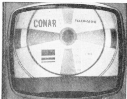
Fig. 19. Vertical centering control misadjusted. Yoke adjustments can often pull into line.
