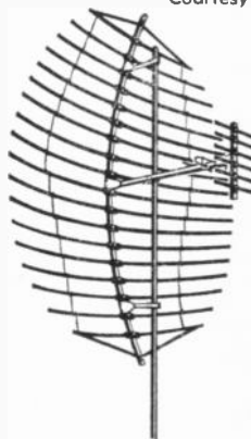
Double reflection, from parabola to flat reflector, assures maximum pick up area to catch UHF signals.
