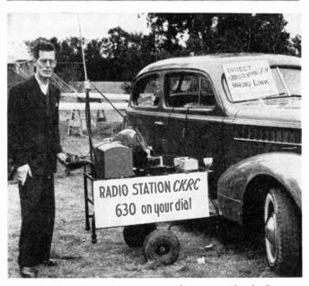
The FM radio equipment used to provide CKRC's listeners with an on-the-spot account of the Canadian Open Golf Tournament.
