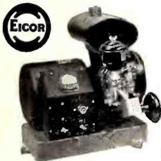
Here's plenty of power with matchless Eicor dependability. Operates at 1800 R.P.M., rated at 450 Watts A.C.—500 Watts D.C. All standard voltages. Push button starting. Available with remote control. 17" high, 15" wide, 17" long. Easily portable. Other Eicor Electric Plants in a complete range of sizes.
