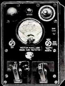
**Model 669 Vacuum Tube Voltmeter and Signal Detector** . . . Hear as well as measure the signal with this inexpensive instrument. Measures gain in video and sound amplifying channels—peak voltages in thyatron generators in oscillator circuits—grid potentials on cathode ray tubes—and other essential measurements in sound receivers.
