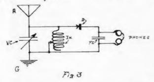
nection of aerial, ground and telephone cord, respectively. The crystal detector is represented by the letter "D" and may be made up of a brass cup to hold the mineral which a post just opposite from which projects a spring strip of metal having a fine Connect post "A" to the cup of the Detector "D." From the other terminal run a wire to the quter binding post "T." Connect one free end of the inductance to the cup of the Detector. Then run a wire from post (Continued on page 31)
