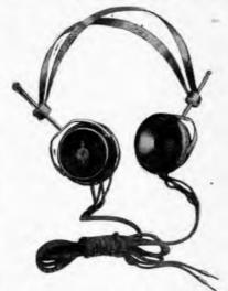
has resulted in the Manhattan Company placing upon the market receivers of their own product. The headband is designed for sanitation, being made of flat spring steel, rubber japanned with no covering. The sliding friction grip method of adjustment is employed. The case proper is flush on the back and the cord tips are concealed within the case. It is made in two types, 2000 and 3000 ohms.
