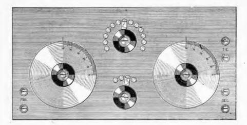
might be well to clear up a question that seems to lurk unspoken in the minds of many experimenters-a sort of skeleton in the closet question, ignorance of which no one wants to admit. "What does the secondary variometer do? How can it tune the circuit to a given wave-length, when there is no capacity in the circuit?" Yet the variometer does tune, and very sharply.
