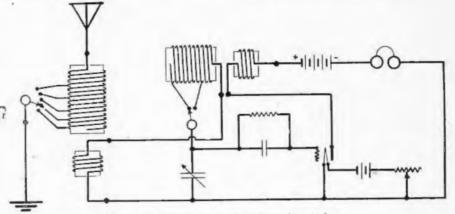
Fig. 3. Connections for the regenerative receiver
