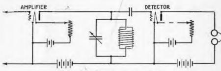
Fig. 1. A simplified circuit of the amplifier
